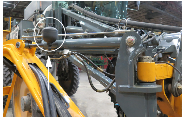
Accumulator (2) -Typical View
