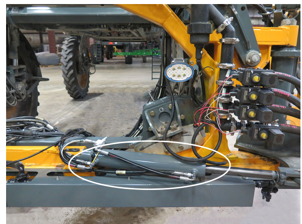
Main Fold/Breakaway Cylinder -Typical View
