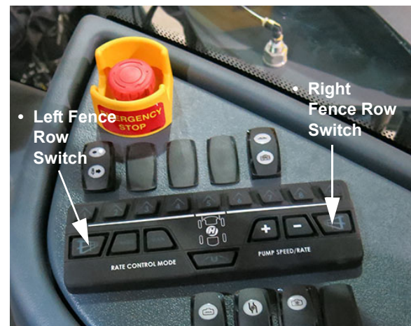
Fence Row Switches - Left and Right (Located on the side console) -Typical View
