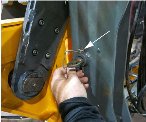
Lock Pin (Located on the outer side of transom frame) -Typical View
