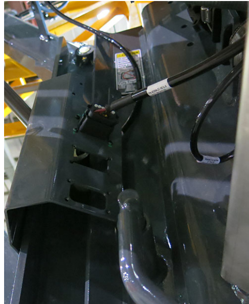
NORAC Connection (Located on the front right-hand side of machine) -Typical View
