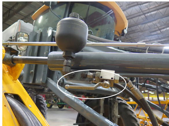
Level Cylinder Lock Valves (2) (Located near the level cylinder on each side of transom) -Typical View
