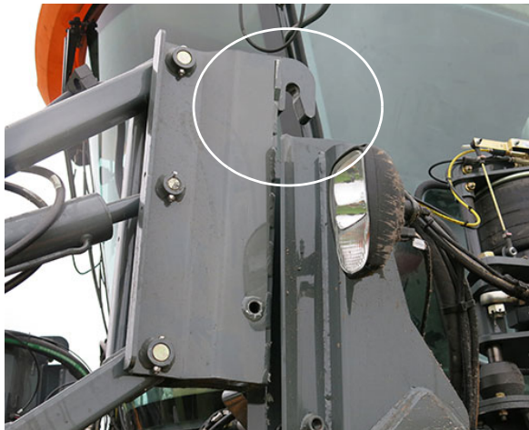
Attachment Clearing Mounting Pin -Typical View
