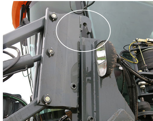
Attachment Clearing Mounting Pin -Typical View
