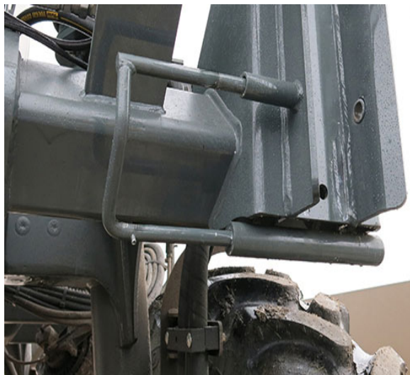
Lock Pin (2) (Located on the front left and right-hand side of machine) -Typical View
