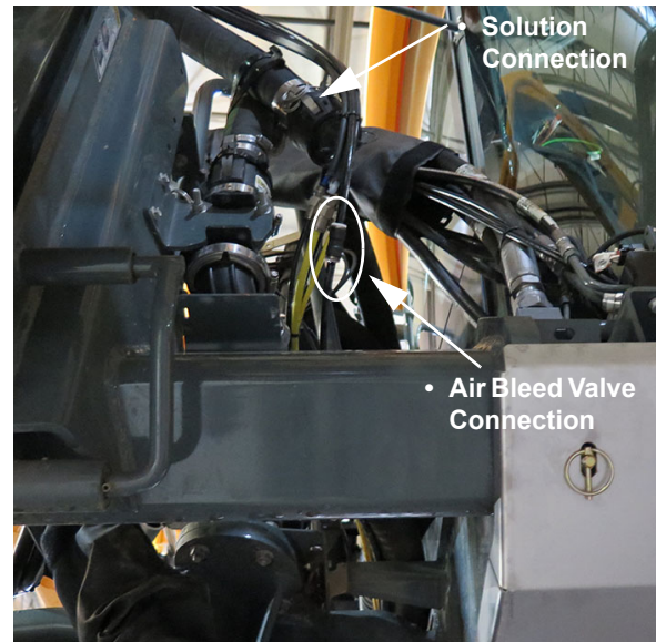
Solution and Air Bleed Valve Connections - Standard (Located on the front right-hand side of machine) -Typical View
