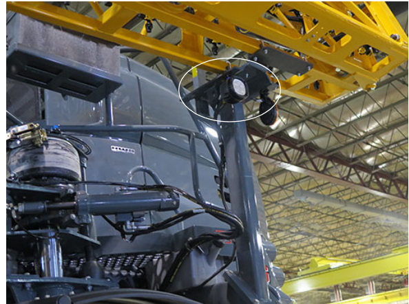
Work Lights (2) (Located on each boom cradle) -Typical View
