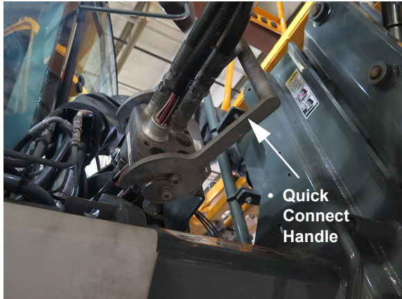
Hydraulic/Electric Multi-Coupler Assembly - if equipped (Located on the front left-hand side of machine)
