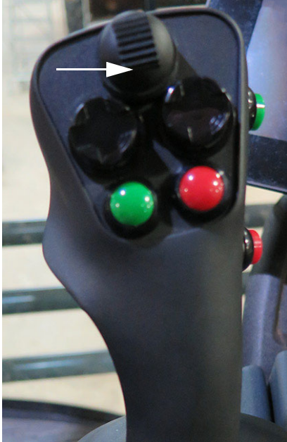
Transom Switch - DOWN (Located on the Hydrostatic Drive Control Handle) -Typical View
