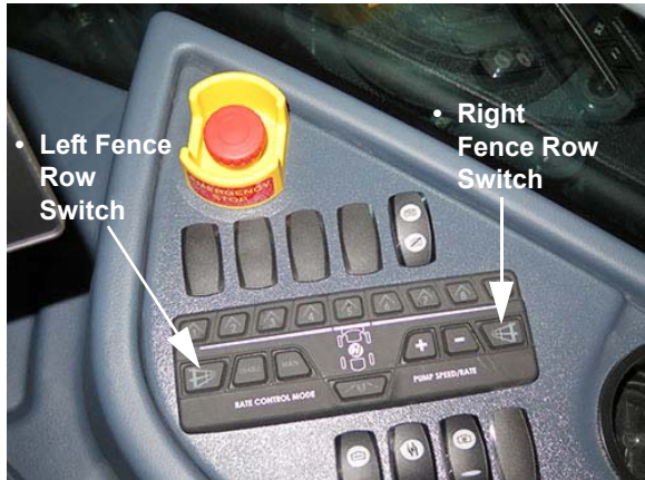
Fence Row Switches - Left and Right (Located on the side console) -Typical View
