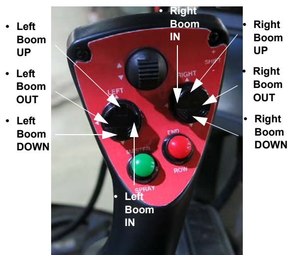
Left and Right-Hand Boom Switches (Located on the Hydrostatic Drive Control Handle) -Typical View
