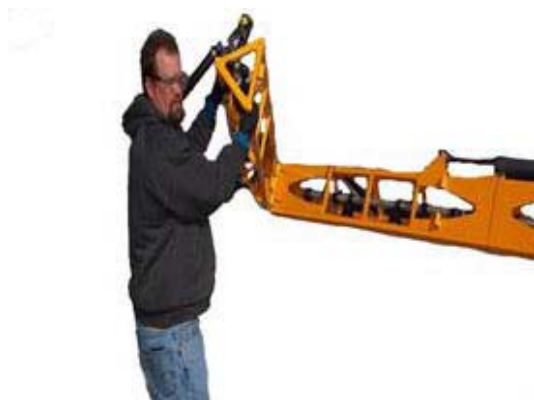
Securement Bolt (Located on the back side of boom) -Typical View
