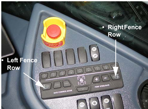
Fence Row Switches - Left/Right (Located on the side console) -Typical View
