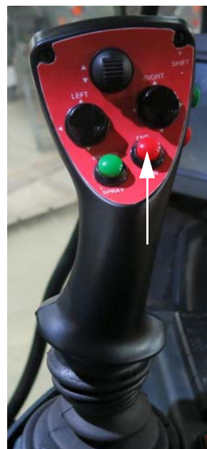
End Row Management Switch (Located on the Hydrostatic Drive Control Handle) -Typical View
