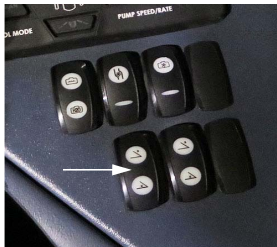
Boom Extension Switch * 90-ft. Spray Booms (Located on the side console) -Typical View
