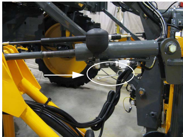
Level Cylinder Lock Valve (2) - 90/100' Boom (Located on each left and right-hand level cylinder) -Typical View
