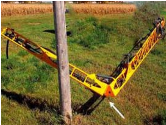
Outer Boom Breakaway -Typical View
