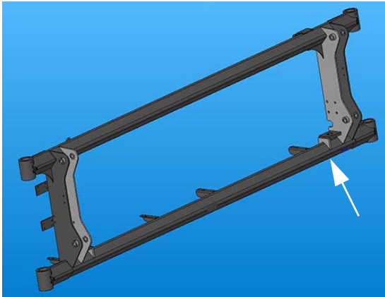
90/100' Steel Spray Boom Identification Plate -Typical View
