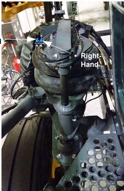
Air Suspension Valves (Located on the left-hand front air bag) -Typical View
