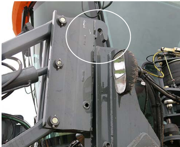
Attachment Clearing Mounting Pin -Typical View
