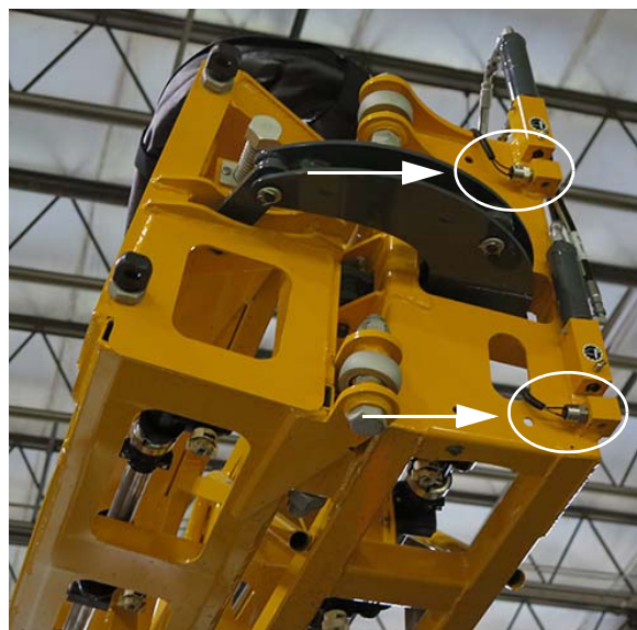
Outer Fold Latch Sensors -Typical View
