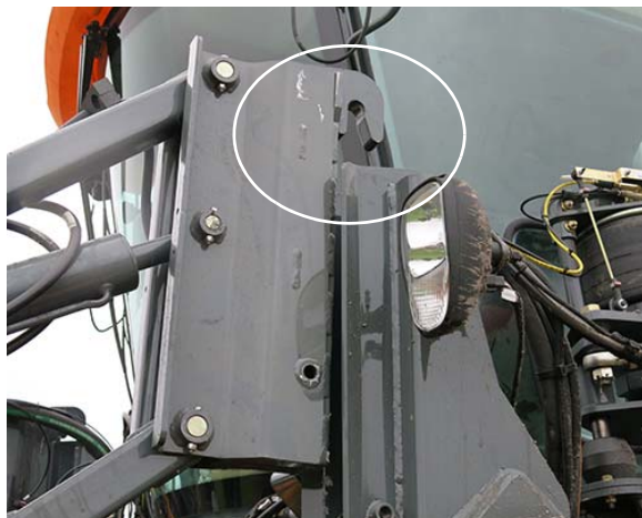
Attachment Clearing Mounting Pin -Typical View
