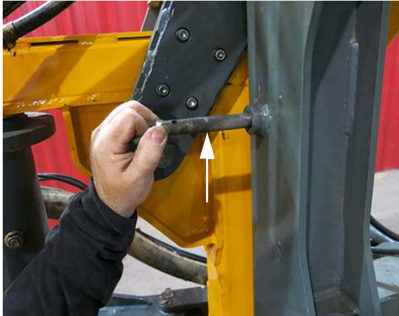
Mounting Bolt (Located on the outer side of transom frame) -Typical View
