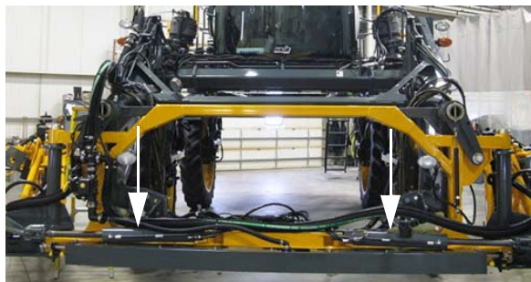
Main Pivot/Breakaway Cylinders -Typical View
