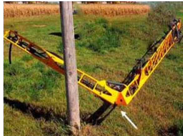
Outer Boom Breakaway -Typical View
