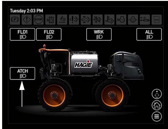
Attachment Lights Button (Located on the Machine Display Exterior Lighting Screen)
