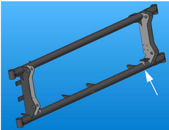
90/100' Steel Spray Boom Identification Plate -Typical View
