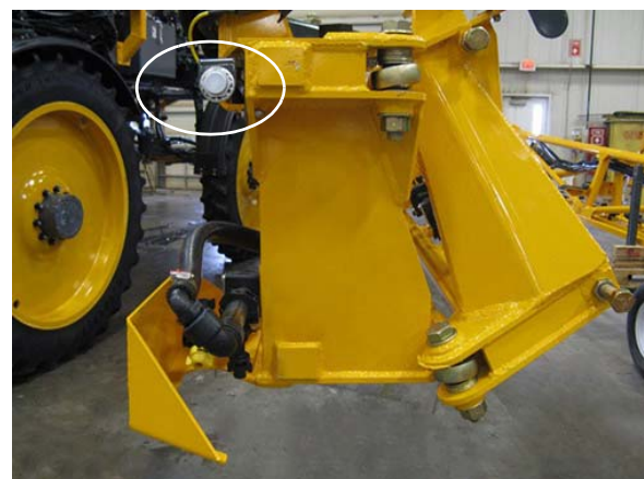
Proximity Sensors -Typical View
