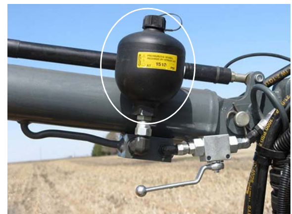
Accumulator -Typical View
