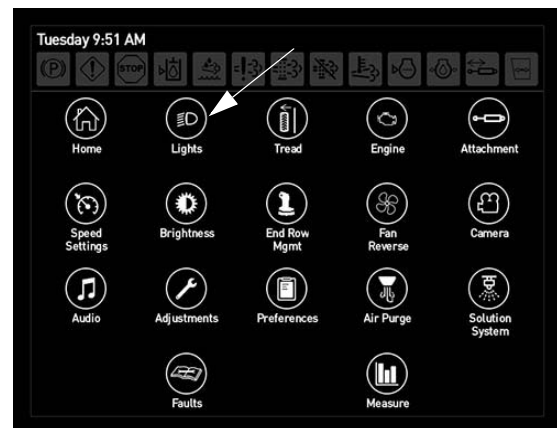
Lights Button (Located on the Machine Display Main Menu Page)
