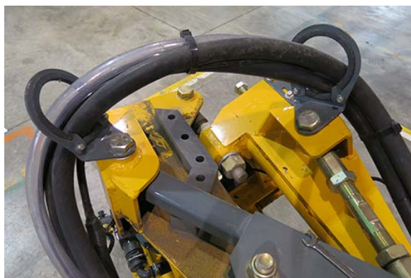
Boom Hose Clamp Installation -Typical View
