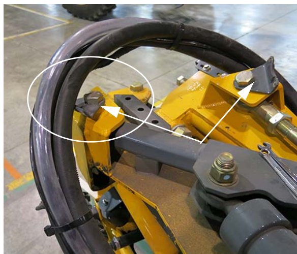
Hose Routing Brackets (2) (Located near the end of outer boom fold) -Typical View
