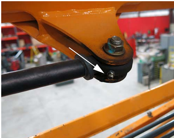
Boom Breakaway Cylinder Rod End -Typical View
