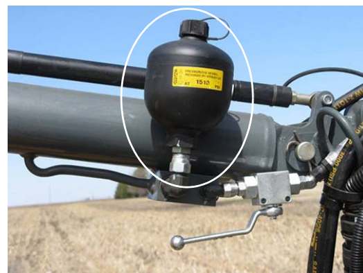
Accumulator -Typical View
