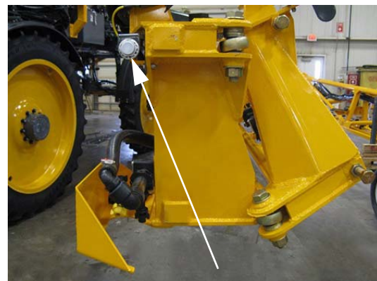
Proximity Sensors -Typical View
