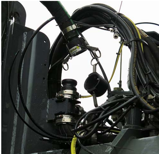
Solution Connection (Located on the front right-hand side of machine) -Typical View
