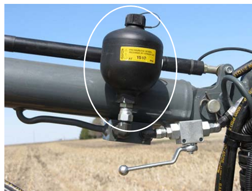
Accumulator -Typical View
