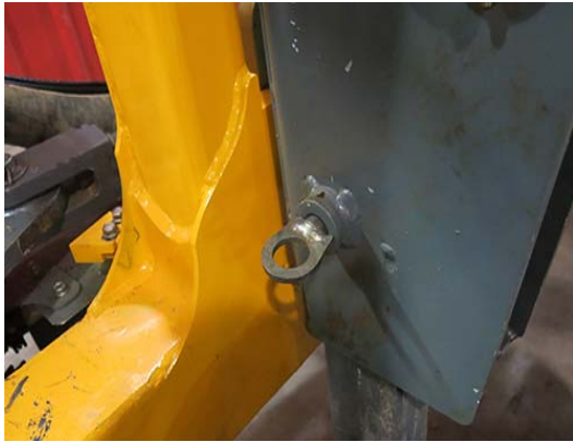
Lock Pin Removed -Typical View
