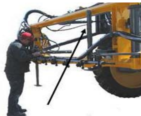
Boom Stand in "Travel" Position -Typical View
