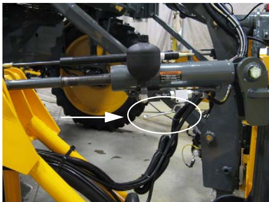
NORAC Hand Valve (2) - if equipped (Located on the left and right-hand level cylinders) -Typical View
