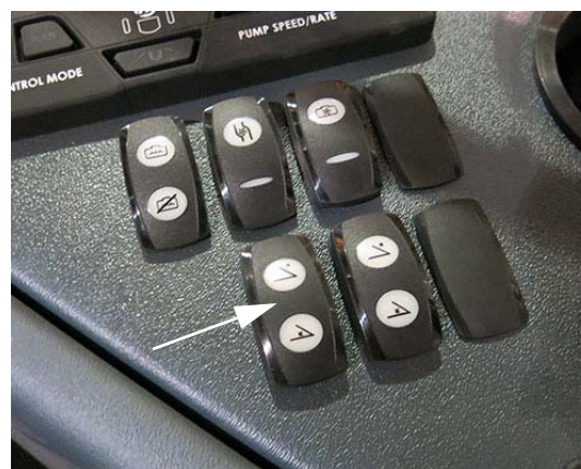
Boom Extension Switch * 90-ft. Spray Booms (Located on the side console) -Typical View
