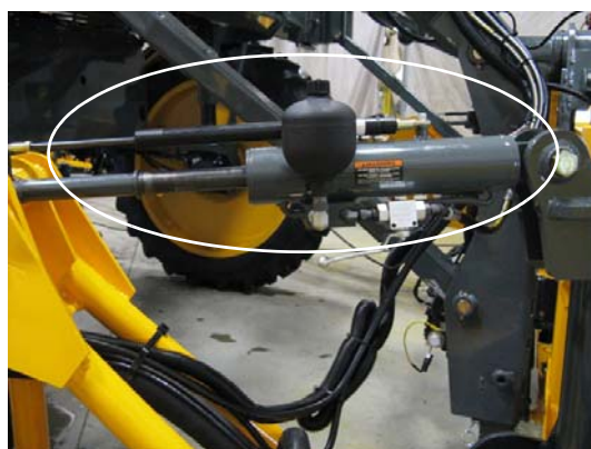
Level Cylinders -Typical View
