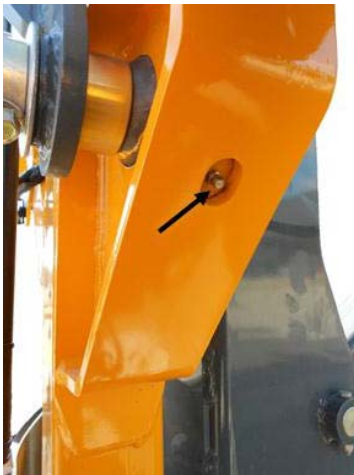
Pivot Transom Ball Joints -Typical View
