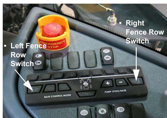
Fence Row Switches - Left and Right (Located on the side console) -Typical View
