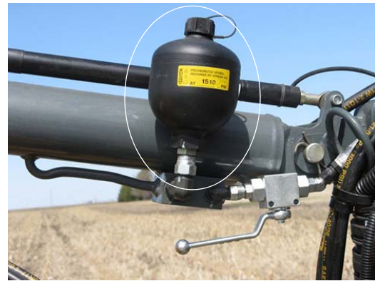
Accumulator -Typical View
