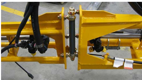
Outer Breakaway -Typical View
