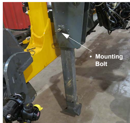
Boom Stand (Extended position shown) -Typical View
