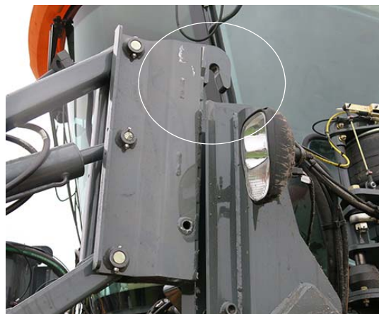
Attachment Clearing Mounting Pin -Typical View
