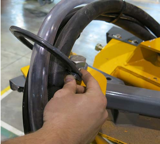
Boom Hose Clamp -Typical View
