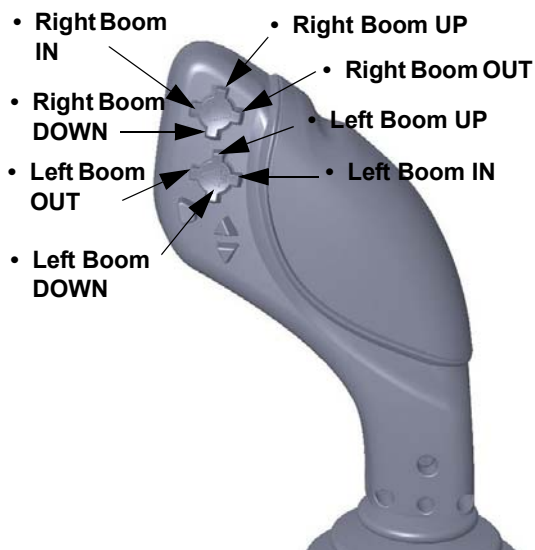
Left and Right-Hand Boom Switches (Located on the Hydrostatic Drive Control Handle - Version 1) -Typical View
