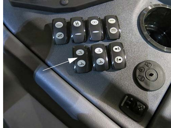
Boom Extension Switch * 90-ft. Spray Booms (Located on the side console) -Typical View
