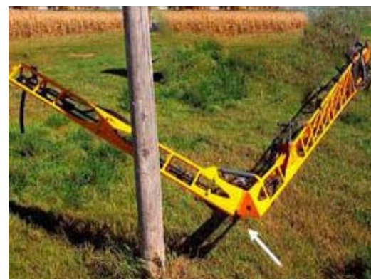
Outer Boom Breakaway -Typical View
