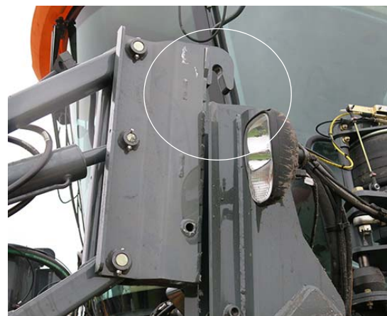
Attachment Clearing Mounting Pin -Typical View
