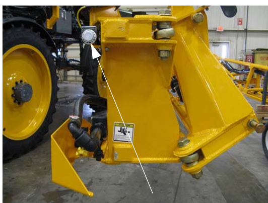
Proximity Sensors -Typical View
