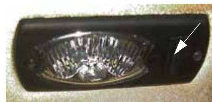
Interior Work Light Switch -Typical View
