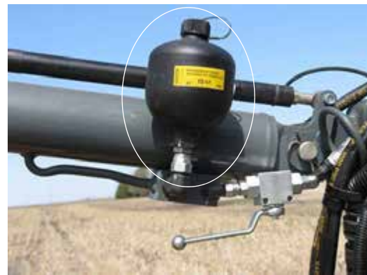
Accumulator -Typical View
