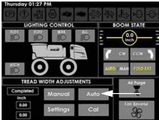
Auto Button (Located on the Machine Display Auxiliary Controls Page)
