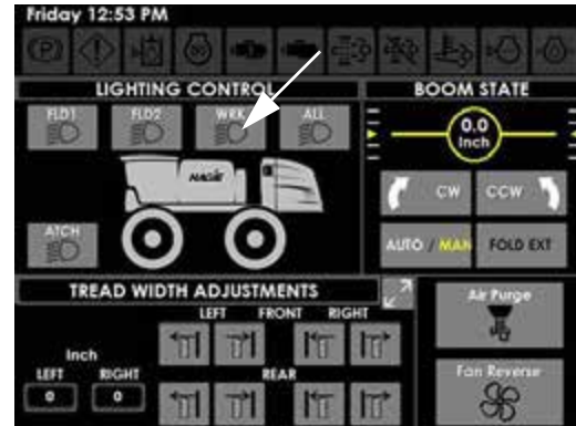
Work Lights Button
