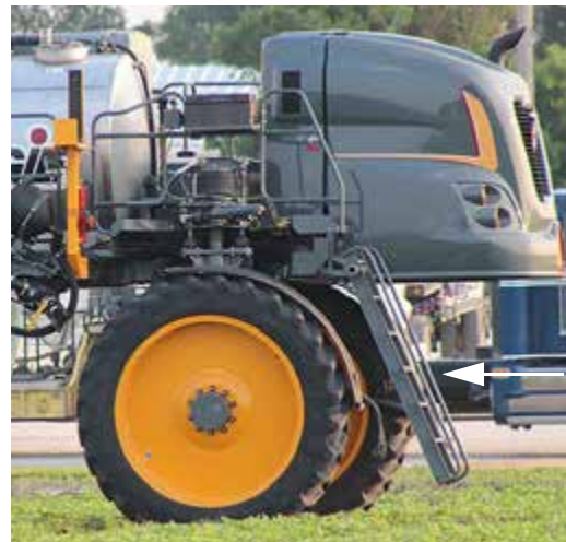
Ladder -Typical View * Lowered position shown
