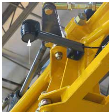
NORAC Sensor Foam Pad (Located on the bottom of each sensor) -Typical View
