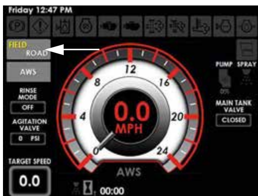
Field/Road Button (Located on the Machine Display Home Page)
