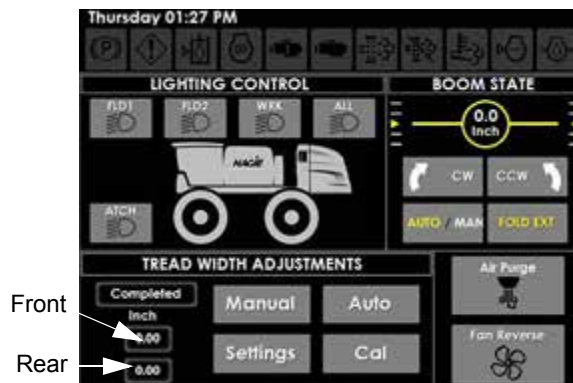
Front/Rear Tread Width Indicators (Located on the Machine Display Auxiliary Controls Page)
