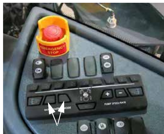
Rate Control Switches (Located on the side console) -Typical View
