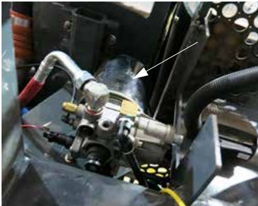
Air Dryer (Located beneath the right-hand side of machine) -Typical View
