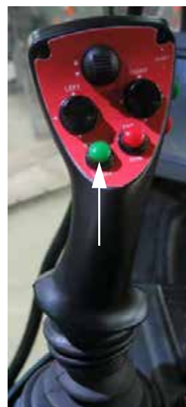
Master Spray Switch (Located on the Hydrostatic Drive Control Handle) -Typical View
