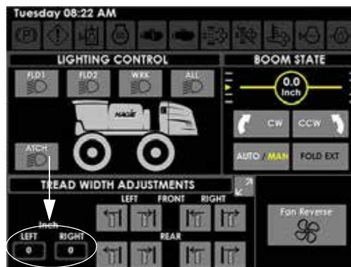
Left/Right Tread Width Indicators - Rear Legs (Located on the Machine Display Auxiliary Controls Page)
