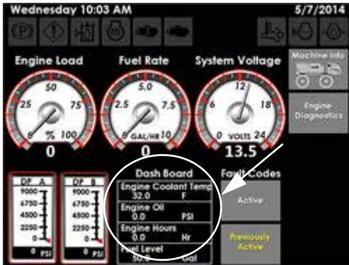
System Diagnostics (Located on the Machine Diagnostics Page)
