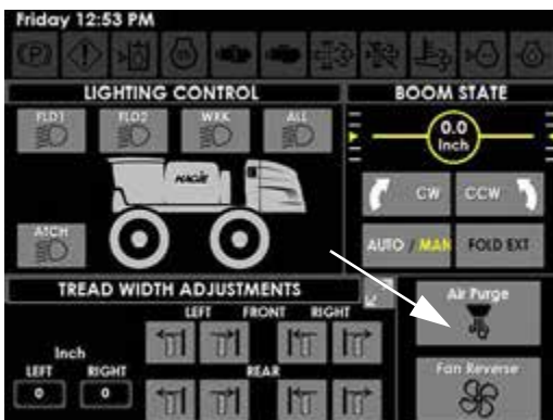
Air Purge Button (Located on the Auxiliary Controls Page)
