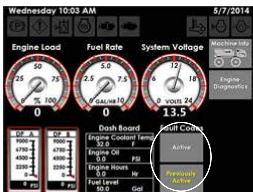
Fault Code Buttons (Located on the Machine Diagnostics Page)
