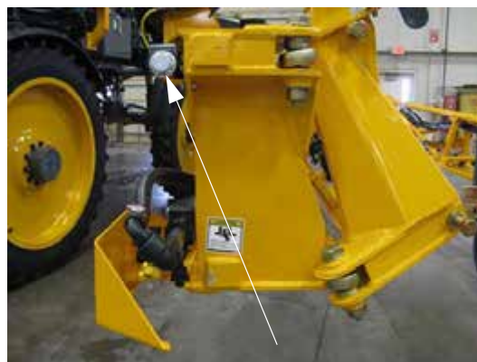
Proximity Sensors -Typical View
