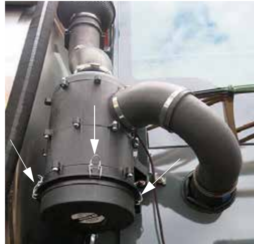
Filter Latches (4) (Located on the exterior filter housing) -Typical View
