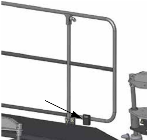
Hand Wash Foot Pedal (Located along the left-hand lower handrail) -Typical View
