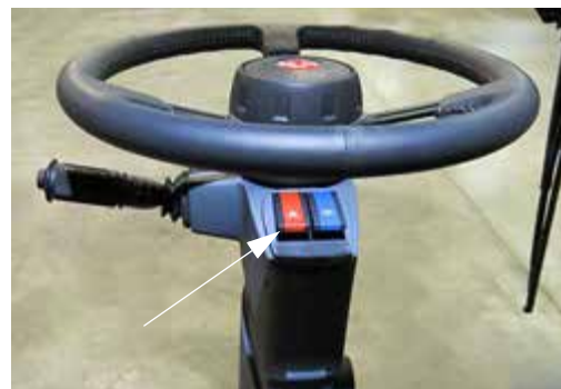
Hazard/Warning Lights Switch (Located on steering column)
