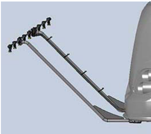
Rear Boom Installation -Typical View
