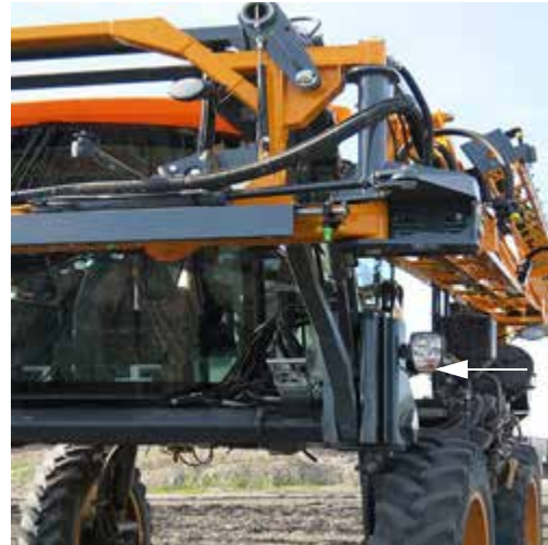
Hazard/Warning Lights (Located on each side of the front/rear machine and hood)
