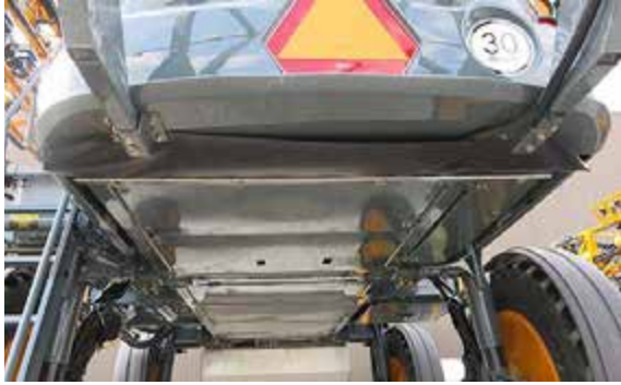
Belly Shield/Brush Curtain Installation -Typical View
