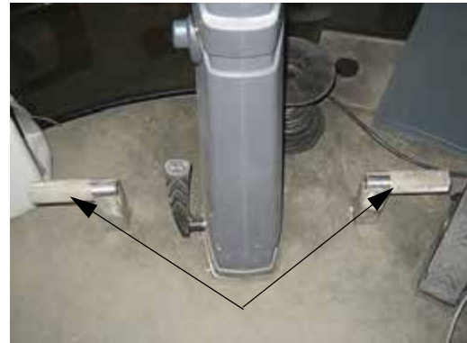
Operator Foot Pegs (Located on each side of the steering column) -Typical View
