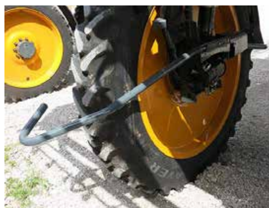
Installed Crop Divider -Typical View
