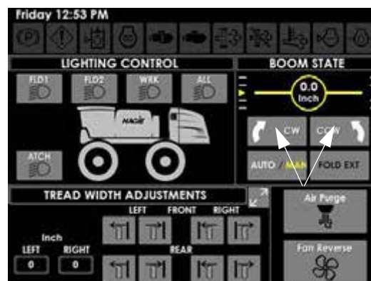
Roll Command Buttons (CW/CCW) (Located on the Machine Display Auxiliary Controls Page)
