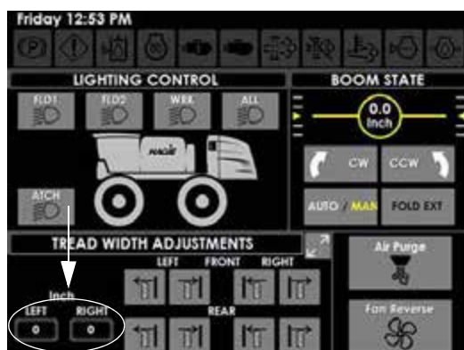
Left/Right Tread Width Indicators - Rear Legs (Located on the Machine Display Auxiliary Controls Page)
