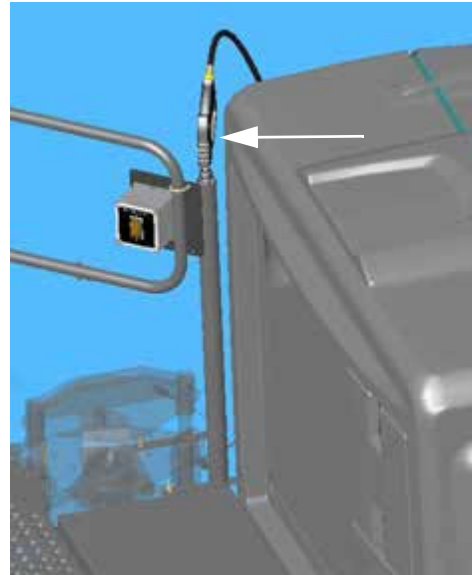
Pressure Washer Wand (Mounted on the rear right-hand handrail) -Typical View
