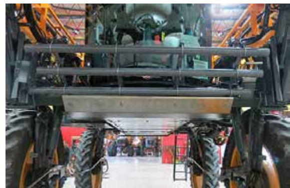
Brush Guard Installation -Typical View
