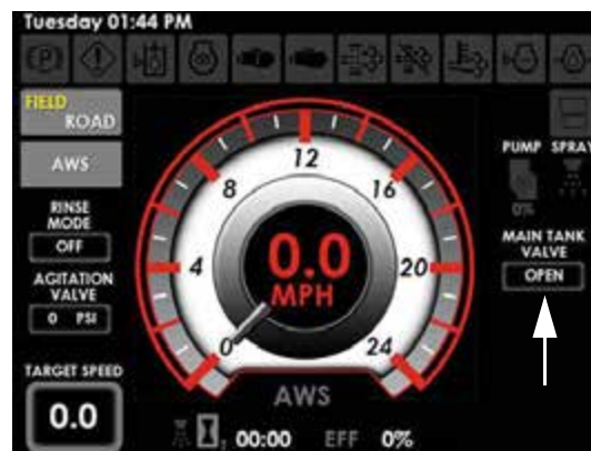
Main Tank Valve Status Indicator (Located on the Machine Home Page - Field Mode) -Typical View
