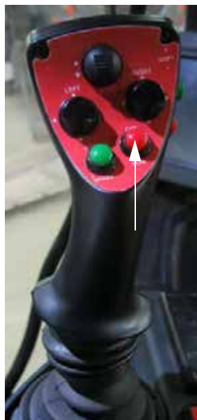
End Row Management Switch (Located on the Hydrostatic Drive Control Handle) -Typical View
