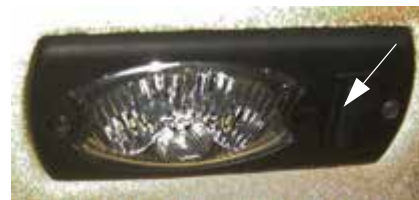
Interior Work Light Switch -Typical View
