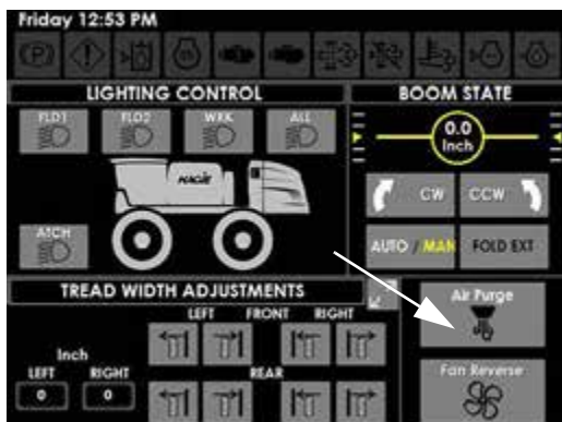
Air Purge Button (Located on the Auxiliary Controls Page)
