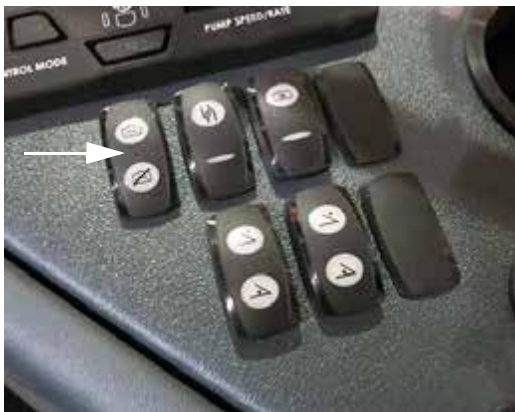
Main Tank Valve Switch (Located on the side console) -Typical View
