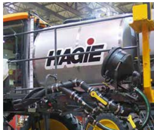
Solution Tank -Typical View
