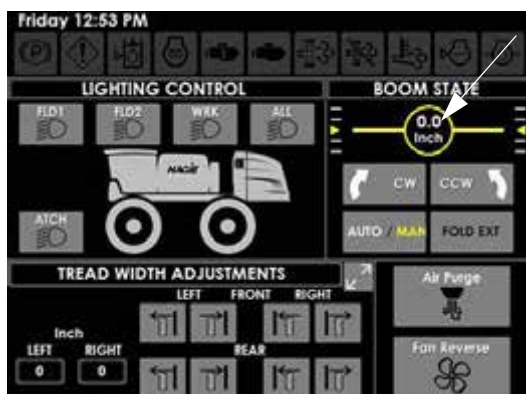
Boom Alignment Value (Located on the Machine Display Auxiliary Controls Page)
