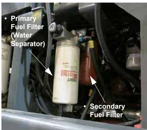
Primary and Secondary Fuel Filters (Located along left-hand side of machine - open hood to access) -Typical View
