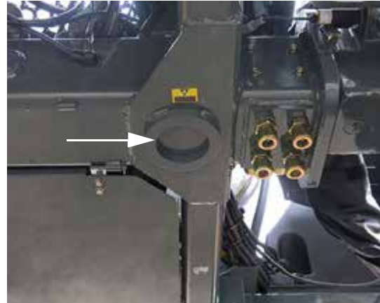
Lifting Point Containment Ring (Located on the frame near each leg) -Typical View
