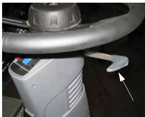
Steering Wheel Telescope Adjust Handle (Located to the right of the steering column) -Typical View
