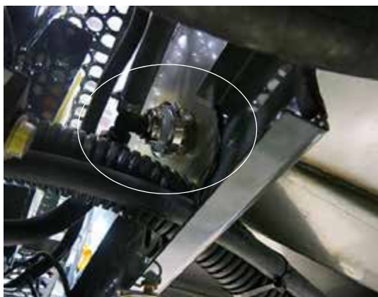
Jet Agitator (Located on each end of the solution tank) -Typical View
