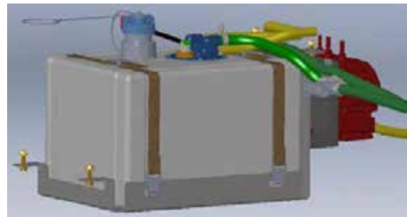
DEF Tank (Located beneath center of machine) -Typical View
