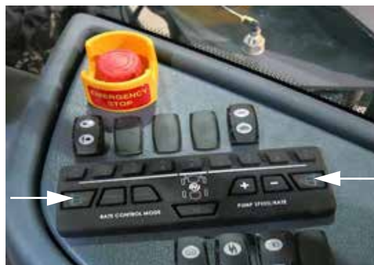
Fence Row Switches - Left/Right (Located on the side console) -Typical View
