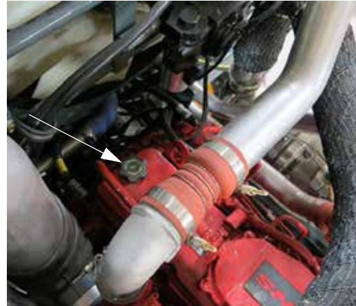
Engine Oil Fill (Located on top of engine) -Typical View
