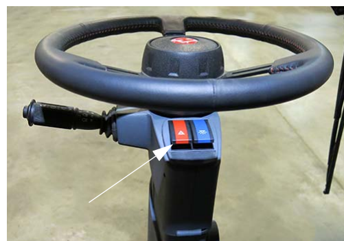
Hazard/Warning Lights Switch (Located on steering column)
