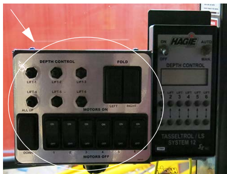
Detasseling Control Panel -Typical View
