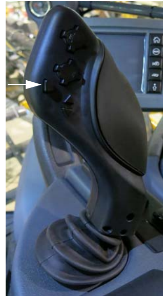
End Row Management Switch (Located on the Hydrostatic Drive Control Handle) -Typical View
