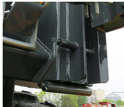
Lock Pin -Typical View * Engaged position shown
