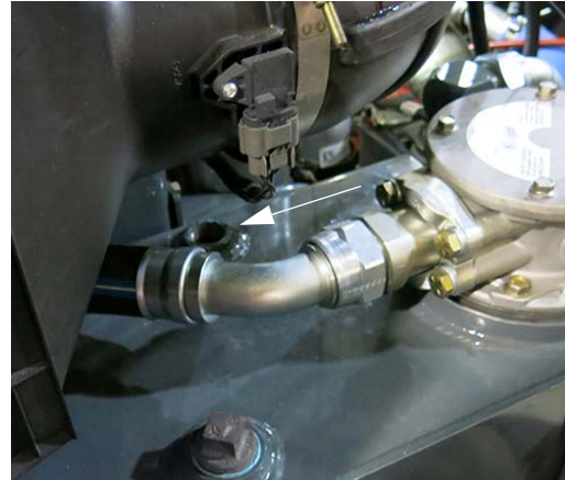
Breather Cap Removed -Typical View
