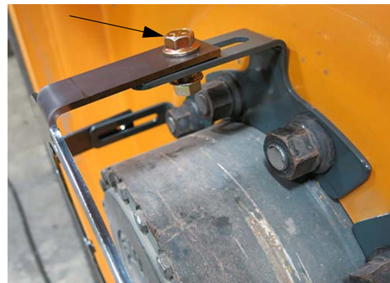
Hub Cap Adapter Bolt Installation -Typical View
