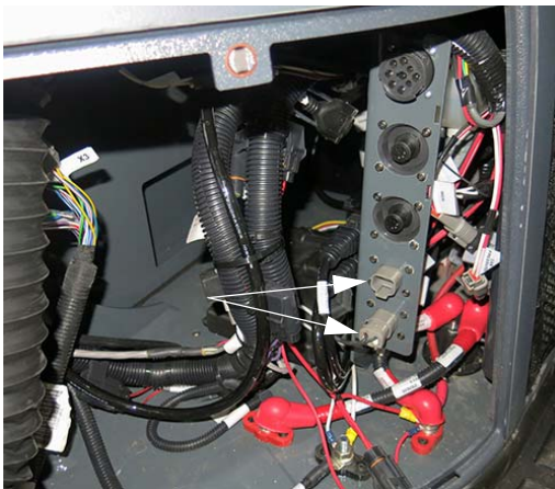
4-Pin Power Connectors (2) (Located inside the side console - remove front panel to access) -Typical View
