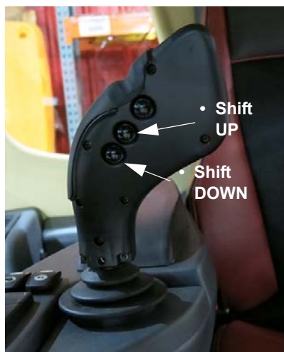
Shift Up/Down Switches (Located on the back side of the Hydrostatic Drive Control Handle) -Typical View
