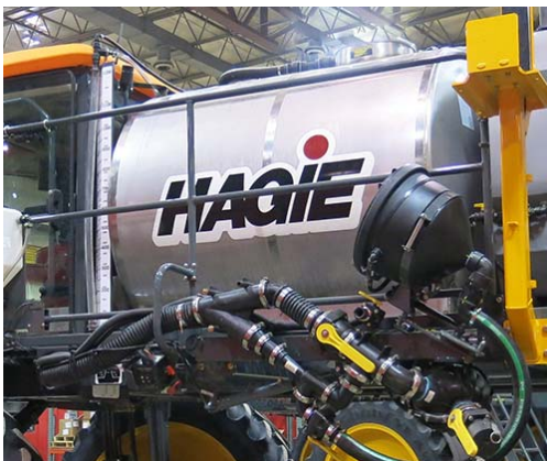
Solution Tank -Typical View
