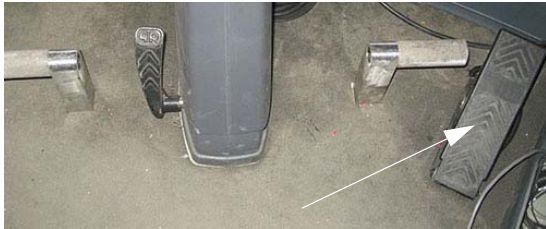
Decel Pedal (Located to the lower right-hand side of the steering column) -Typical View
