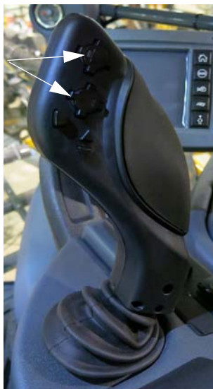
Left and Right Boom Switches (Located on the Hydrostatic Drive Control Handle) -Typical View
