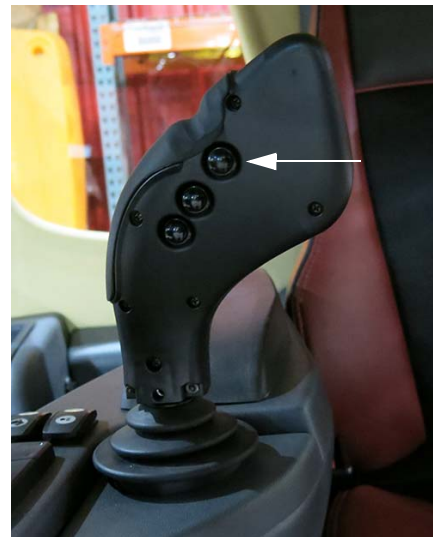
Master Spray Switch (Located on the back side of the Hydrostatic Drive Control Handle)
