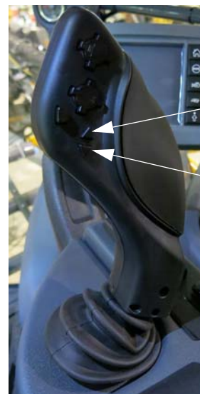
All-Up/Down Switches (Located on the Hydrostatic Drive Control Handle) -Typical View
