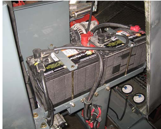
Battery Access (Located on the left-hand side of machine - open hood to access) -Typical View
