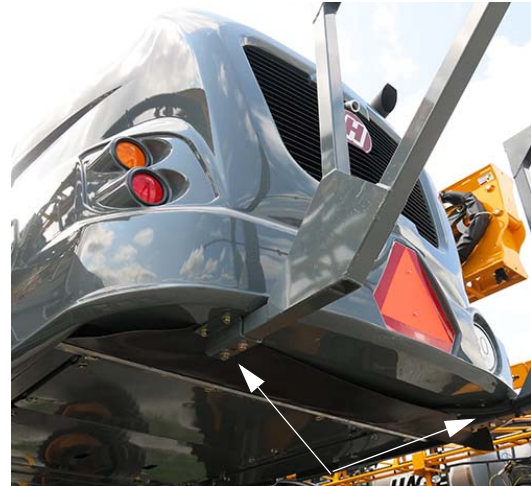
Brush Curtain Attached to Hood -Typical View
