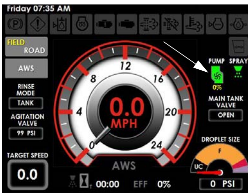
Solution Pump Indicator (Located on the Machine Display Home Page - Field Mode)
