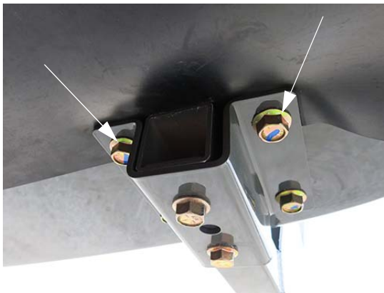
Mounting Bolts (Two located on each side of hood bracket) -Typical View
