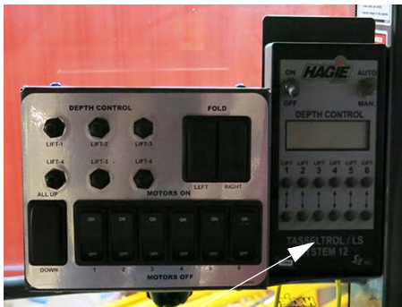
Tasselrol Control Panel -Typical View
