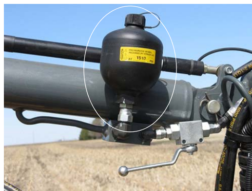
Accumulator -Typical View
