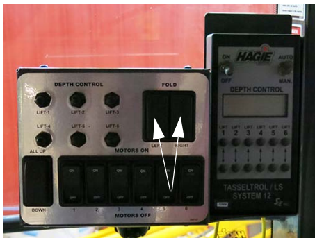
Left/Right Fold Switches (Located on the Detasseling Control Panel) -Typical View
