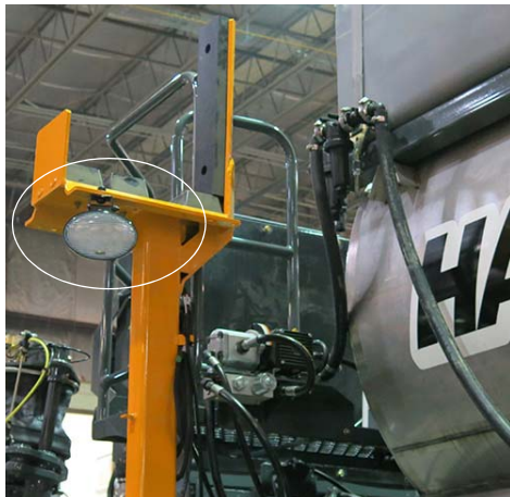
Work Lights (Located on each boom cradle) -Typical View
