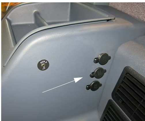
12V Power Ports -Typical installation shown
