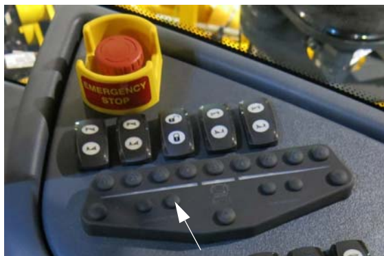
Manual "MAN" Rate Control Switch (Located on the side console) -Typical View
