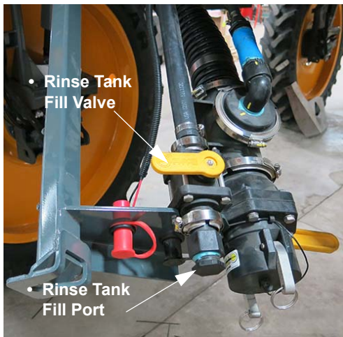
Front Fill Assembly (Lowered position shown) -Typical View
