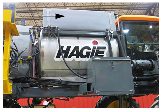
Rinse Tank -Typical View
