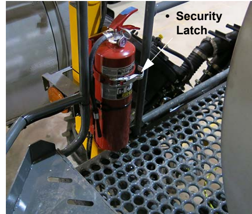
• Security Latch Fire Extinguisher (Located along the catwalk on left-hand side of machine) -Typical View
