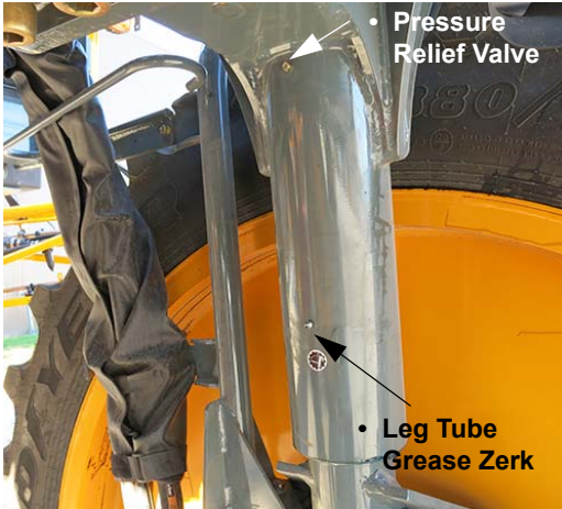
Leg Tube Grease Zerk and Pressure Relief Valve (Located on front and rear legs) -Typical View
