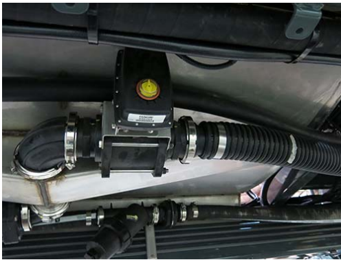
Solution Tank Valve -Typical View
