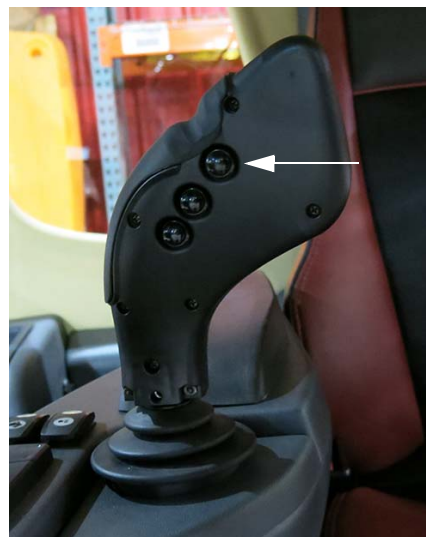
Master Spray Switch (Located on the back side of the Hydrostatic Drive Control Handle)
