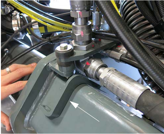
Brush Guard Mounting Bracket (Right-hand side of machine shown) -Typical View
