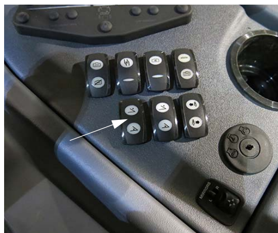
Boom Extension Switch *90-ft. Spray Booms (Located on the side console) -Typical View
