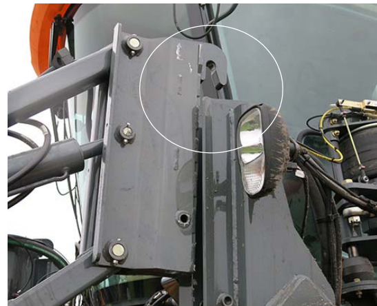
Attachment Clearing Mounting Pin -Typical View
