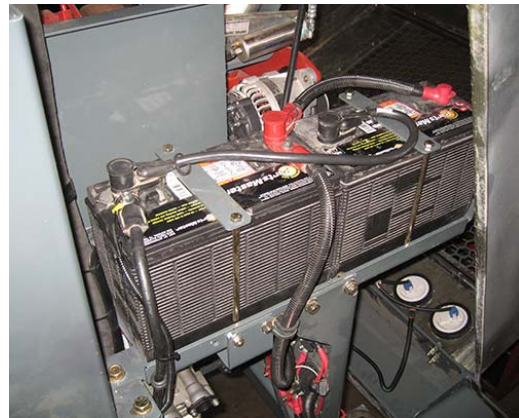
Battery Access (Located on the left-hand side of machine - open hood to access) -Typical View
