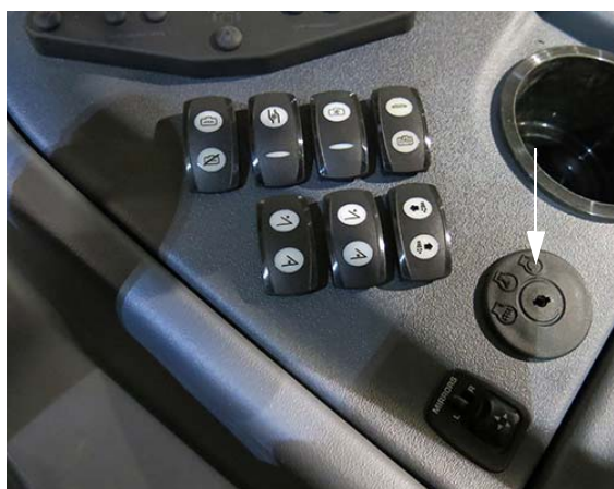
Ignition Switch (Located on the side console) -Typical View
