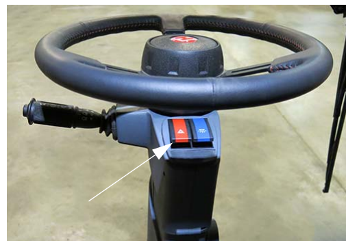
Hazard/Warning Lights Switch (Located on steering column)
