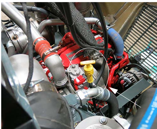
Engine Oil Dipstick (Located on the left-hand side of engine - open hood to access) -Typical View
