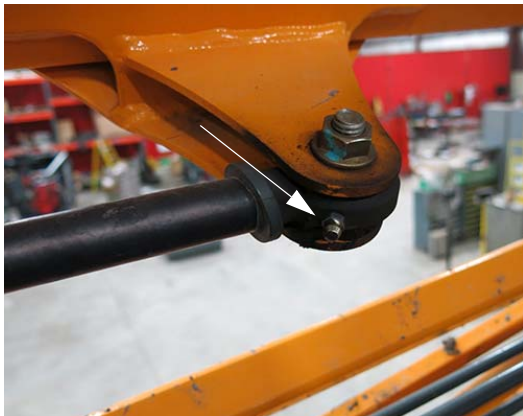
Boom Breakaway Cylinder Rod End -Typical View
