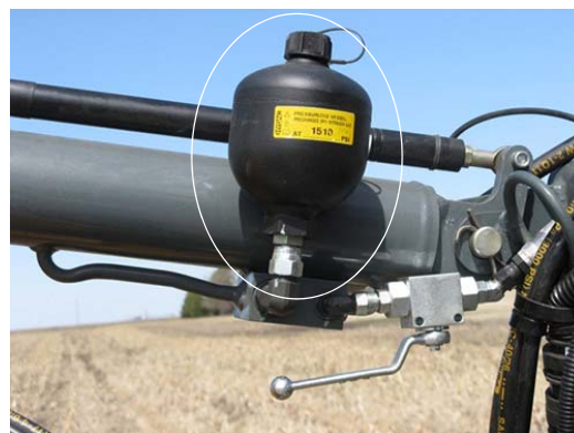
Accumulator -Typical View
