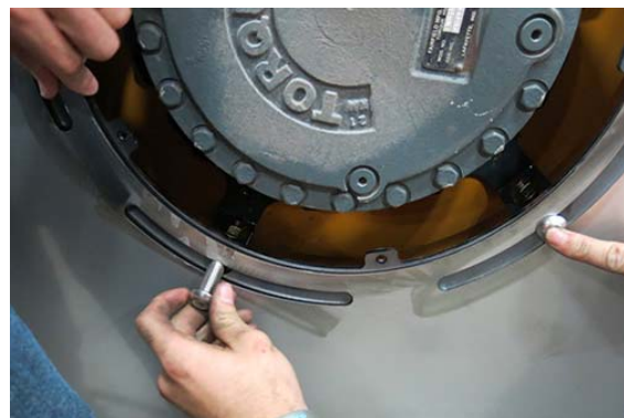
Wheel Cover Mounting Bolt Installation -Typical View
