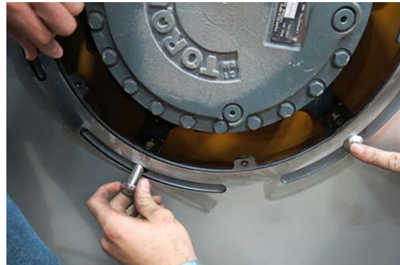
Wheel Cover Mounting Bolt Installation -Typical View
