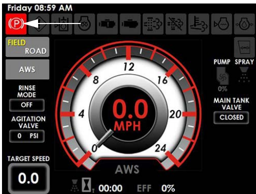
Parking Brake Indicator (Located on the top left-hand side of each Machine Display page)
