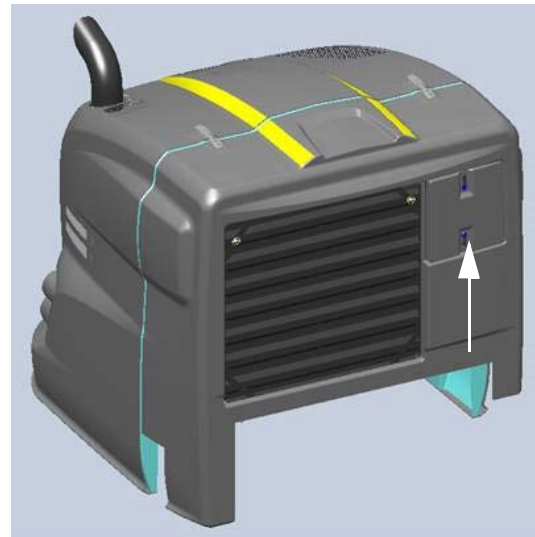
Engine Air Intake Filter Access Panel (Located on left-hand side of hood) -Typical View
