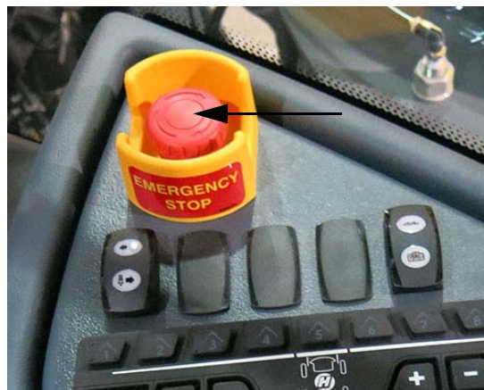
E-Stop Switch (Located on the side console) -Typical View
