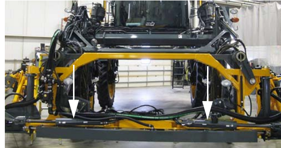
Main Pivot/Breakaway Cylinders -Typical View
