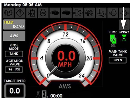
Master Spray Indicator (Located on the Machine Display Home Page - Field Mode)
