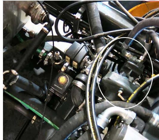
Solution Pump (Located near center of machine) -Typical View
