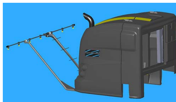
Rear Boom Installation -Typical View
