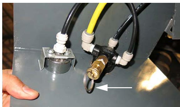
Pressure Relief Pull Ring (Located on the back side of the foam pressure regulator) -Typical View
