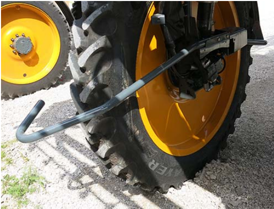
Installed Crop Divider -Typical View
