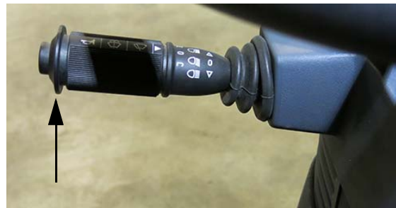
Windshield Washer Button (Located on the end of the turn signal lever) -Typical View
