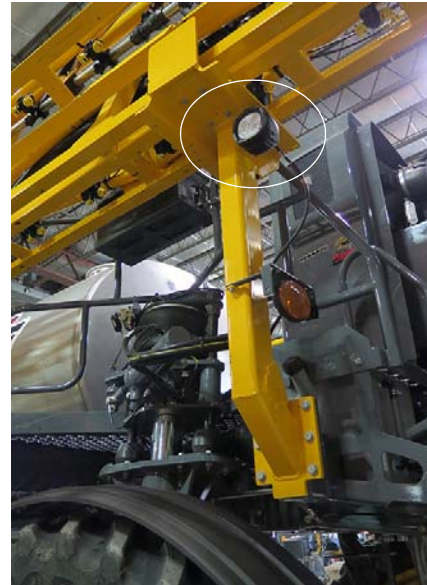
Work Lights (2) (Located on each boom cradle) -Typical View
