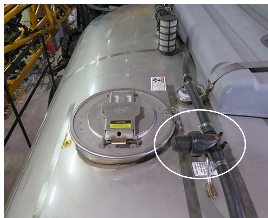
Tank Rinse Strainer (Located on top of solution tank) -Typical View
