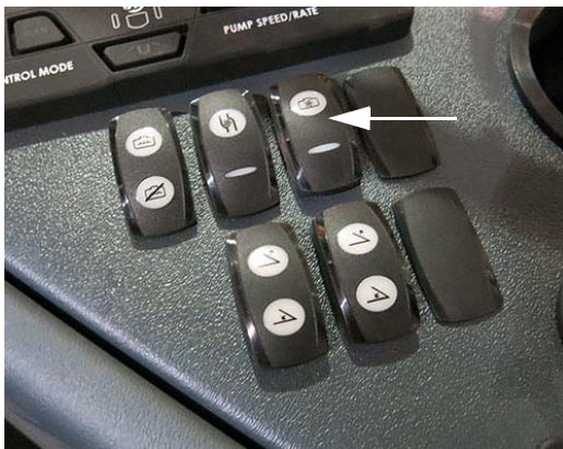
Agitation Valve Switch (Located on the side console) -Typical View
