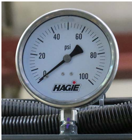
Pressure Gauge (Mounted on boom) -Typical View
