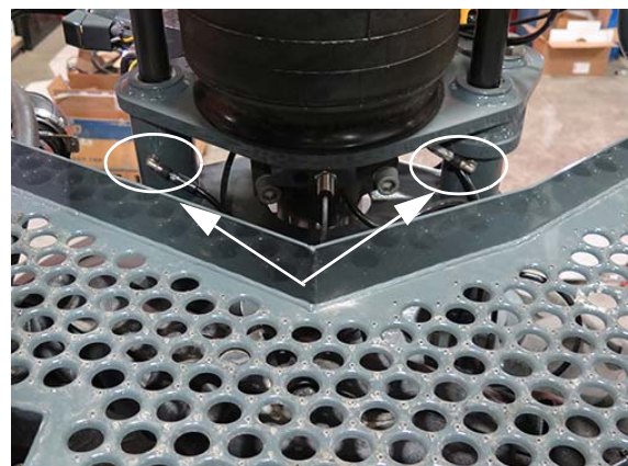
Tower Bearing Grease Zerks (8) (Located on the front and rear legs) -Typical View
