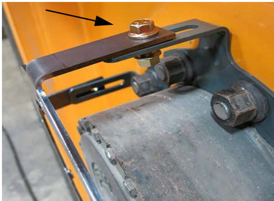
Hub Cap Adapter Bolt Installation -Typical View
