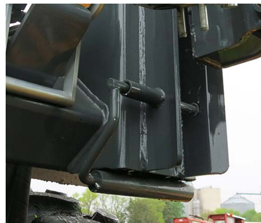
Lock Pin -Typical View * Engaged position shown
