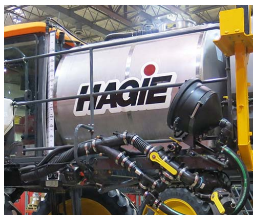
Solution Tank -Typical View
