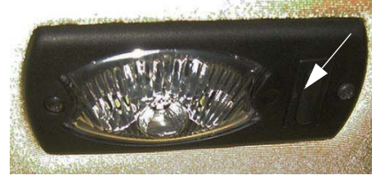
Interior Work Light Switch -Typical View
