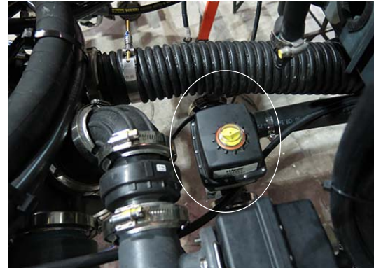
Agitation Valve (Located near center of machine) -Typical View * View shown from top of machine
