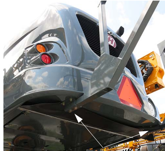
Brush Curtain Attached to Hood -Typical View
