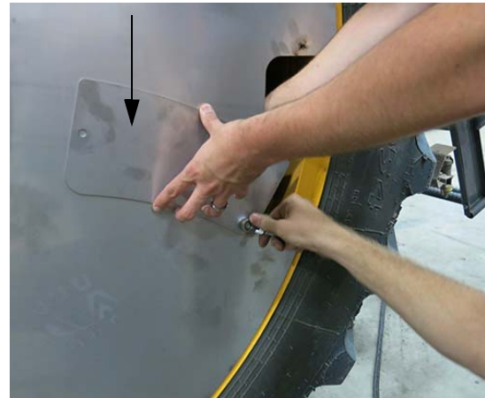
Valve Stem Access Panel -Typical View
