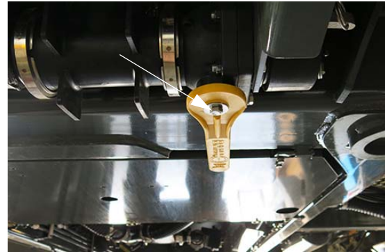
Front Fill Valve Bolt -Typical View
