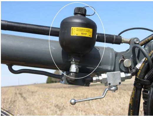
Accumulator -Typical View
