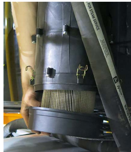
Filter Removal -Typical View
