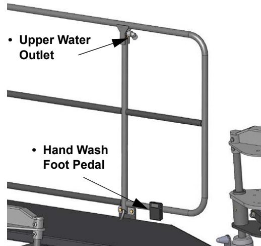
Upper Water Outlet/Hand Wash Foot Pedal (Located along lower handrail on left-hand side of machine) -Typical View
