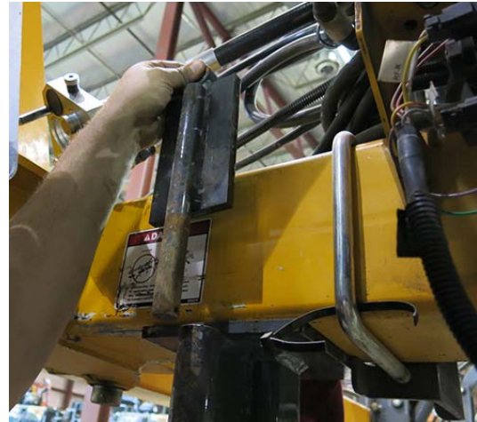
Stop Plate (Located on the inward side of each combo attachment stand) -Typical View
