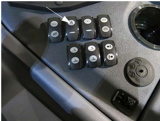
Solution Pump Switch (Located on the side console) -Typical View
