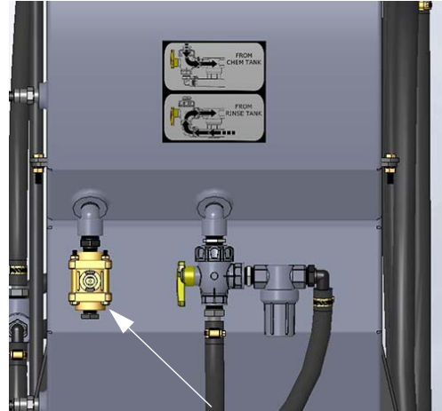
Tank Drain Valve -Typical View
