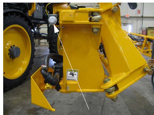
Proximity Sensors -Typical View
