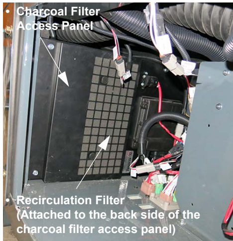
Charcoal Filter Access Panel (Located behind exterior service panel on right-hand side of cab) -Typical View
