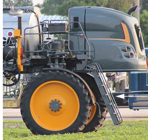
Ladder -Typical View * Lowered position shown
