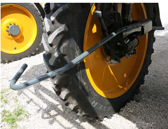
Installed Crop Divider -Typical View
