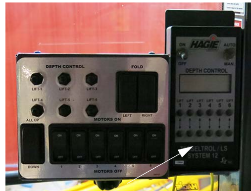
Tasselrol Control Panel -Typical View
