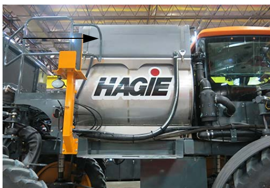
Rinse Tank -Typical View
