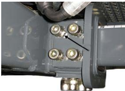
Jam Nut (Located on each tread adjust bearing bolt) -Typical View
