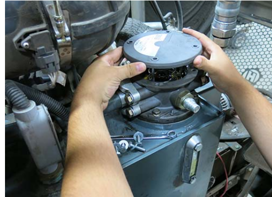
Filling Tank Through Hydraulic Return Filter Housing -Typical View
