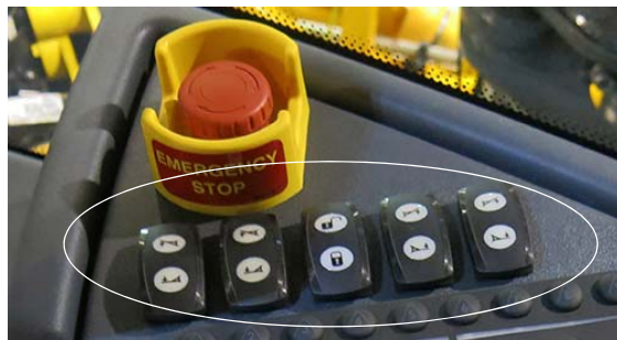
60' NTB Switches (Located on the side console) -Typical View
