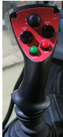
Hydrostatic Drive Control Handle (Version 2) -Typical View
