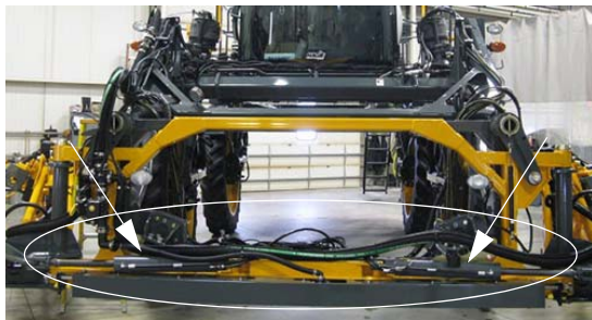
Main Pivot/Breakaway Cylinders -Typical View
