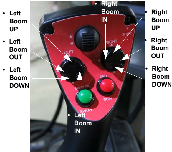
Left and Right-Hand Boom Switches (Located on the Hydrostatic Drive Control Handle - Version 2) -Typical View
