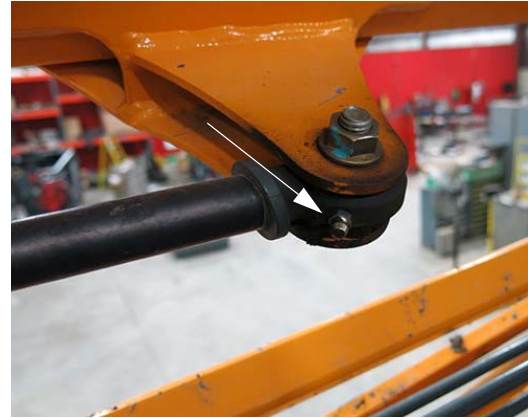
Boom Breakaway Cylinder Rod End -Typical View
