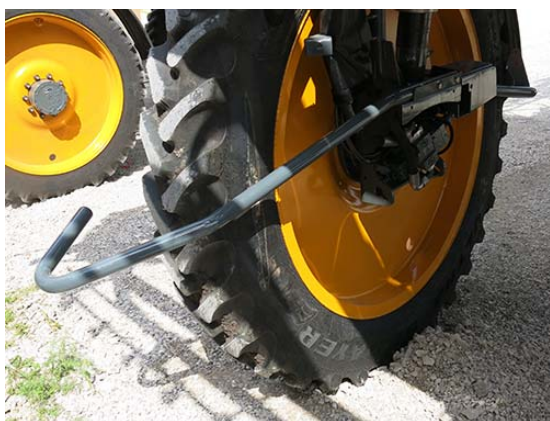
Installed Crop Divider -Typical View
