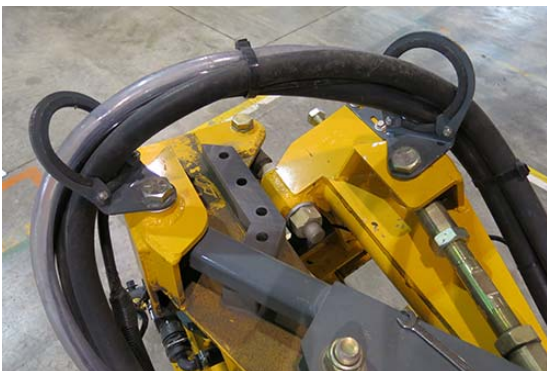
Boom Hose Clamp Installation -Typical View
