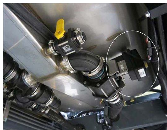
Solution Tank Valve (Located beneath the solution tank on underside of machine) -Typical View
