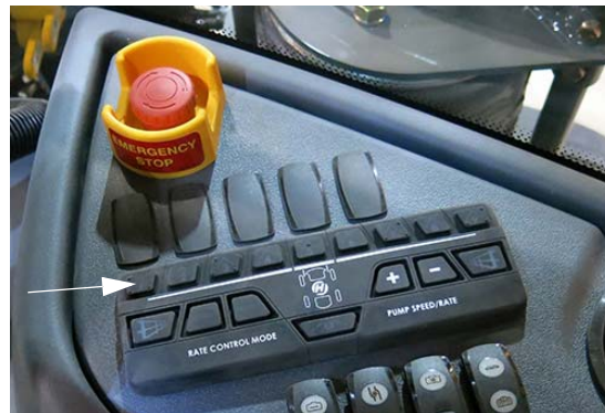
Boom Solution Valve Switches (Located on the side console) -Typical View
