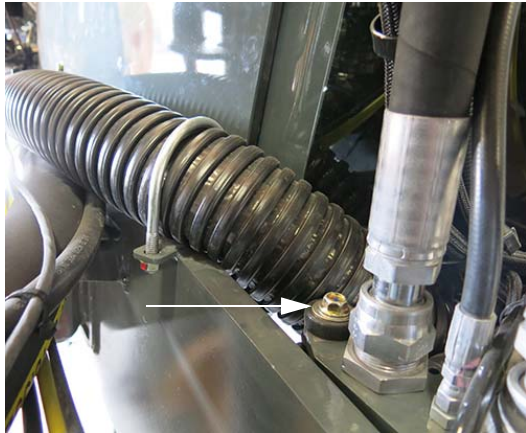
Mounting Bolts (2) - Front/Rear (Located on the right-hand cross member hose assembly mounting bracket) -Typical View *Rear bolt shown
