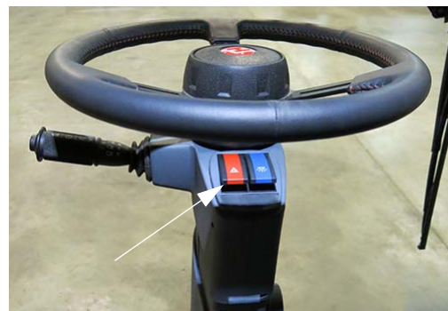
Hazard/Warning Lights Switch (Located on steering column)
