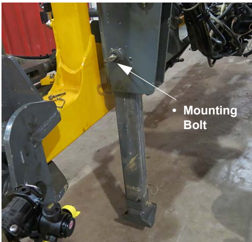
Boom Stand (Extended position shown) -Typical View
