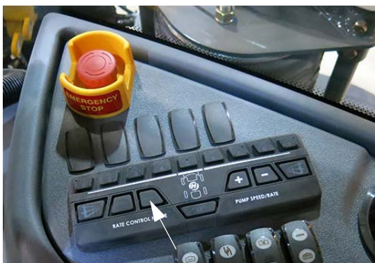
Manual “MAN” Rate Control Switch (Located on the side console) -Typical View
