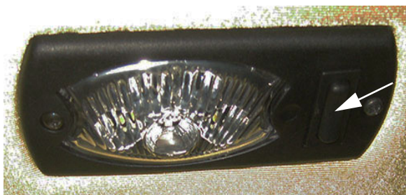
Interior Work Light Switch -Typical View
