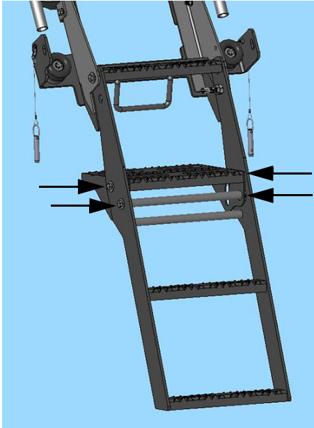
Lower Ladder Pivot Points - Platform (4) -Typical View
