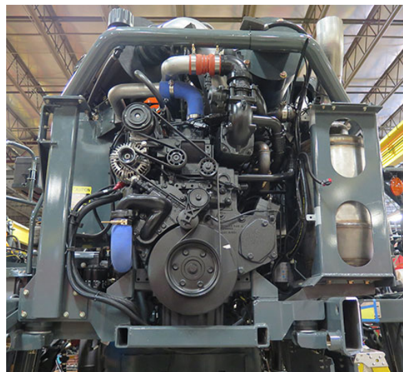
John Deere Final Tier 4 PSS 9.0L Diesel Engine - STS14/STS16 -Typical View
