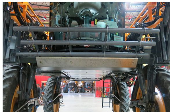
Brush Guard Installation -Typical View
