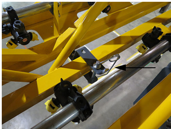
Transport Lock Pin (2) (Located on each side of boom - Section 2) -Typical View * Shown in the “transport” position
