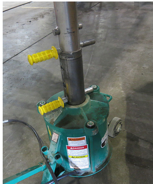
Lock Pin Installation -Typical View
