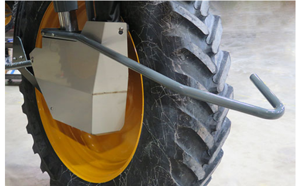
Installed Crop Divider -Typical View
