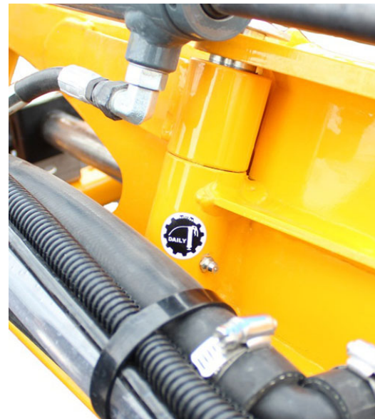
Boom Breakaway -Typical View
