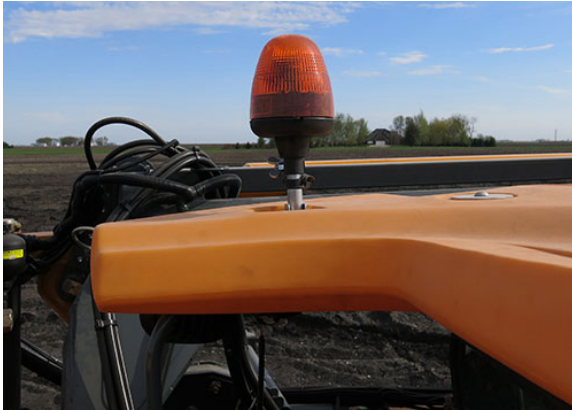
Rotating Beacon (Located on front roof cap) -Typical View
