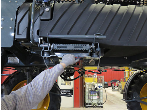
Lower Ladder Handle -Typical View
