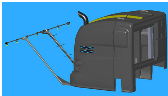
Rear Boom Installation -Typical View
