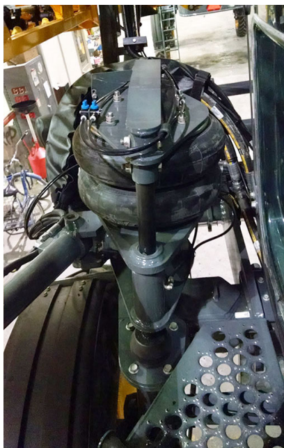
Air Bag (Located on each leg) -Typical View * Front Air Bag Shown
