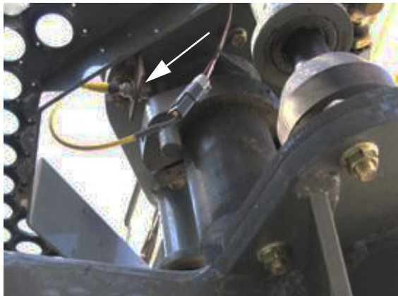
External Proximity Sensor -Typical View
