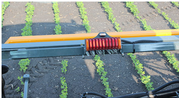
Boom Solution Valve Indicators (Located on transom) -Typical View
