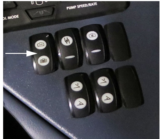
Tank Valve Selector Switch (Located on the side console) -Typical View
