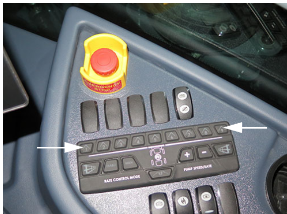
Boom Solution Valve Switches - Sections 1 and 9 (Located on the side console) -Typical View
