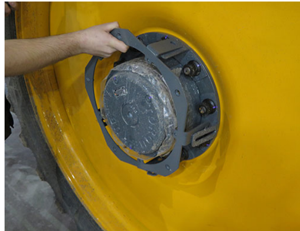
Hub Cap Adapter Weldment -Typical View
