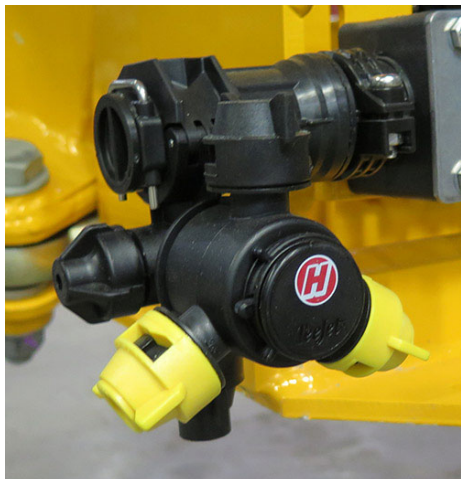
Nozzle Body (Located throughout boom) -Typical View
