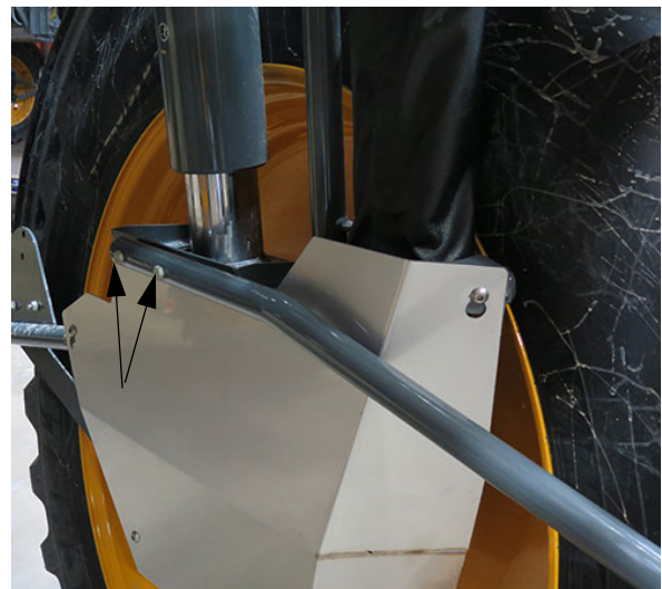
Crop Divider Mounting Bolts (2) -Typical View
