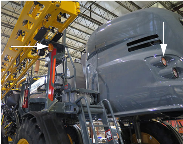
Rear Hazard/Warning Light Flashers (4) -Typical View
