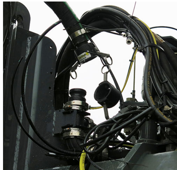
Solution Connection - Standard (Located on the front right-hand side of machine) -Typical View
