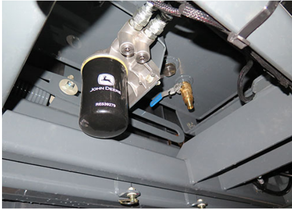
Engine Oil Filter (Located on rear left-hand side of machine below hydraulic oil reservoir) -Typical View
