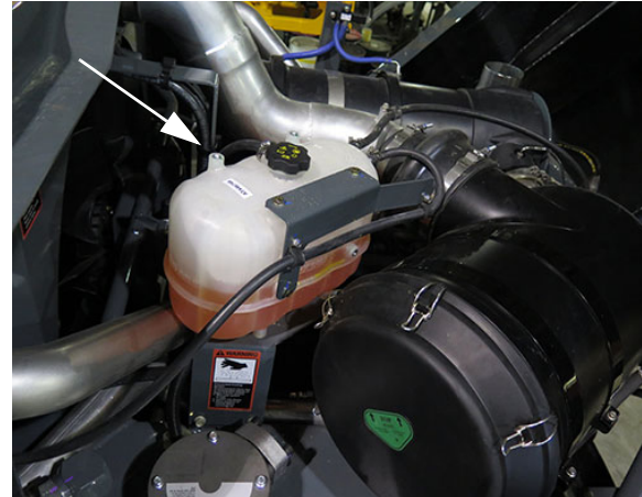
Surge Tank - STS14/STS16 (Located near the rear of machine - open hood to access) -Typical View
