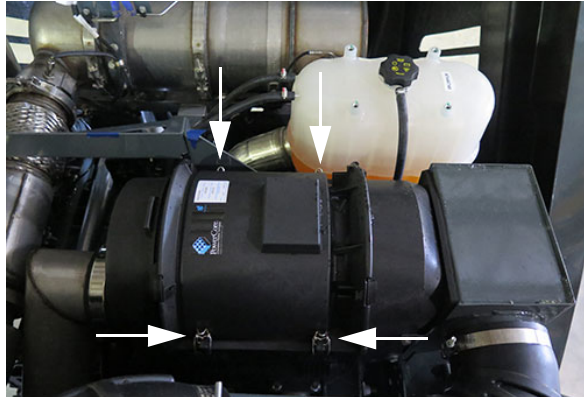
Security Latches (4) - STS10/STS12 (Located on each side of filter housing) -Typical View
