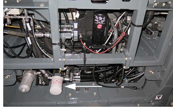
Case Drain Filter 2 (Located on left-hand side of machine ahead of engine frame) -Typical View
