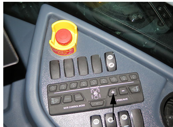
"+" Pump Speed/Rate Switch (Located on the side console) -Typical View
