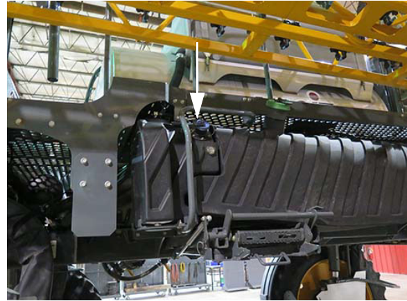
DEF Fill Cap (Located on front of DEF tank) -Typical View
