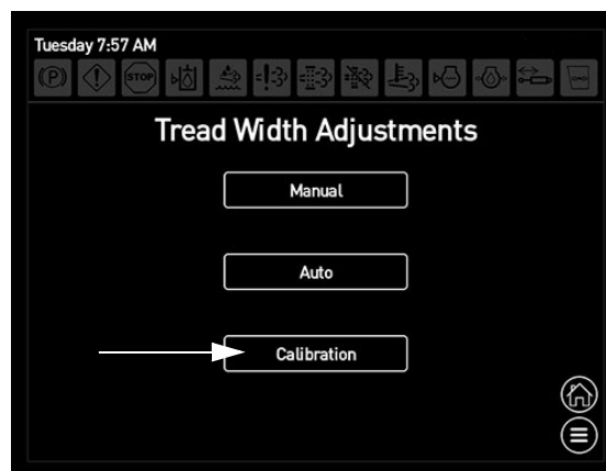
Calibration Button (Located on the Tread Width Adjustments Screen)
