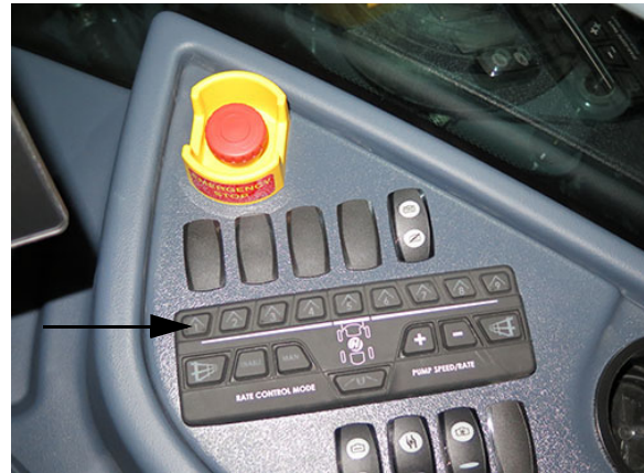
Boom Solution Valve Switches - Single Product Section Keypad (Located on the side console) -Typical View
