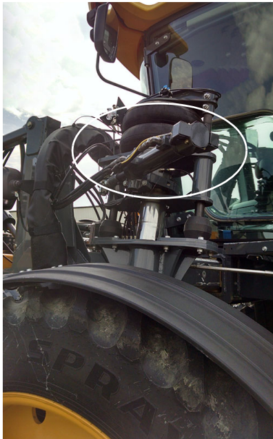
Steering Cylinder -Typical View
