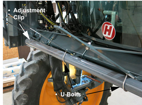
Brush Guard Tube -Typical View
