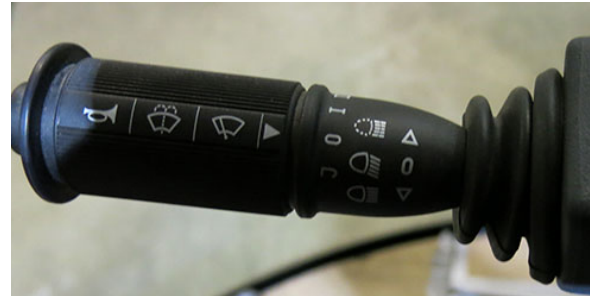
Turn Signal Lever -Typical View
