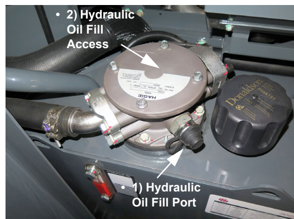
Hydraulic Oil Fill Options -Typical View
