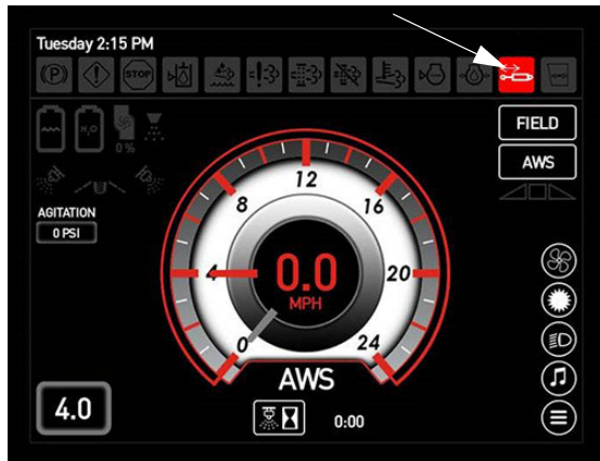
Boom Charge Indicator - 120' Hybrid Booms (Located along the top of each display page)
