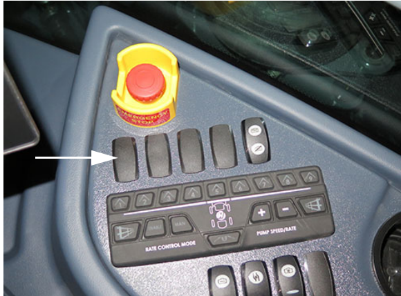
Foam Marker Switch (Located on the side console) -Typical View
