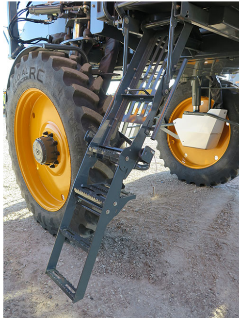
Fuel Fill Ladder (Lowered position shown) -Typical View
