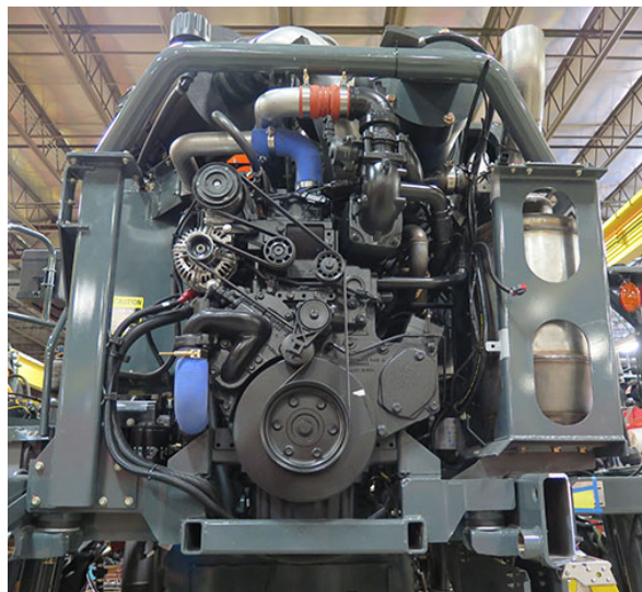
Final Tier 4 Diesel Engine (PSS 9.0L) - STS14/STS16
