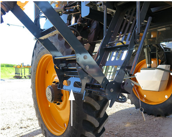
Ladder Platform -Typical View
