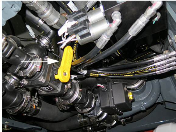
Agitation Shutoff Valve (Located beneath rear of machine) -Typical View * Agitation Shutoff Valve shown in the CLOSED position (Dual Product Mode)
