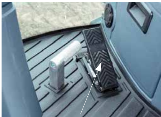
Decel Pedal (Located to the lower right-hand side of the steering column) -Typical View
