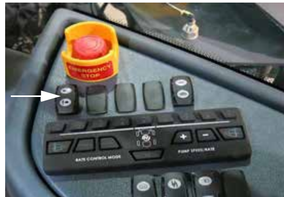
Foam Marker Switch (Located on the side console) -Typical View
