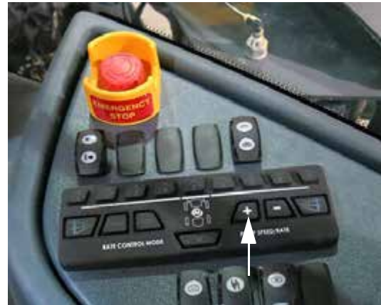
“+” Pump Speed/Rate Switch (Located on the side console) -Typical View
