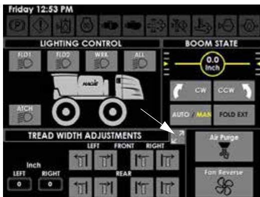
Tread Page Button (Located on the Machine Display Auxiliary Controls Page)
