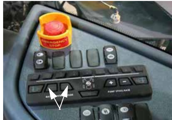
Rate Control Switches (Located on the side console) -Typical View
