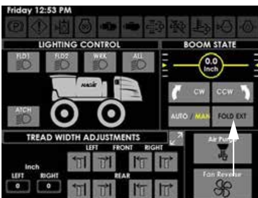
Fold Extension Button (Located on the Auxiliary Controls Page)
