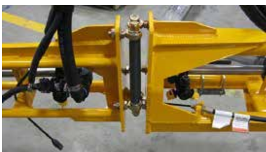
Outer Breakaway -Typical View
