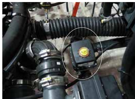
Agitation Valve (Located near center of machine) -Typical View
