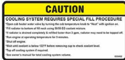
650462 (Located near radiator cap)
