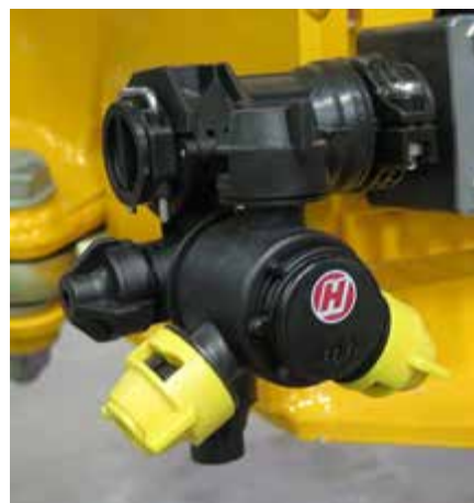
Nozzle Body (Located throughout boom) -Typical View
