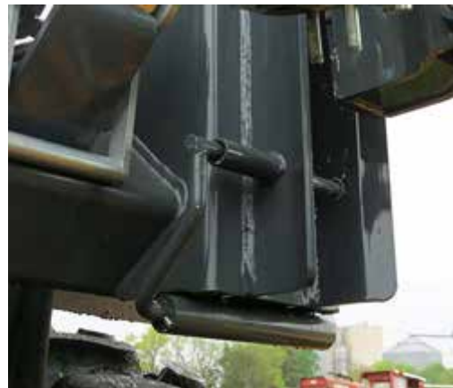
Lock Pin -Typical View * Engaged position shown
