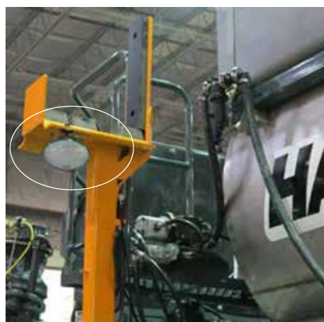
Work Lights (Located on each boom cradle) -Typical View
