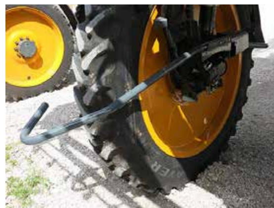
Installed Crop Divider -Typical View
