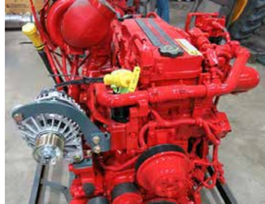
Tier 4 Final Diesel Engine (Located near rear of machine - open hood to access) -Typical View
