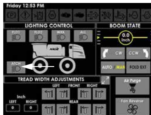
Attachment Lights Button (Located on the Auxiliary Controls Page)
