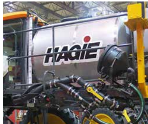
Solution Tank -Typical View
