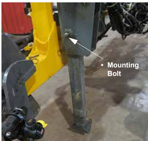
Boom Stand (Extended position shown) -Typical View
