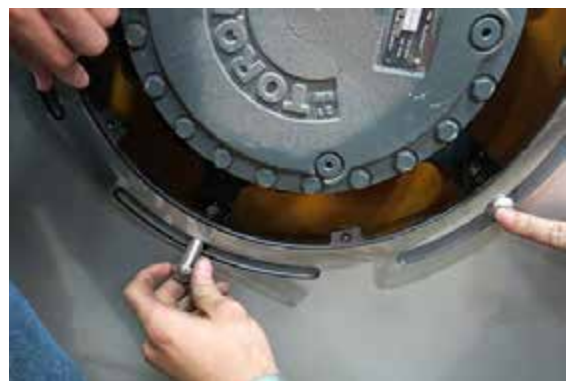
Wheel Cover Mounting Bolt Installation -Typical View
