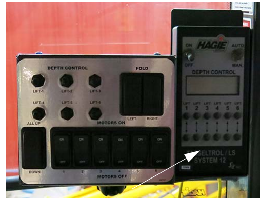
Tasselrol Control Panel -Typical View
