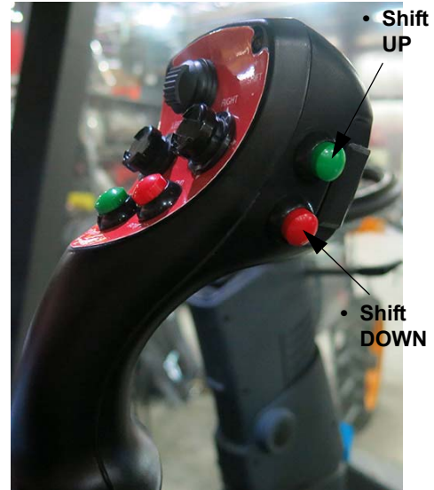
Shift Up/Down Switches (Located on the side of the Hydrostatic Drive Control Handle - Version 2) -Typical View
