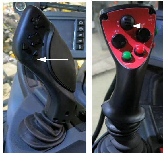
Transom Switch - DOWN (Located on the Hydrostatic Drive Control Handle) -Typical View
