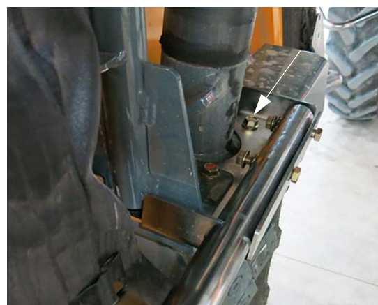
Mounting Plate Bolt -Typical View
