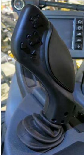
Hydrostatic Drive Control Handle (Version 1) -Typical View
