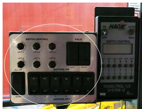
Detasseling Control Panel -Typical View
