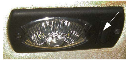
Interior Work Light Switch -Typical View
