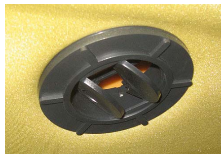
Cab Vent -Typical View
