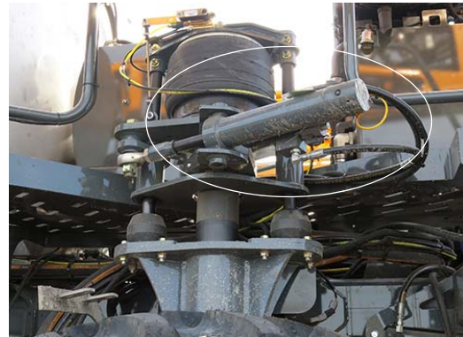
Steering Cylinder (Located on the rear legs) -Typical View
