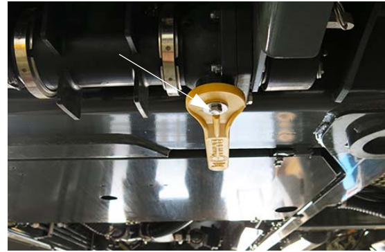
Front Fill Valve Bolt -Typical View
