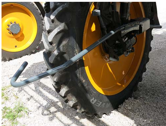
Installed Crop Divider -Typical View
