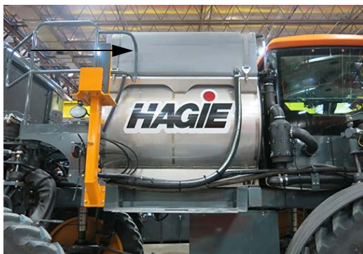
Rinse Tank -Typical View
