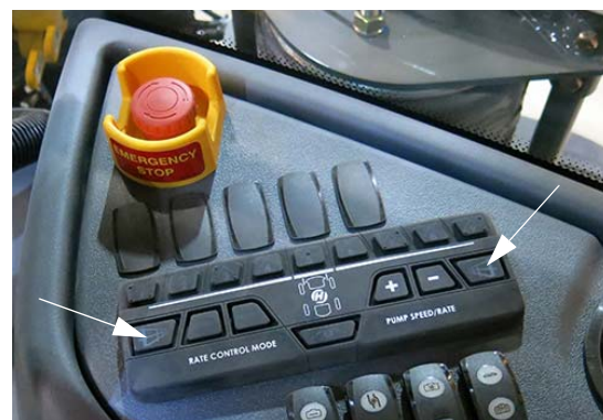
Fence Row Switches (Located on the side console) -Typical View
