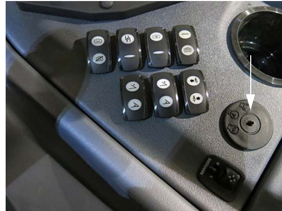
Ignition Switch (Located on the side console) -Typical View
