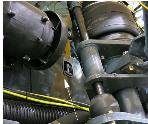
Exterior Service Panel (Located on right-hand side of cab) -Typical View
