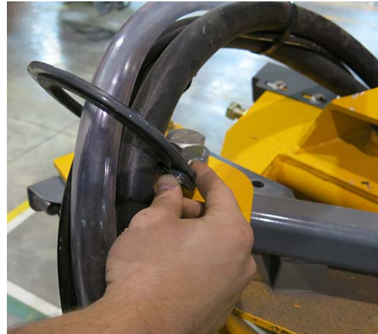
Boom Hose Clamp -Typical View
