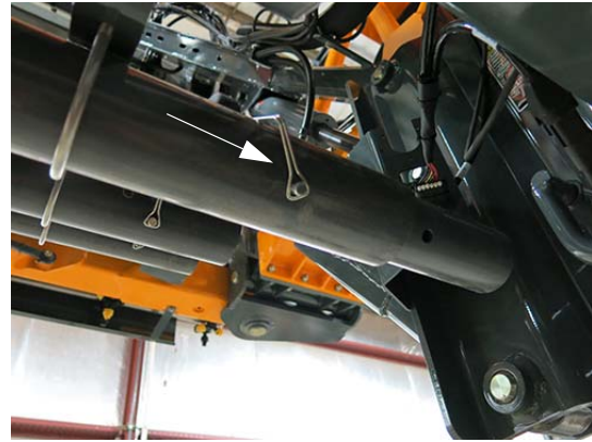
Brush Guard Adjustment Clip (Located on the end of each tube) -Typical View
