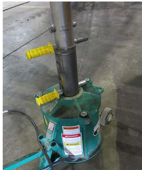
Lock Pin Installation -Typical View
