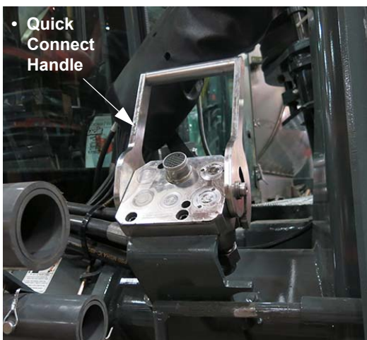
Hydraulic/Electric Multi-Coupler Assembly - If Equipped (Located on the front left-hand side of machine)
