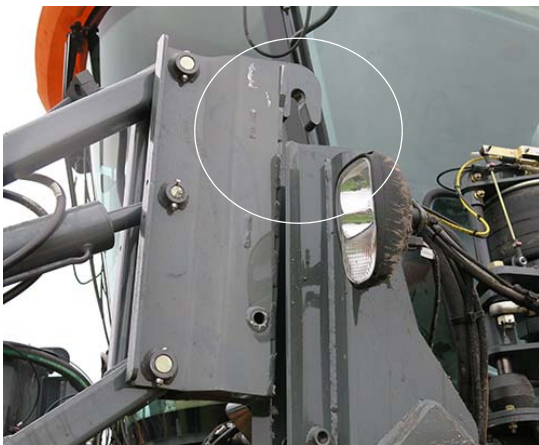
Attachment Clearing Mounting Pin -Typical View
