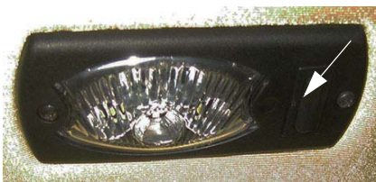
Interior Work Light Switch -Typical View
