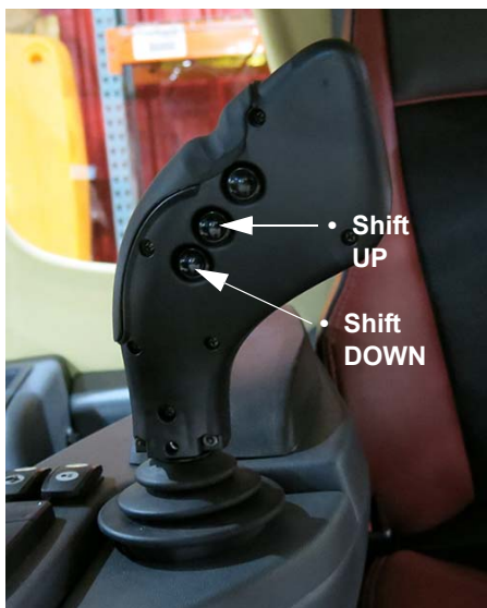
Shift Up/Down Switches (Located on the back side of the Hydrostatic Drive Control Handle - Version 1) -Typical View
