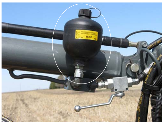
Accumulator -Typical View
