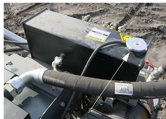
Radiator Cap (Located in the engine compartment) -Typical View
