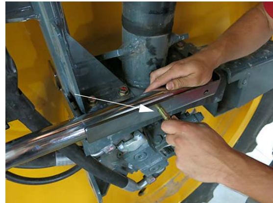
Crop Divider Mounting Bolt -Typical View
