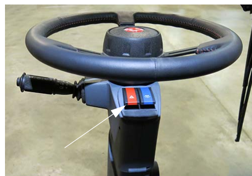
Hazard/Warning Lights Switch (Located on steering column)
