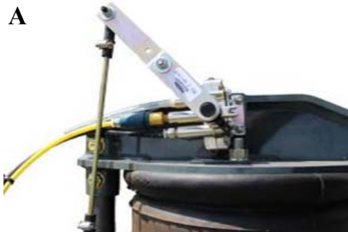
A Dump Valve (One valve located on each leg) -Typical View
