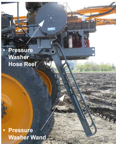
Pressure Washer Wand/ Hose Reel Assembly (Located near ladder on left-hand side of machine) -Typical View
