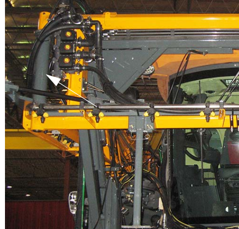
Transom Pivot Tube -Typical View
