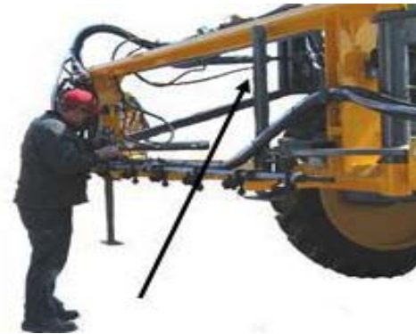
Boom Stand in "Travel" Position -Typical View
