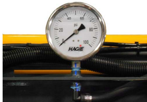
Pressure Gauge -Typical View
