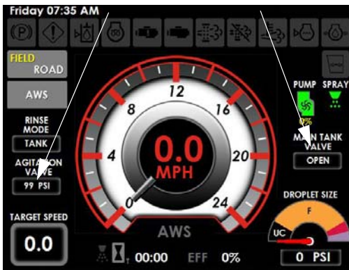
Main Tank Valve Status and Agitation Valve Pressure Indicators (Located on the Machine Display Home Page - Field Mode)
