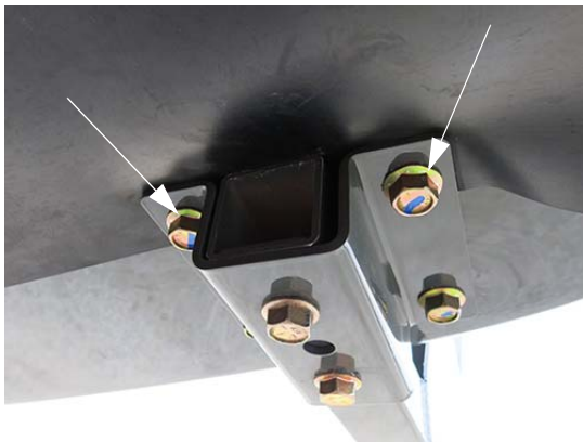
Mounting Bolts (Two located on each side of hood bracket) -Typical View
