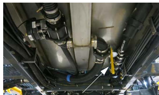
Sump Valve (Located beneath solution tank on right-hand side of machine) -Typical View
