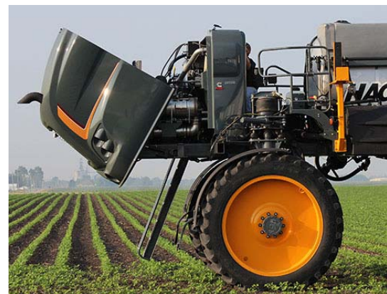
Rear Hood (Open position shown) -Typical View
