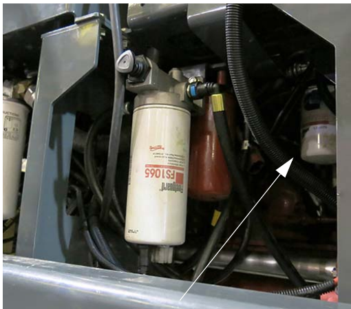
Engine Oil Filter (Located along left-hand side of machine) -Typical View
