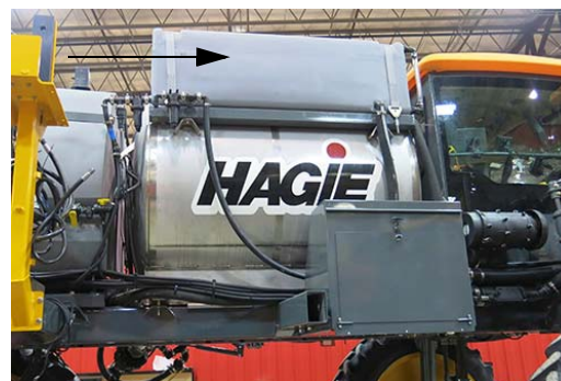
Rinse Tank -Typical View
