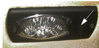
Interior Work Light Switch -Typical View
