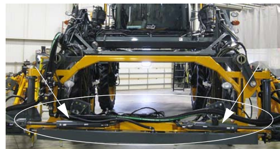
Main Pivot/Breakaway Cylinders -Typical View
