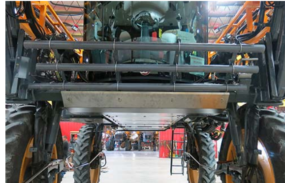
Brush Guard Installation -Typical View
