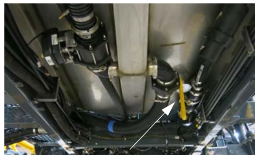
Sump Valve -Typical View
