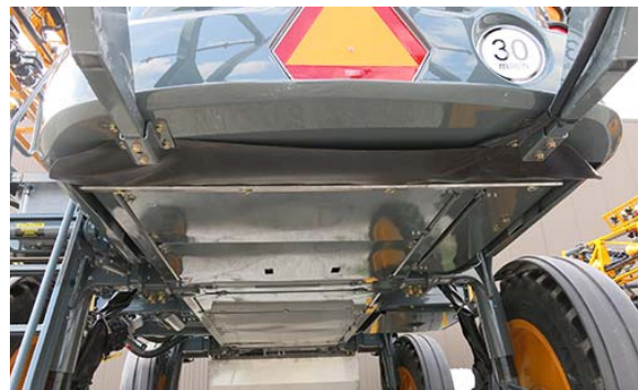
Belly Shield/Brush Curtain Installation -Typical View
