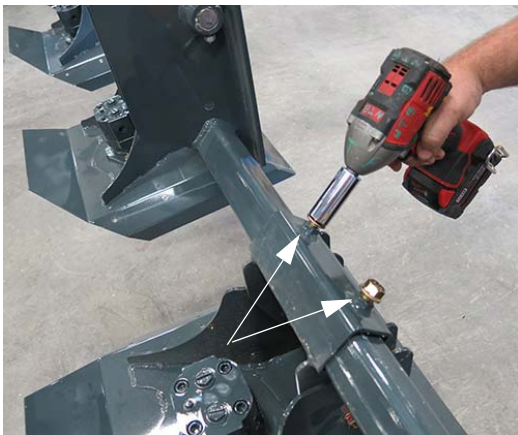
Cutter Head Bolts (Located on each Cutter Head Mounting Tube) -Typical View
