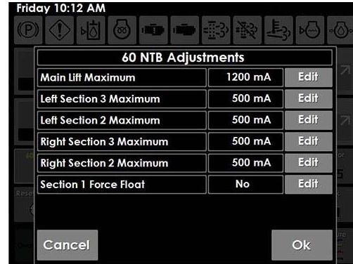
60' NTB Adjustments Screen -Typical View
