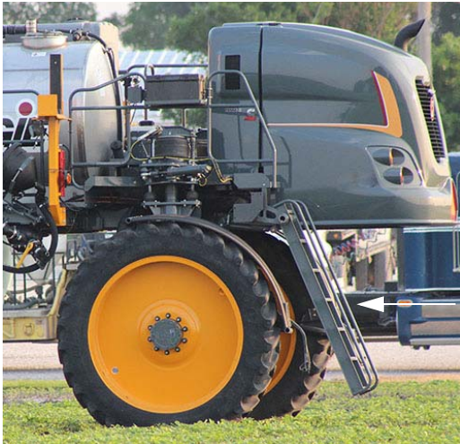
Ladder -Typical View * Lowered position shown
