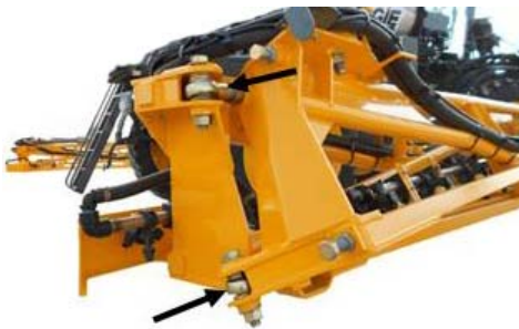
Boom Fold Linkages -Typical View
