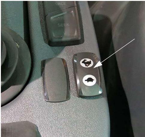
Throttle Switch (Located near the Hydrostatic Drive Control Handle) -Typical View
