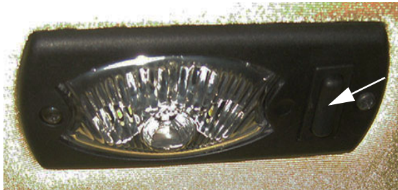
Interior Work Light Switch -Typical View
