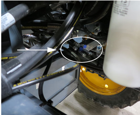
A/C Charge Ports (Located on rear right-hand side of machine - open hood to access) -Typical View
