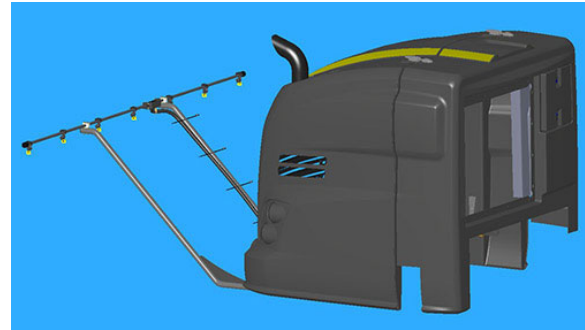
Rear Boom Installation -Typical View
