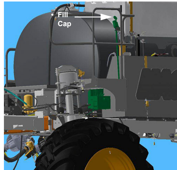
Foam Marker Reservoir Fill (Located on the rear right-hand handrail) -Typical View
