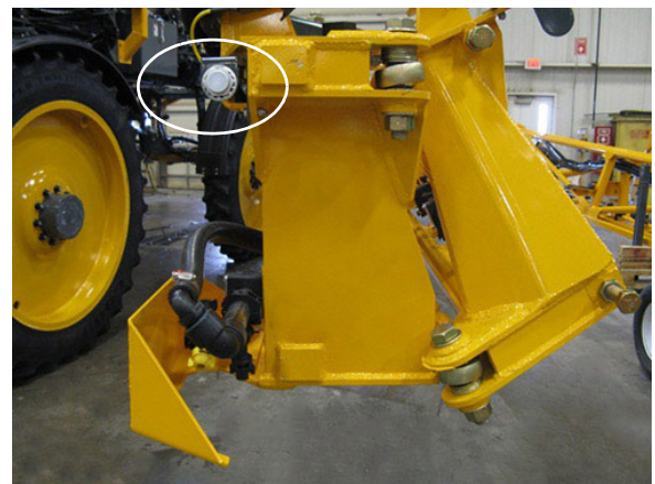
Proximity Sensors -Typical View
