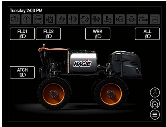
Exterior Lighting Screen
