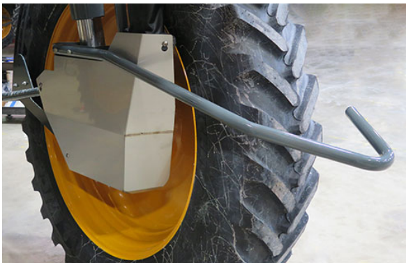
Installed Crop Divider -Typical View
