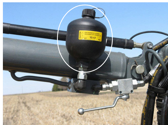
Accumulator -Typical View
