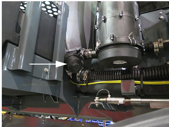
Solution Line Strainer - Secondary (Located near the front right-hand side of machine) -Typical View
