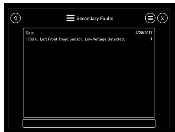
Secondary Faults Screen
