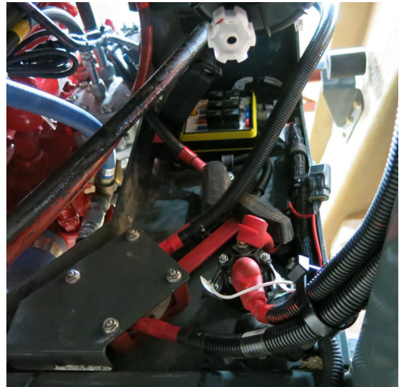
Final Tier 4 Engine Fuse/Relay Block (Located beneath batteries on the rear left-hand side of machine) -Typical View
