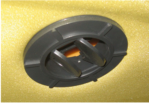
Cab Vent -Typical View
