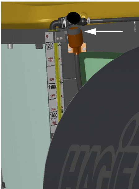
Windshield Washer Fluid Reservoir (Located behind the left-hand side of cab) -Typical View
