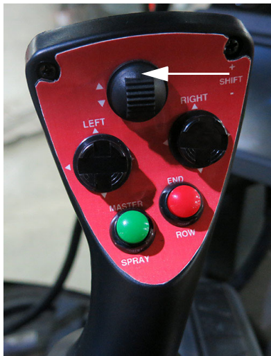
Transom Switch - UP (Located on the Hydrostatic Drive Control Handle) -Typical View
