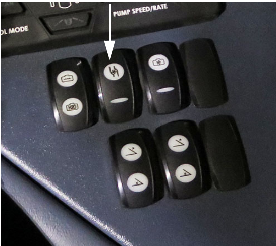
Solution Pump Switch (Located on the side console) -Typical View
