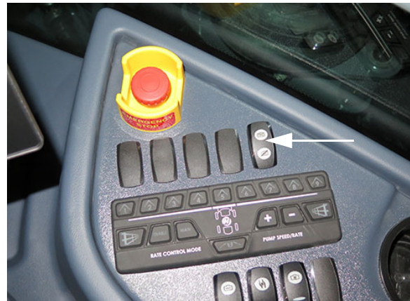
Tank Rinse Switch (Located on the side console) -Typical View
