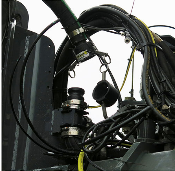
Solution Connection - Standard (Located on the front right-hand side of machine) -Typical View
