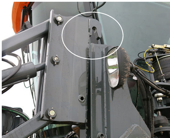
Attachment Clearing Mounting Pin -Typical View
