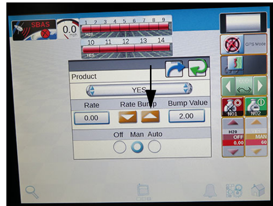
Rate Bump Button (Located on the spray system console) -Typical View
