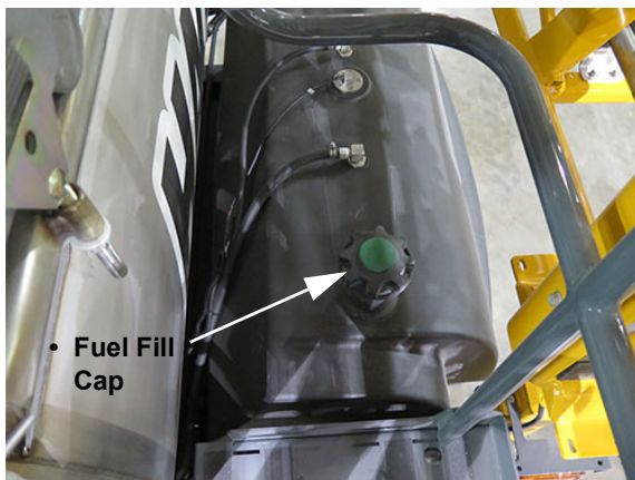
Engine Fuel Fill (Located on top of fuel tank on right-hand side of machine) -Typical View
