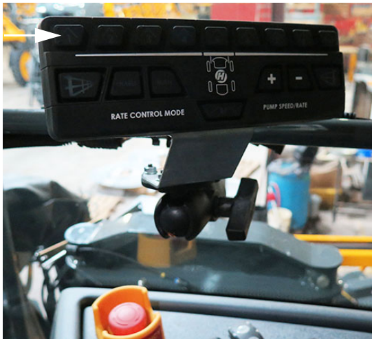
Boom Solution Valve Switches - Dual Product Section Keypad (Mounted near the side console) -Typical View
