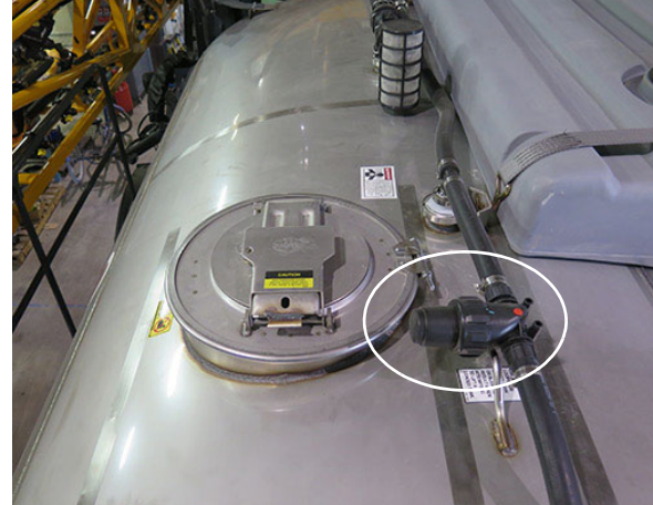
Tank Rinse Strainer - Stainless Steel Tank (Located on top of solution tank) -Typical View
