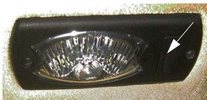
Interior Work Light Switch -Typical View
