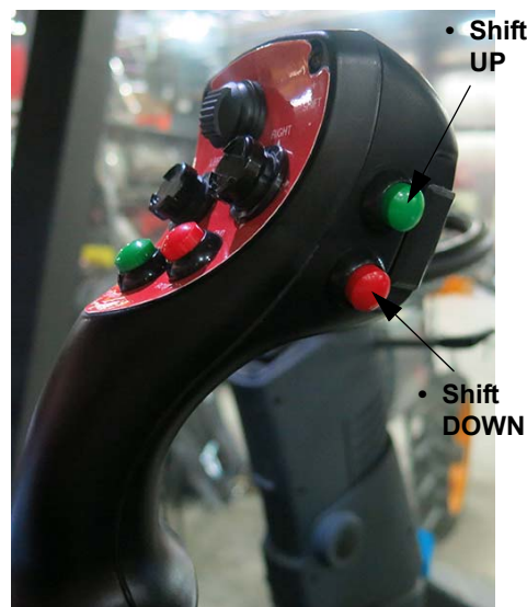
Shift Up/Down Switches (Located on the side of the Hydrostatic Drive Control Handle - Version 2) -Typical View
