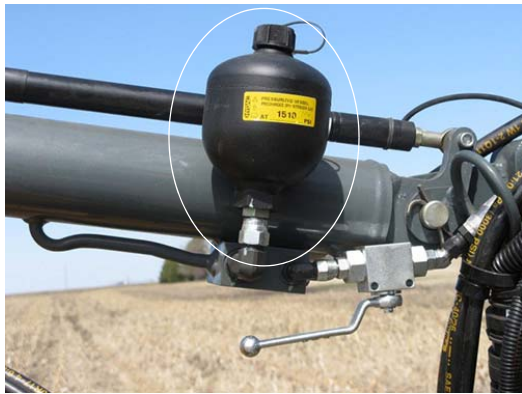
Accumulator -Typical View
