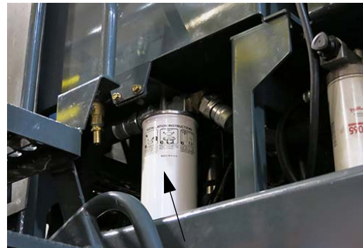
Case Drain Filter (Located on left-hand side of machine) -Typical View
