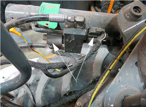
Lock Valves -Typical View
