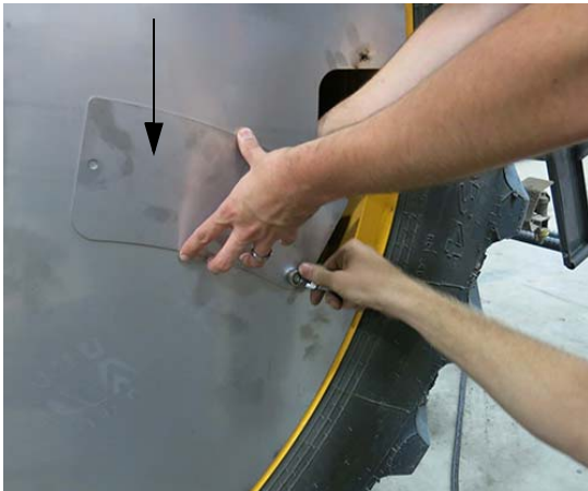
Valve Stem Access Panel -Typical View
