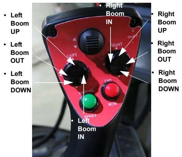
Left and Right-Hand Boom Switches (Located on the Hydrostatic Drive Control Handle - Version 2) -Typical View
