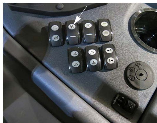
Solution Pump Switch (Located on the side console) -Typical View
