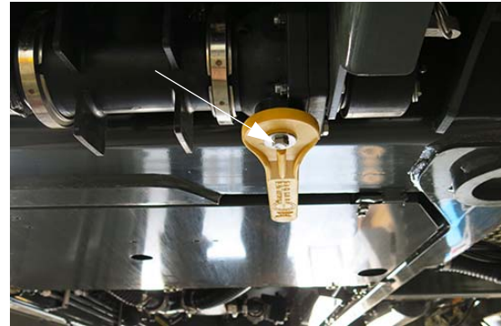
Front Fill Valve Bolt -Typical View
