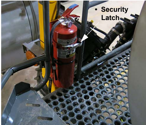
Fire Extinguisher (Located along the platform on left-hand side of machine) -Typical View
