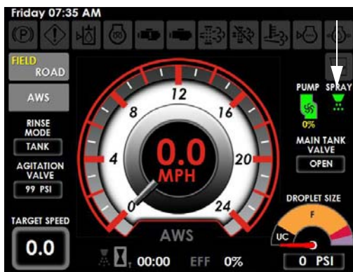
Master Spray Indicator (Located on the Machine Display Home Page - Field Mode)
