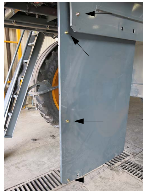
Hanger Pins (Install three pins onto Panel 4 and one pin onto Panel 5, as shown) -Typical View
