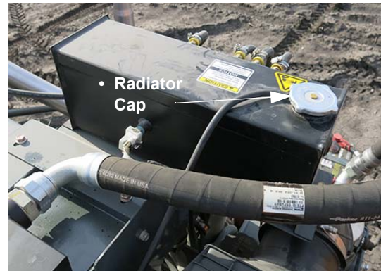
Radiator (Located near the rear of machine - open hood to access) -Typical View
