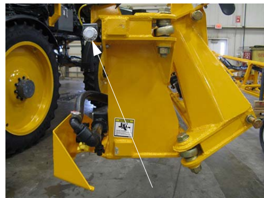
Proximity Sensors -Typical View
