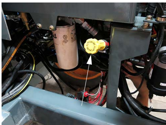
Remote Engine Oil Fill (Located on rear left-hand side of machine - open hood to access) -Typical View
