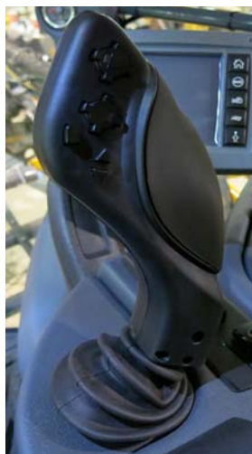
Hydrostatic Drive Control Handle -Typical View
