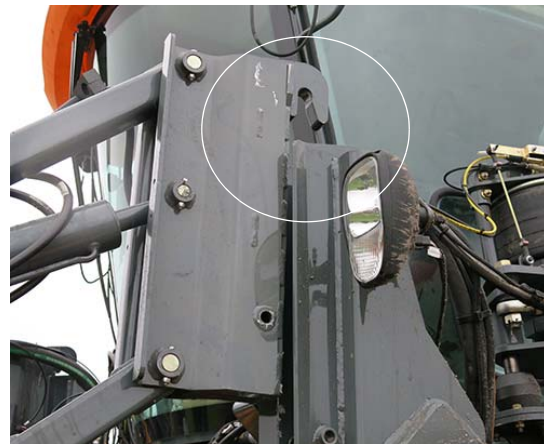
Attachment Clearing Mounting Pin -Typical View
