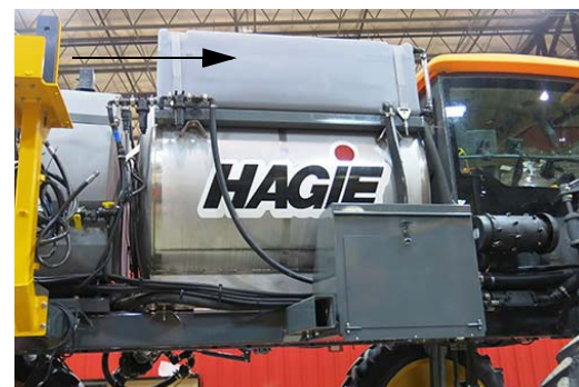
Rinse Tank -Typical View
