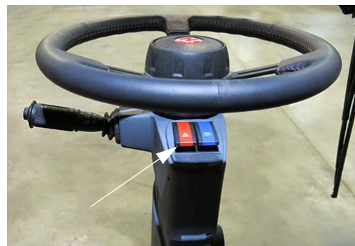
Hazard/Warning Lights Switch (Located on steering column)
