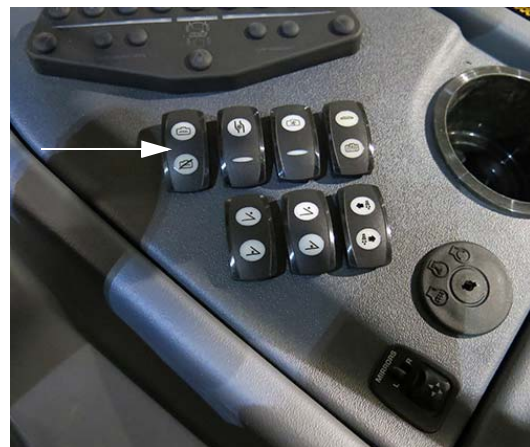
Main Tank Valve Switch (Located on the side console) -Typical View
