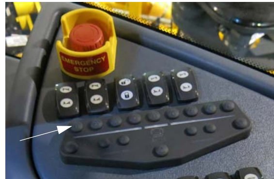
Boom Solution Valve Switches (Located on the side console) -Typical View
