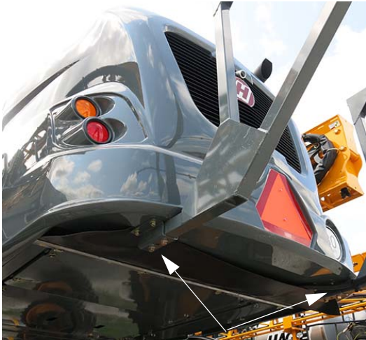
Brush Curtain Attached to Hood -Typical View
