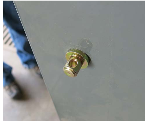
Hanger Pin Installation -Typical View
