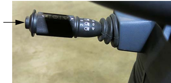
Horn Button (Located on the end of the Turn Signal Lever) -Typical View
