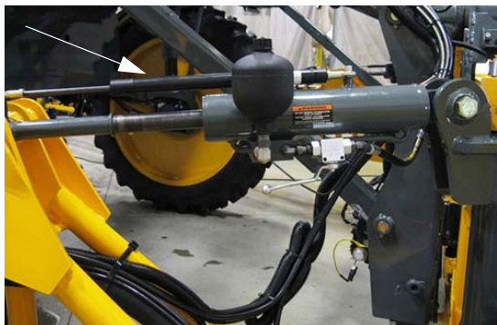
Position Sensor -Typical View
