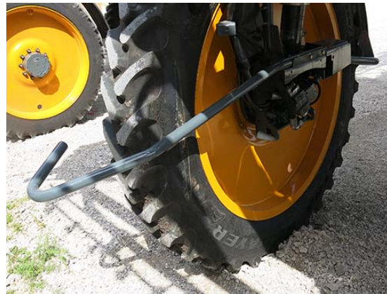
Installed Crop Divider -Typical View
