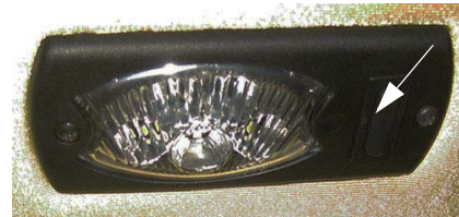
Interior Work Light Switch -Typical View
