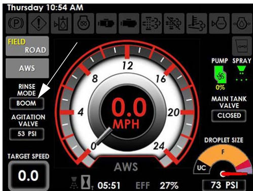
Rinse Mode Indicator (Located on the Machine Display Home Page - Field Mode)
