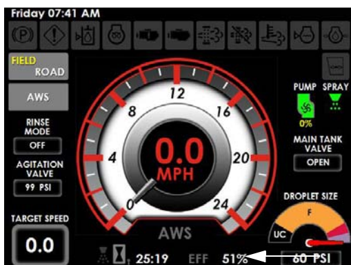
Efficiency (EFF) Rate (Located on the Home Page - Field Mode)
