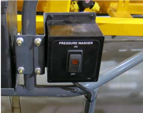
Pressure Washer Switch (Located along the handrail on left-hand side of machine) -Typical View
