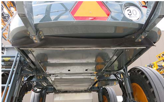
Belly Shield/Brush Curtain Installation -Typical View
