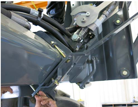
Anchor Bolt Assembly -Typical View
