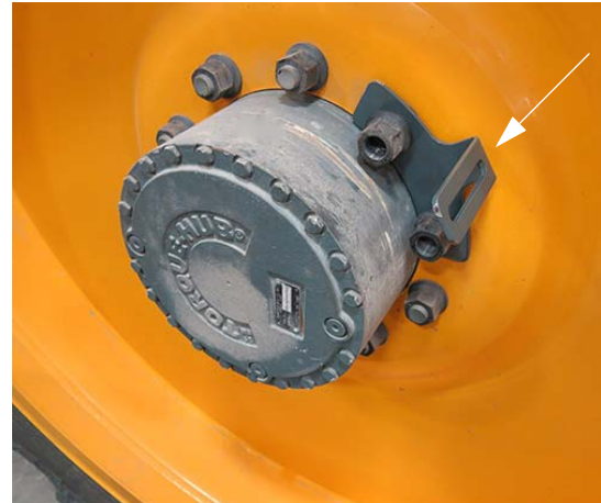
Hub Cap Adapter Plate -Typical View
