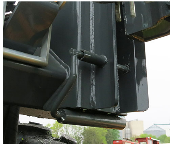
Lock Pin (2) -Typical View * Engaged position shown
