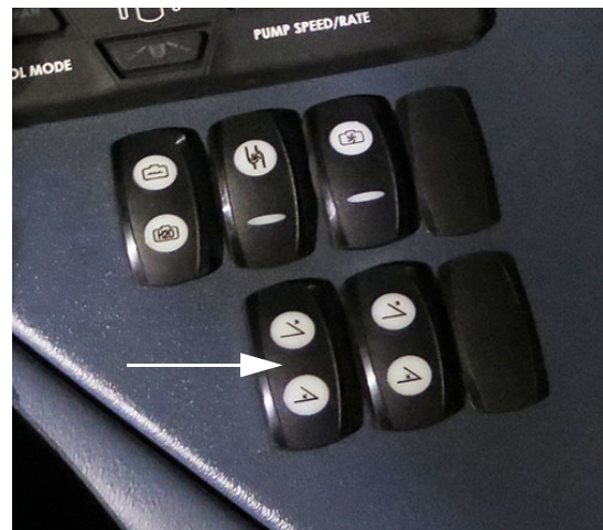
Boom/NTB Extension Switch (Located on the side console) -Typical View
