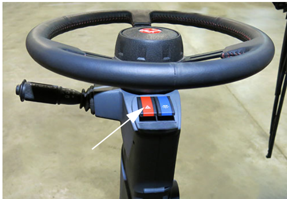
Hazard/Warning Lights Switch (Located on the steering column) -Typical View
