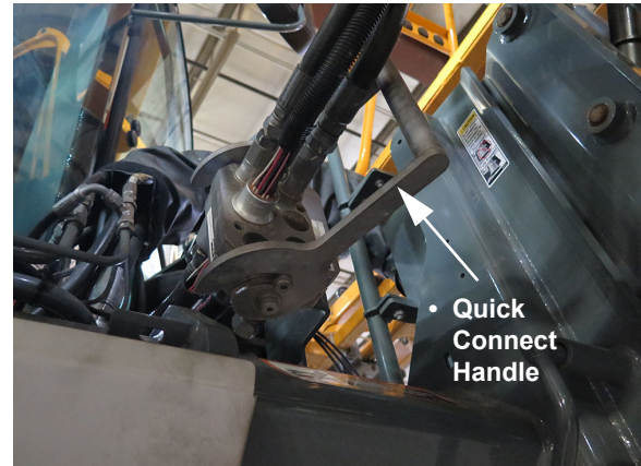
Hydraulic/Electric Multi-Coupler Assembly (Located on the front left-hand side of machine)
