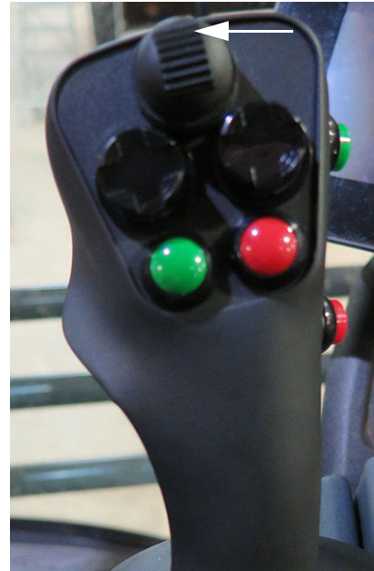
Transom Switch - UP (Located on the Hydrostatic Drive Control Handle) -Typical View
