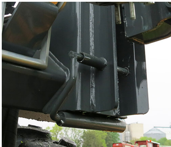
Lock Pin (2) -Typical View * Engaged position shown
