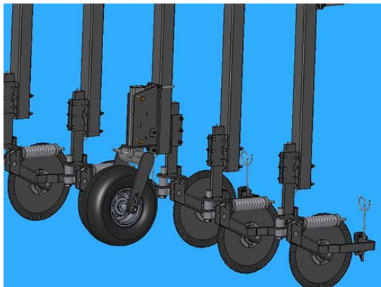
Gauge Wheel (Field position shown) -Typical View
