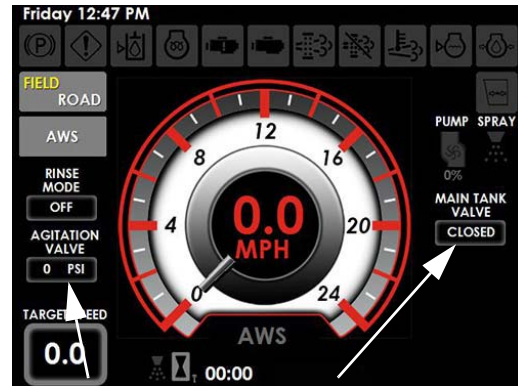
• Agitation Valve Pressure • Main Tank Valve Status
