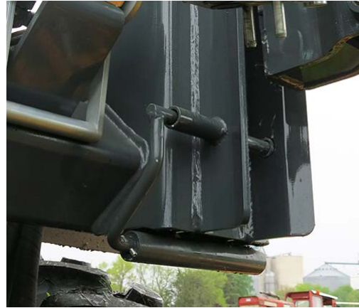
Lock Pin -Typical View * Engaged position shown
