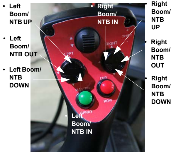
Left and Right Boom/NTB Switches (Located on the Hydrostatic Drive Control Handle) -Typical View
