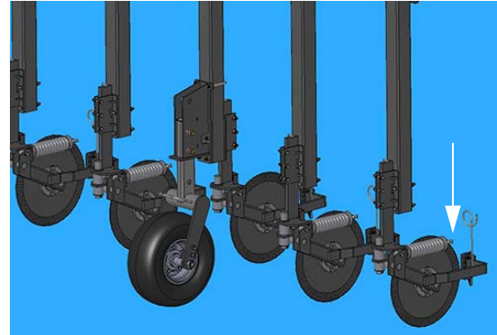
Adjustment Nut (Located on the end of each couler spring) -Typical View
