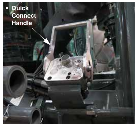
Hydraulic/Electric Multi-Coupler Assembly (Located on the front left-hand side of machine) -Typical View
