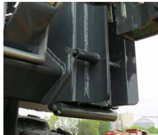
Lock Pin -Typical View * Engaged position shown
