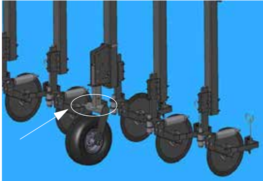
Lift Handle (Located above gauge wheel) -Typical View
