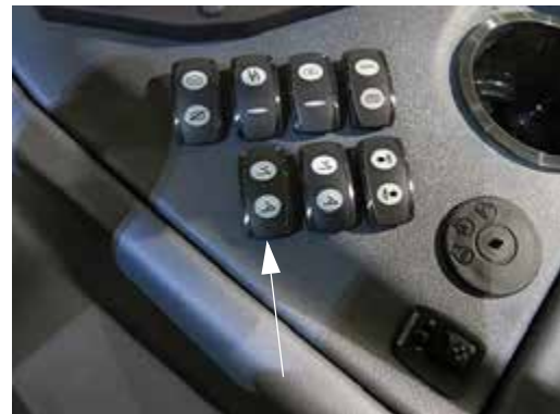
Boom/NTB Extension Switch (Located on the side console) -Typical View
