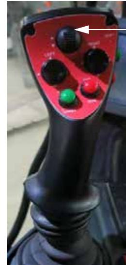
Transom Switch - UP (Located on the Hydrostatic Drive Control Handle - Version 2) -Typical View
