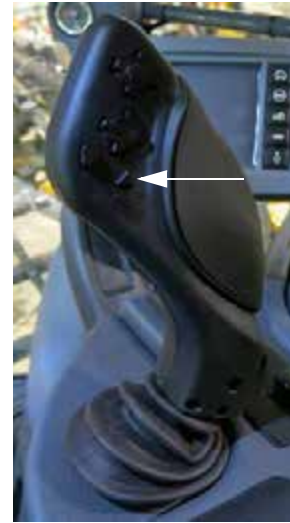
Transom Switch - UP (Located on the Hydrostatic Drive Control Handle - Version 1) -Typical View
