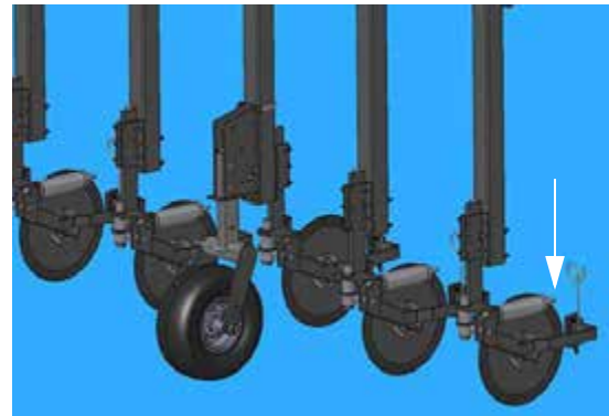
Adjustment Nut (Located on the end of each coulters spring) -Typical View
