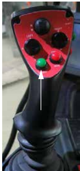
Master Spray Switch (Located on the Hydrostatic Drive Control Handle - Version 2) -Typical View
