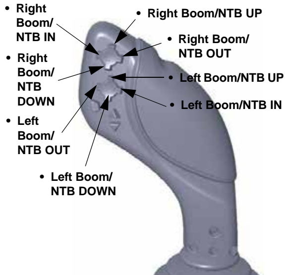
Left and Right Boom/NTB Switches (Located on the Hydrostatic Drive Control Handle - Version 1) -Typical View
