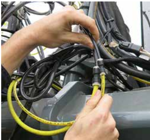
Foam Marker Connection (Located on front right-hand side of machine) -Typical View
