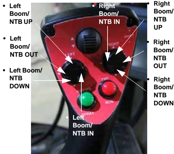
Left and Right Boom/NTB Switches (Located on the Hydrostatic Drive Control Handle - Version 2) -Typical View
