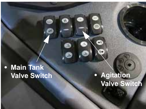
Main Tank and Agitation Valve Switches (Located on the side console) -Typical View
