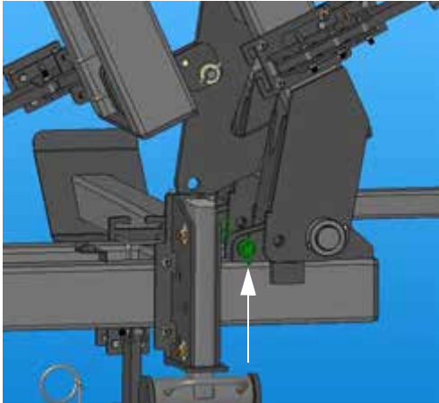
Main Fold Lock Pin (Located on the front side of toolbar near the main fold point - "Field/Unlocked Position" shown) -Typical View
