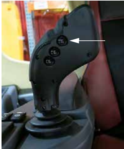
Master Spray Switch (Located on the back side of the Hydrostatic Drive Control Handle - Version 1) -Typical View
