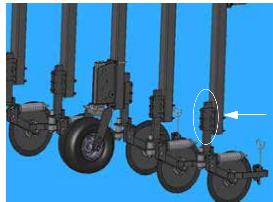
Mounting Bolts (Located on the side of the coulters mounting plate) -Typical View
