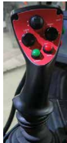
Hydrostatic Drive Control Handle (Version 2) -Typical View
