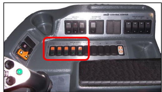
Figure 12: Spray section switches
