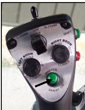
Figure 11: Master spray switch
