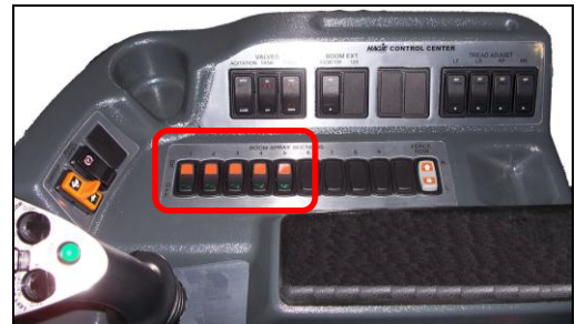
Figure 10: Spray section switches
