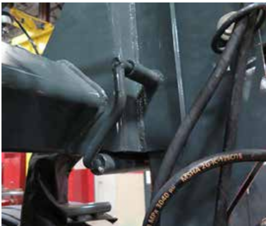
Lock Pin -Typical View Engaged position shown
