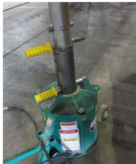
Lock Pin Installation -Typical View
