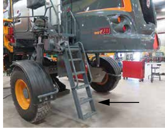
Ladder -Typical View * Lowered position shown
