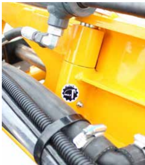
Boom Breakaway -Typical View
