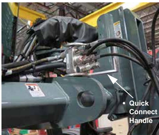
Hydraulic/Electrical Connections (Located on front left-hand side of machine) -Typical View
