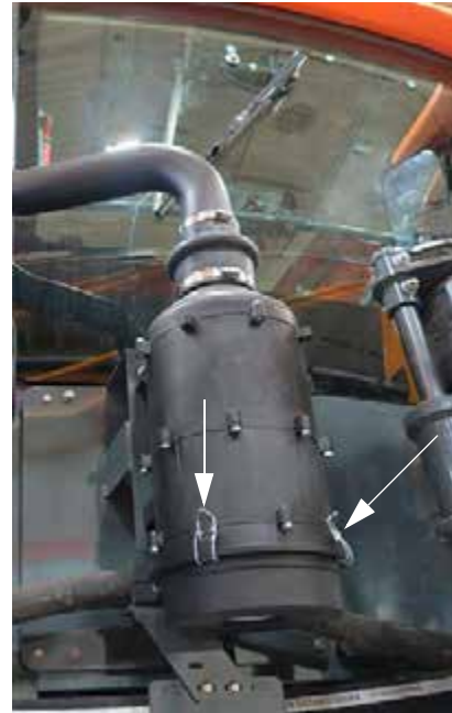
Filter Latches -Typical View
