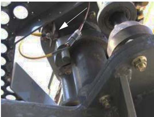
External Proximity Sensor -Typical View
