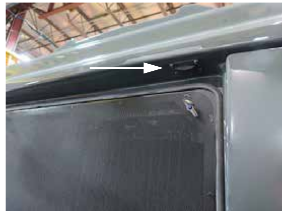
Hood Actuator Switch (Located ahead of rear hood above the radiator screen) -Typical View
