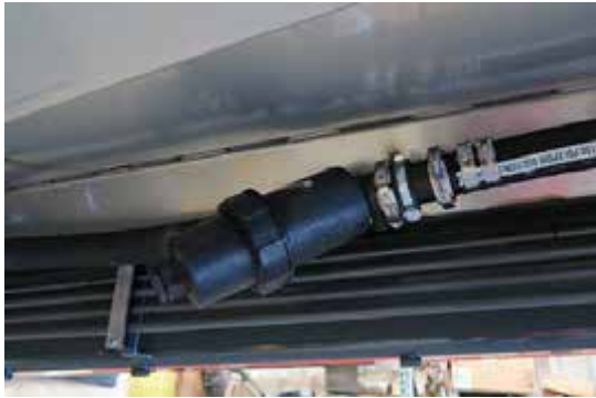
Solution Line Strainer (Located beneath the center right-hand side of machine) -Typical View
