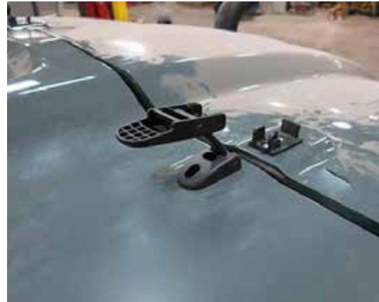
Hood Latch (2) (Located on each side of top hood) -Typical View
