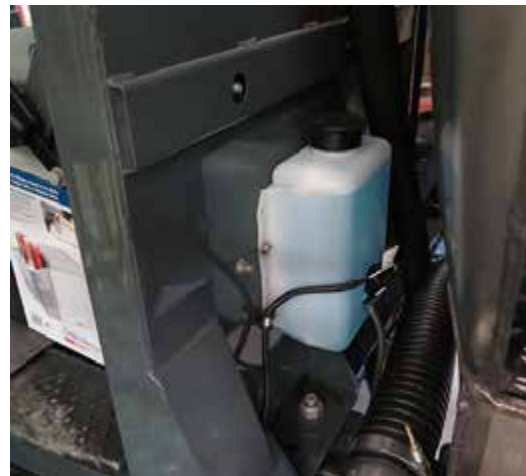
Windshield Washer Fluid Reservoir (Located behind the left-hand side of exterior cab) -Typical View
