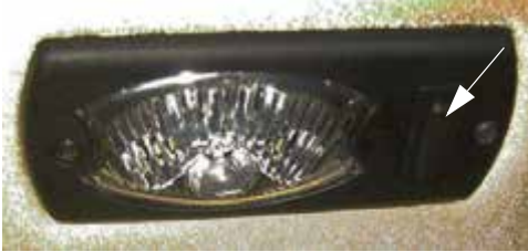
Interior Work Light Switch -Typical View
