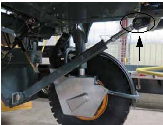
Securement Bolt/Nut Assembly - Upper -Typical View
