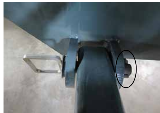
Securement Bolt/Nut Assembly - Lower -Typical View
