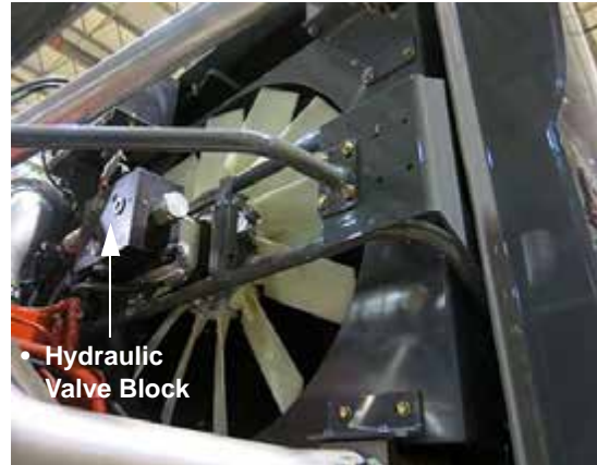
Reversible Fan (Located near the rear of machine - open hood to access) -Typical View
