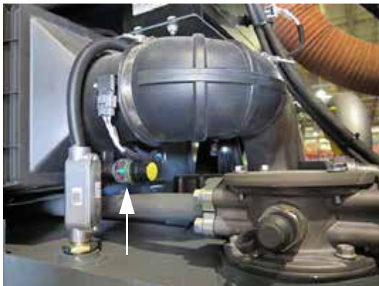
Filter Minder (Located near engine pre-filter - open hood to access) -Typical View
