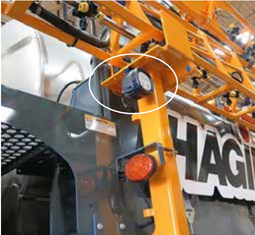
Work Lights (Located on each boom cradle) -Typical View
