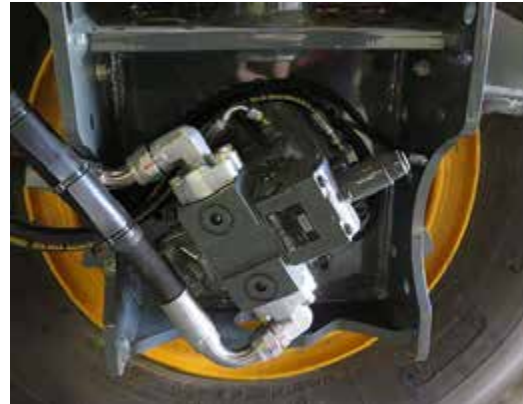
Wheel Motor -Typical View
