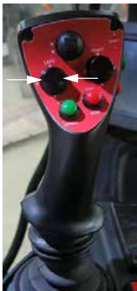
Brush Open/Close Switches (Located on the Hydrostatic Drive Control Handle) -Typical View
