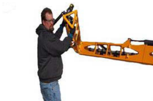
Securement Bolt (Located on the back side of boom) -Typical View
