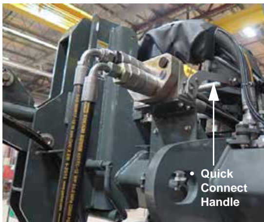
Hydraulic Connection (Located on front right-hand side of machine) -Typical View * Push UP to engage
