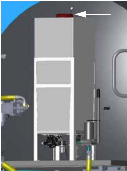
Deluge Fill Cap (Located on top of reservoir) -Typical View
