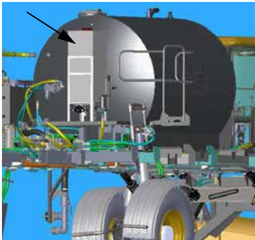
Deluge Solution Reservoir (Located along rear platform behind solution tank) -Typical View
