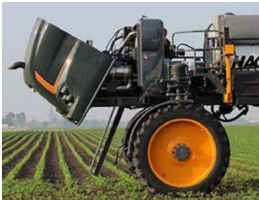
Rear Hood (Open position shown) -Typical View
