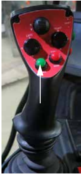
Brush On/Off Switch (Located on the Hydrostatic Drive Control Handle) -Typical View
