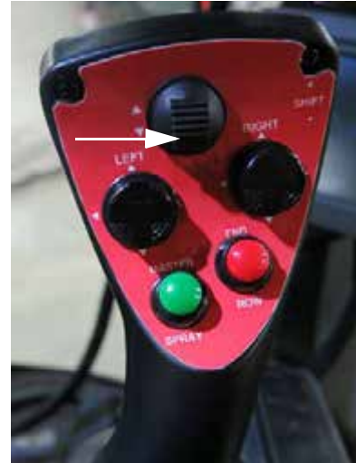
Transom Switch - DOWN (Located on the Hydrostatic Drive Control Handle) -Typical View
