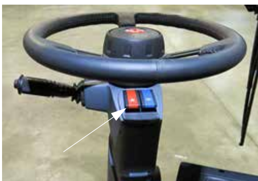
Hazard/Warning Lights Switch (Located on steering column) -Typical View
