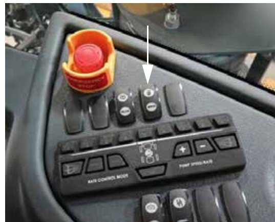
Heated Mirror Switch (Located on the side console) -Typical View
