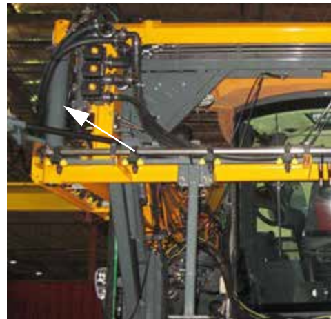
Transom Pivot Tube -Typical View
