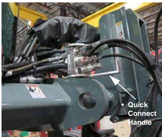
Hydraulic/Electrical Connections (Located on front left-hand side of machine) -Typical View * Push OUT to engage
