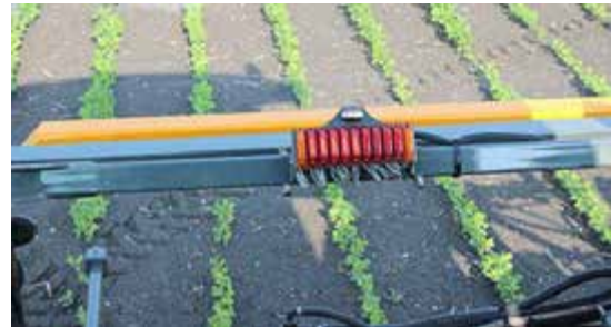
Boom Solution Valve Indicators (Located on transom) -Typical View
