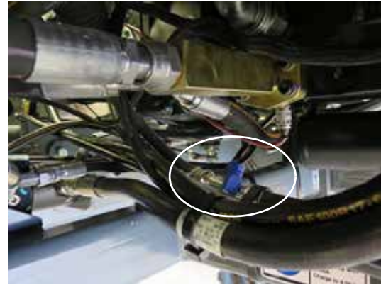
A/C Charge Ports (Located above mainframe on rear left-hand side of machine) -Typical View
