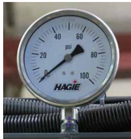
Pressure Gauge (Mounted on boom) -Typical View
