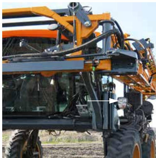
Highway Running Lights (Located on each side of cab) -Typical View
