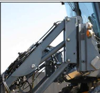
**LOWER THE BOOM TO THE GROUND**– Slowly and gently ease the boom to the ground. \*Airbags may need to be dumped.
