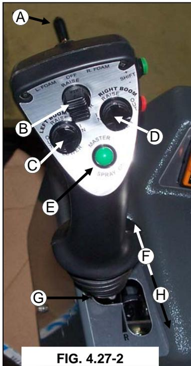
**FORWARD CONTROL-** The hydrostatic lever is responsible for the direction of motion of the machine. To move forward, slowly move the hydrostatic lever forward. (fig. 4.27-2, item F)
