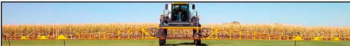
The spraying system is a constantly monitored and continuously adjusted computer controlled system. The cab mounted digital console receives information from various inputs to help determine GPM (gallons per minute) and GPA (gallons per acre).
