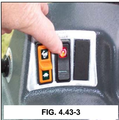
**LADDER-** To raise or lower the ladder you will need to locate the BRAKE/LADDER switch at the front of the right hand console (fig. 4.43-3). When the brake is applied the ladder will lower automatically (fig. 4.43-1). The ladder will not raise (fig. 4.43-2) until the machine is running and the switch has been returned to the OFF position.
