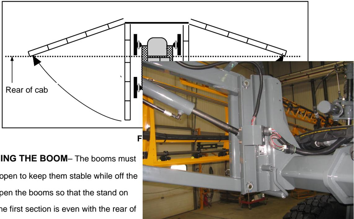
**OPENING THE BOOM**– The booms must be partially open to keep them stable while off the machine. Open the booms so that the stand on the end of the first section is even with the rear of the cab (fig. 4.59-1).
