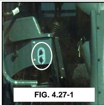
**POWER PORTS-** On the front of the side console there are two power ports (fig. 4.27-1) for extra equipment to be plugged in. They are each protected by a 15 amp fuse. They are not intended for the permanent connection of extra systems to the sprayer. There is a terminal strip intended for the installation of extra radios and computer equipment. See the SERVICE section E on the electrical components. Top port is 12V all the time and bottom port is powered by key.
