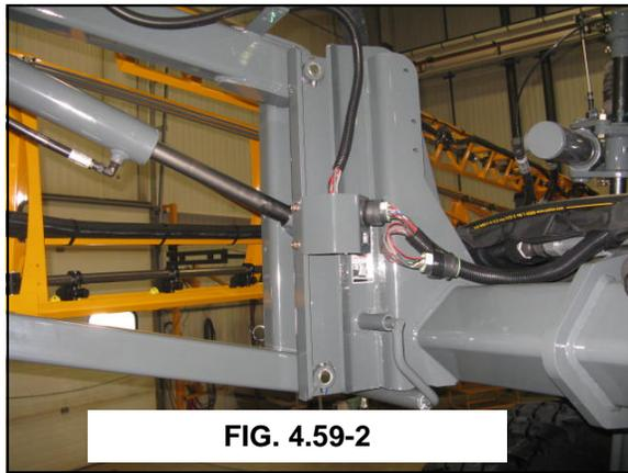
**DISENGAGE THE LOCK ASSEMBLY**– Disengage the lock pin assembly only after you have lowered the boom close to the ground.
