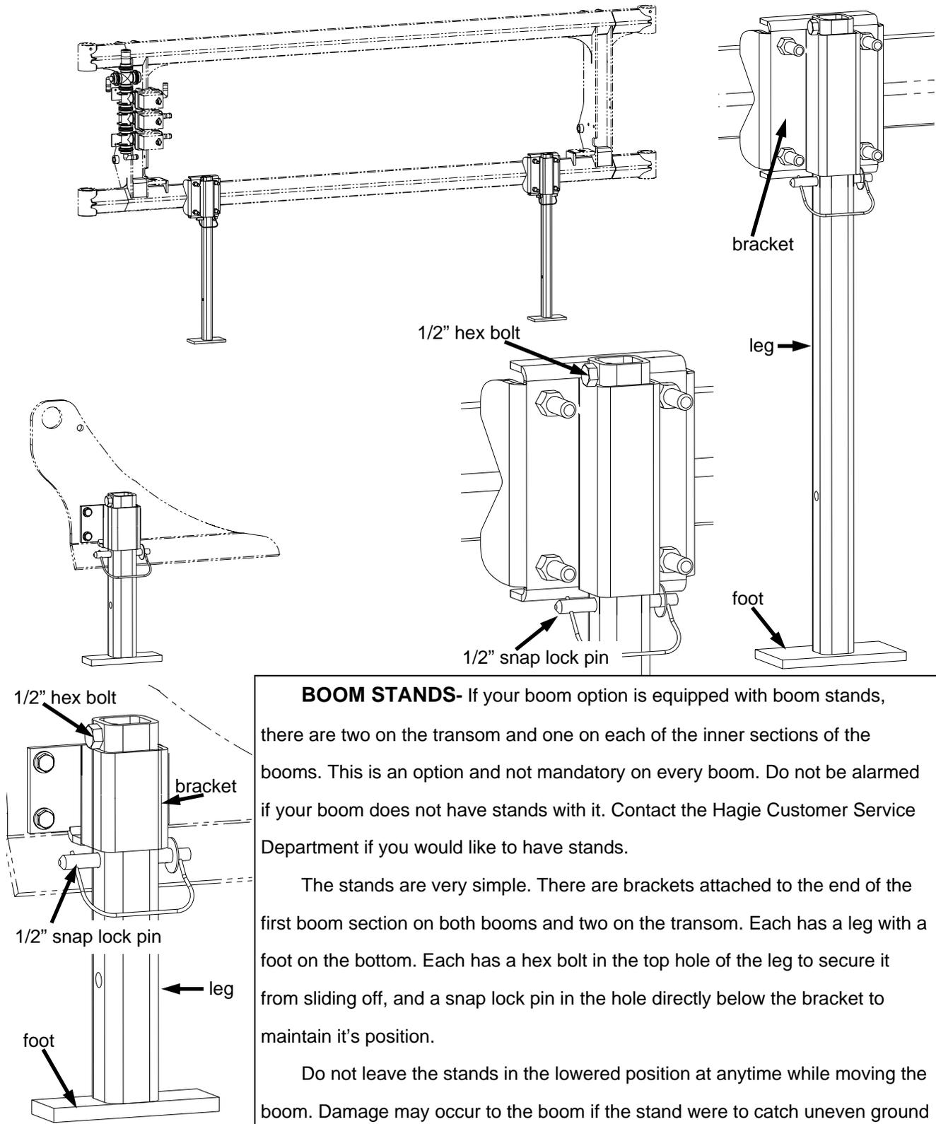
**BOOM STANDS-** If your boom option is equipped with boom stands, there are two on the transom and one on each of the inner sections of the booms. This is an option and not mandatory on every boom. Do not be alarmed if your boom does not have stands with it. Contact the Hagie Customer Service Department if you would like to have stands.
