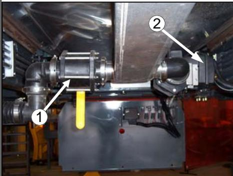
**TANK SUMP VALVE**– The tank sump valve (fig. 4.52-2, item 2) is a ball type valve that has to be turned on and off manually.
