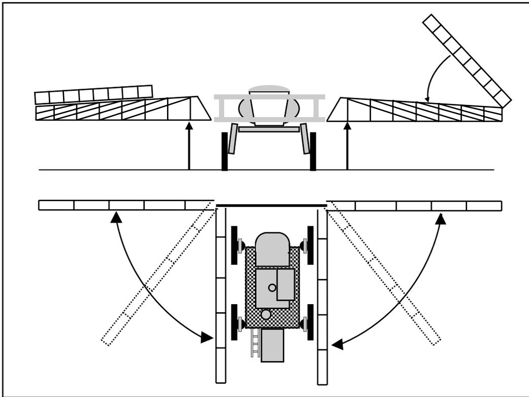
The booms should always be cradled before traveling, transporting, or parking for an extended period of time. **The booms must be folded when cradled.**
