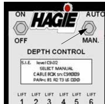
Auto/Manual Switch (Located on the Tasseltrol Control Panel)
