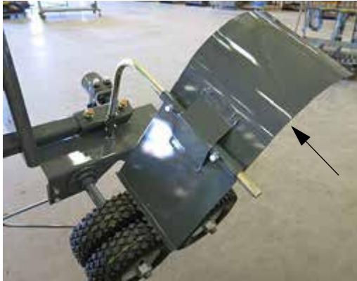
Deflector Shield -Typical View
