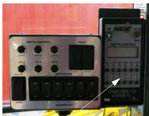
Tasselrol/LS System 12 Control Panel -Typical View
