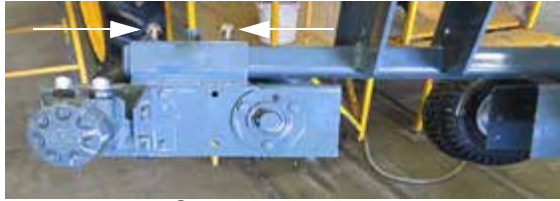
Quad Puller Bolts (Located on each Quad Puller Mounting Tube) -Typical View
