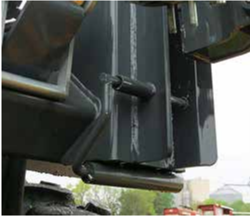
Lock Pin -Typical View * Engaged position shown
