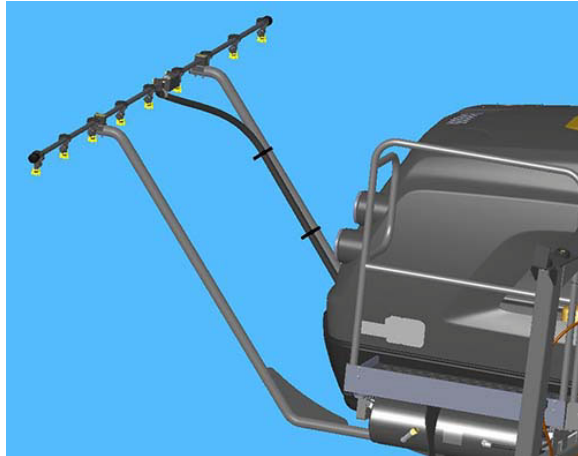
Rear Spray Boom Installation -Typical View
