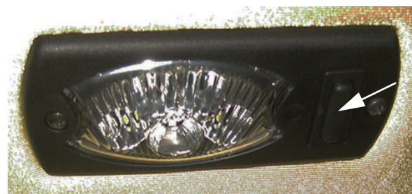
Interior Work Light Switch -Typical View
