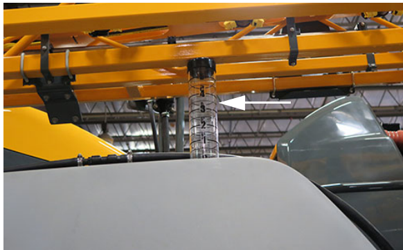
Solution Tank Sight Gauge (2) (Located on top of each solution tank) -Typical View
