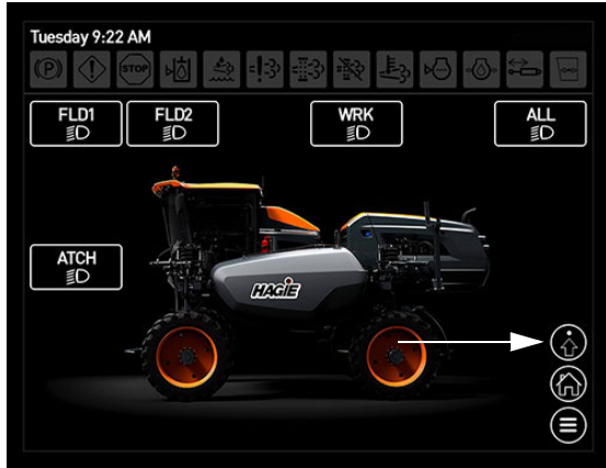
Settings Button (Located on the Exterior Lighting Screen)
