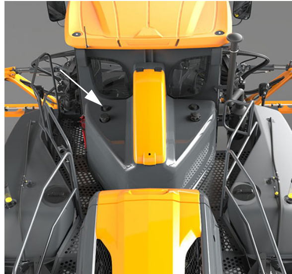
Foam Marker Reservoir Fill (Located on the front left-hand side of fuel-rinse module - “FRM”) -Typical View
