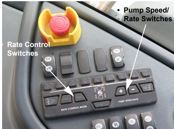
Rate Control and Pump Speed/Rate Switches (Located on the side console) -Typical View
