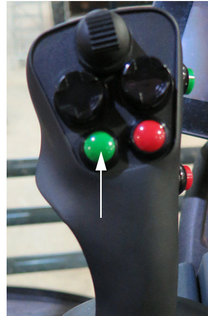
Master Spray Switch (Located on the Hydrostatic Drive Control Handle) -Typical View
