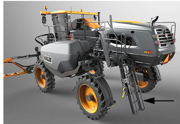
Ladder -Typical View * Lowered position shown
