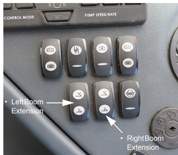
Boom Extension Switches - Left/Right (Located on the side console) -Typical View
