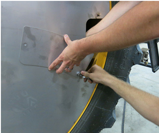
Valve Stem Access Panel -Typical View
