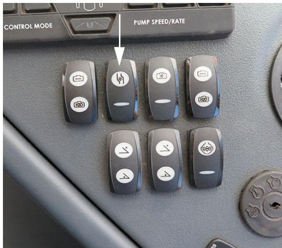
Solution Pump Switch (Located on the side console) -Typical View
