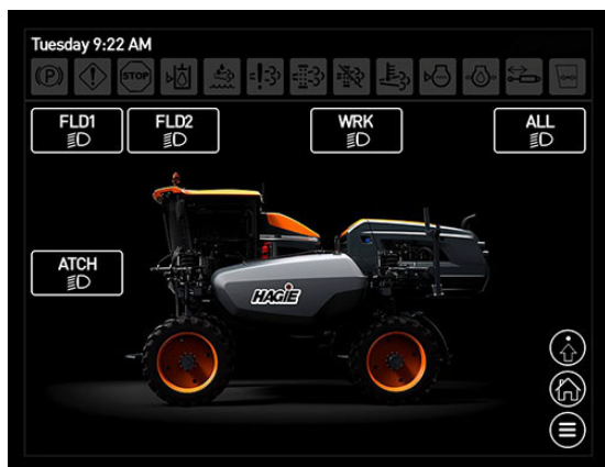
Exterior Lighting Screen
