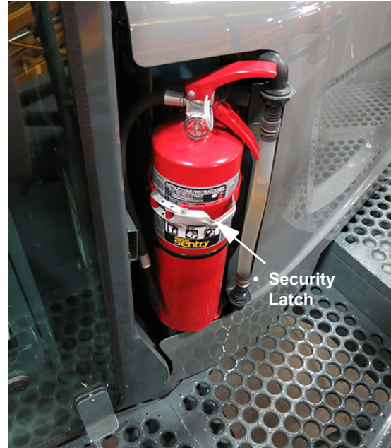
Fire Extinguisher (Located behind left-hand side of cab) -Typical View
