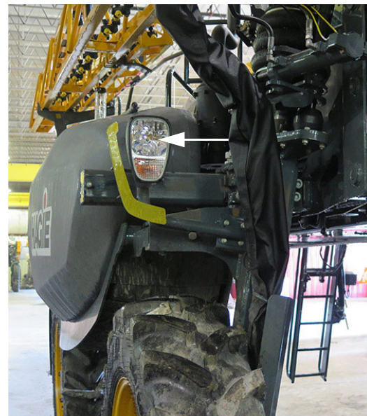
Highway Running Lights (2) -Typical View
