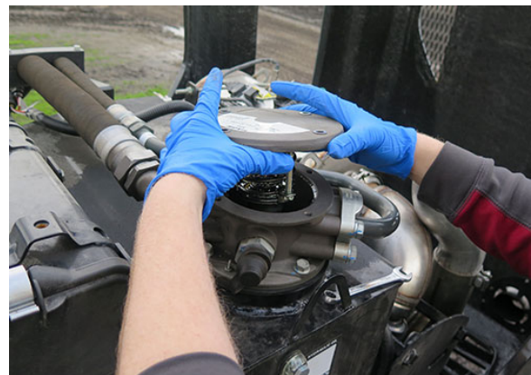
Filling Tank Through Hydraulic Return Filter Housing -Typical View
