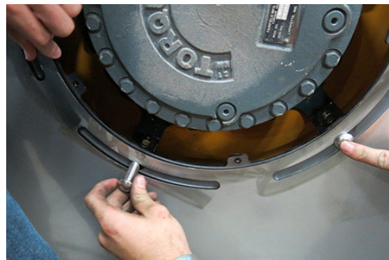
Wheel Cover Mounting Bolt Installation -Typical View
