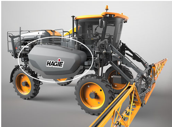
Solution Tank -Typical View
