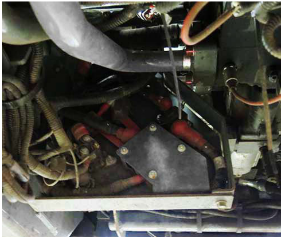
Final Tier 4 Engine Fuse/Relay Block (Located beneath batteries on the rear right-hand side of machine) -Typical View
