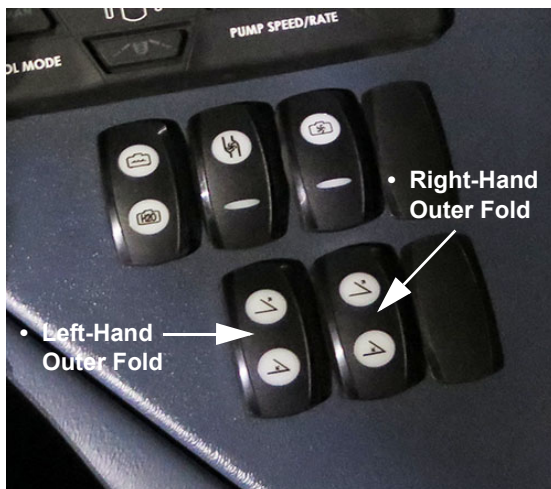
Boom Extension Switches - Left/Right (Located on the side console) -Typical View
