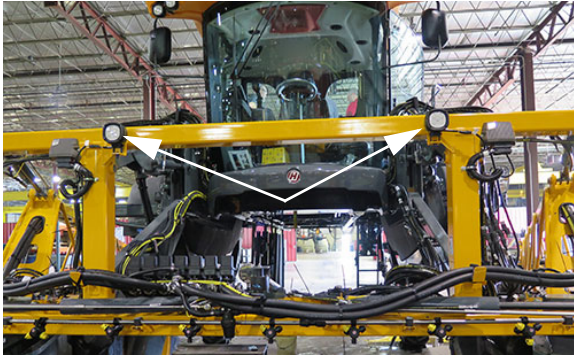
Attachment Lights (Located on the front of transom) -Typical View
