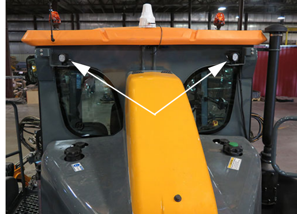
Platform Lights (2) (Located on the rear of cab) -Typical View
