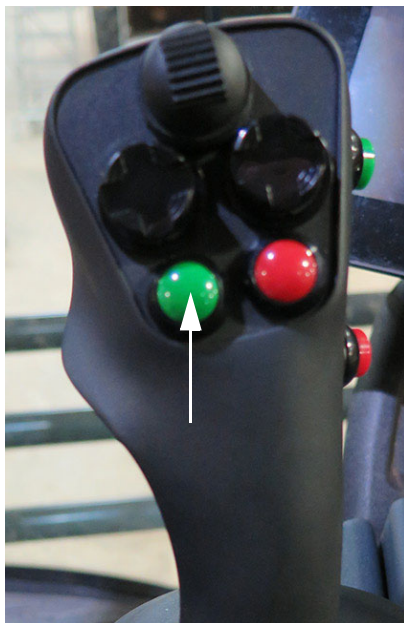
Master Spray Switch (Located on the Hydrostatic Drive Control Handle) -Typical View
