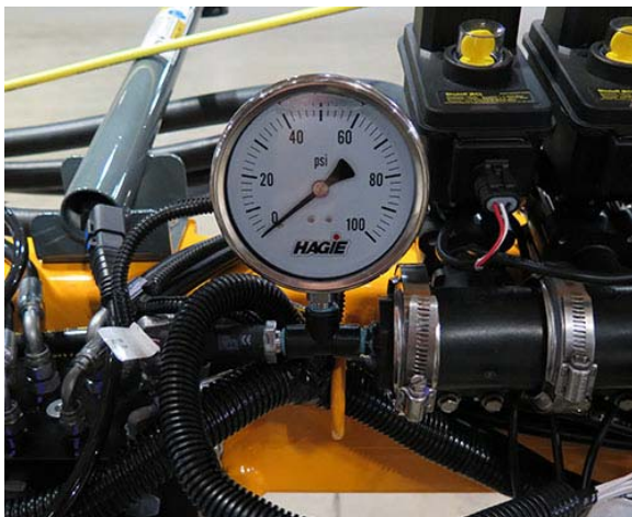
Pressure Gauge (Mounted on boom) -Typical View
