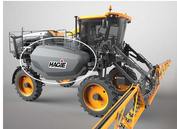
Solution Tank -Typical View
