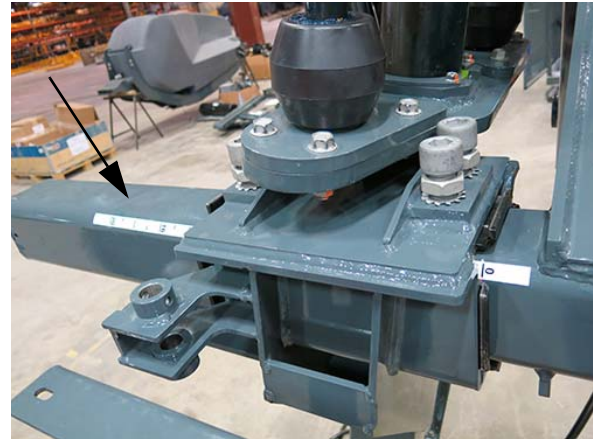
Tread Adjust Slide Path (Located on each leg) -Typical View
