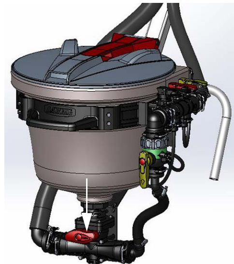
Eductor Tank Valve (Located near the bottom of the eductor tank) -Typical View
