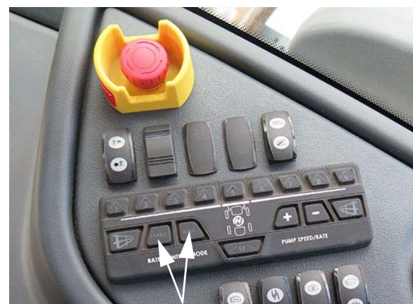
Rate Control Switches (Located on the side console) -Typical View
