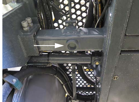
Lifting Point Containment Ring (Located on the frame near each leg) -Typical View
