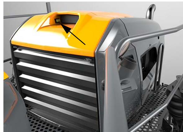
Hood Actuator Switch (Located near front of hood above the radiator screen) -Typical View
