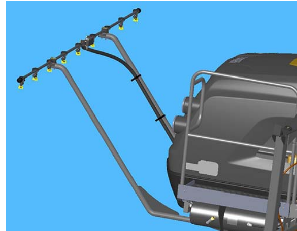
Rear Spray Boom Installation -Typical View
