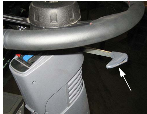
Steering Wheel Telescope Adjust Handle (Located on the right-hand side of steering column) -Typical View
