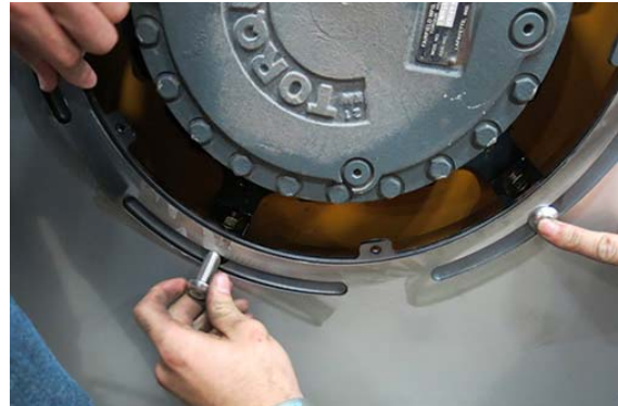
Wheel Cover Mounting Bolt Installation -Typical View
