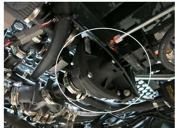
Solution Pump (Located beneath center of machine) -Typical View
