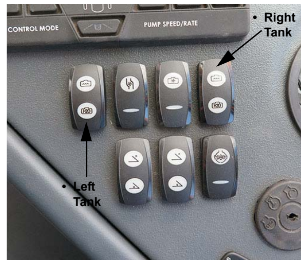
Tank Valve Selector Switches - Left/Right (Located on the side console) -Typical View
