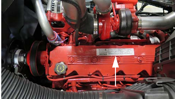
Engine Identification Plate -Typical View
