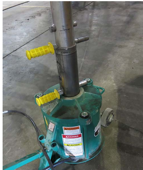
Lock Pin Installation -Typical View
