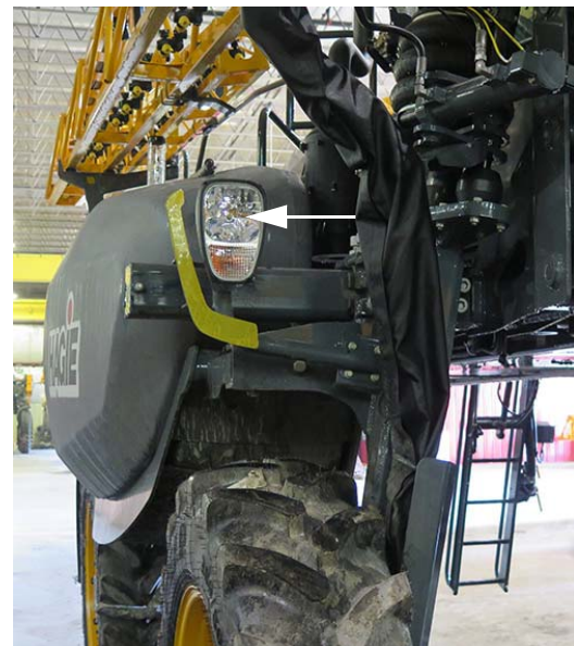
Highway Running Lights (2) -Typical View
