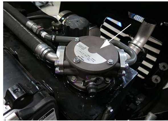
Return Filter Housing (Located on top of hydraulic oil reservoir - open hood to access) -Typical View
