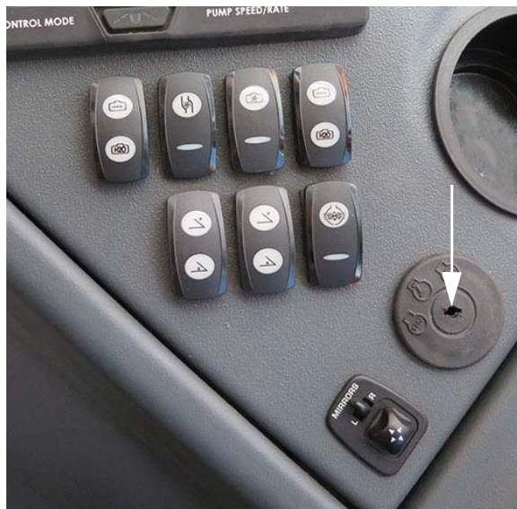
Ignition Switch (Located on the side console) -Typical View
