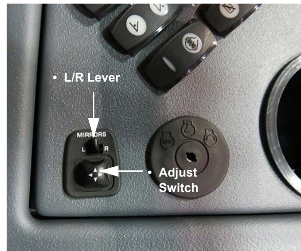
Power Mirror Switch (Located on the side console) -Typical View
