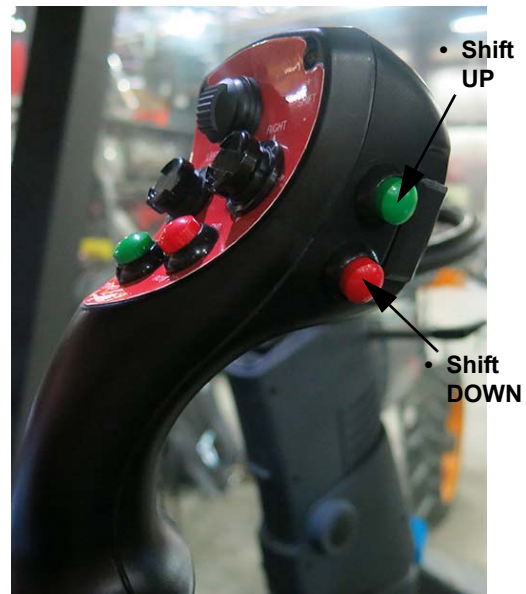
Shift Up/Down Switches (Located on the side of the Hydrostatic Drive Control Handle) -Typical View
