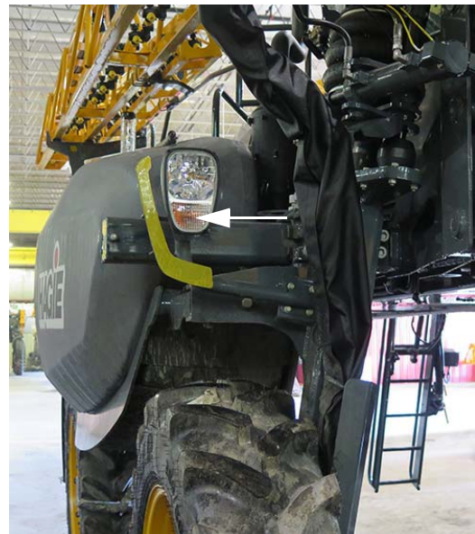
Front Hazard/Warning Light Flashers (2) -Typical View
