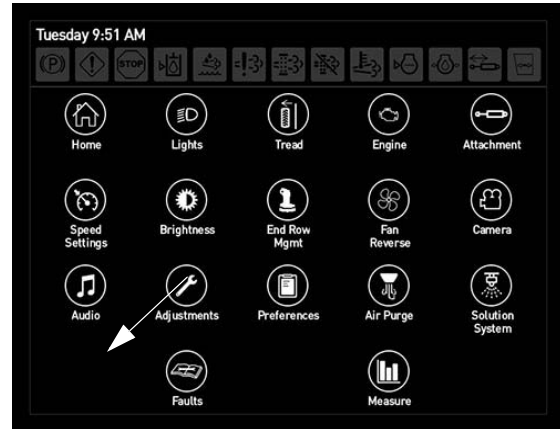
Faults Button (Located on the Main Menu Page)
