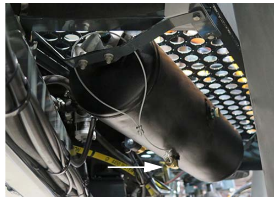
Tank Drain Valve (Air Purge) - if equipped (Located beneath platform near center right-hand side of machine) * Pull DOWN to open -Typical View
