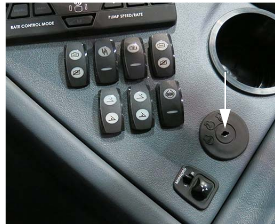
Ignition Switch (Located on the side console) -Typical View
