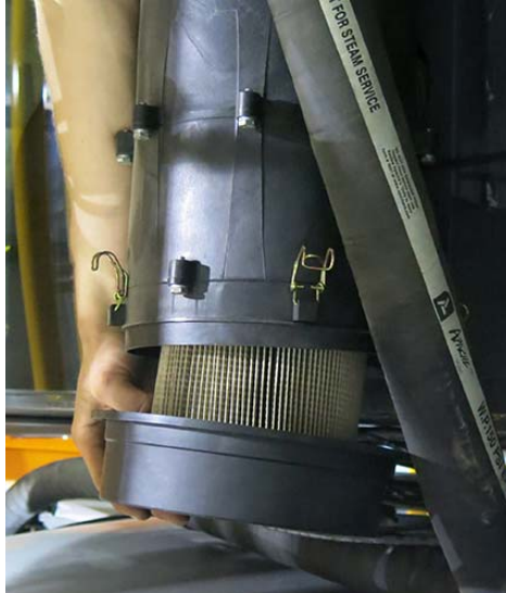
Filter Removal -Typical View
