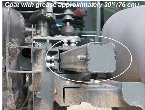
Tread Adjust Bearing Slide Path (4) (Located on each leg) -Typical View
