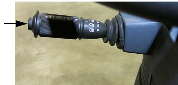
Horn Button (Located on the end of the turn signal lever) -Typical View
