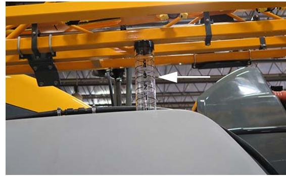
Solution Tank Sight Gauge (2) (Located on top of each solution tank) -Typical View
