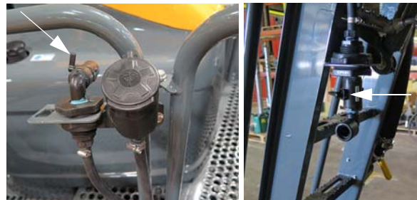
Hand Wash Valve (Left-Hand Platform Handrail)
