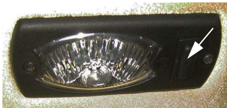
Interior Work Light Switch -Typical View
