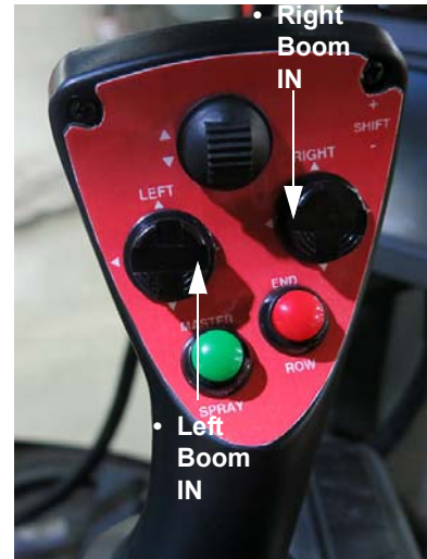
Left and Right-Hand Boom Switches (Located on the Hydrostatic Drive Control Handle) -Typical View
