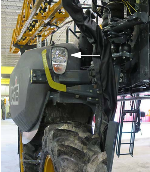
Highway Running Lights (2) -Typical View
