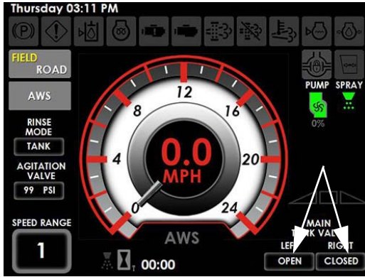
Main Tank Valve Status Indicators (Located on the Machine Display Home Page - Field Mode)
