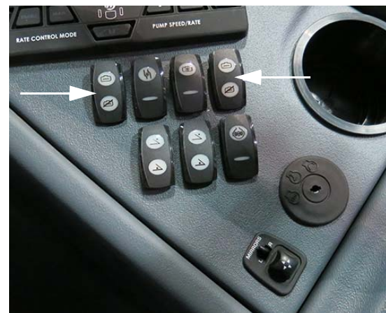
Main Tank Valve Switches (Located on the side console) -Typical View
