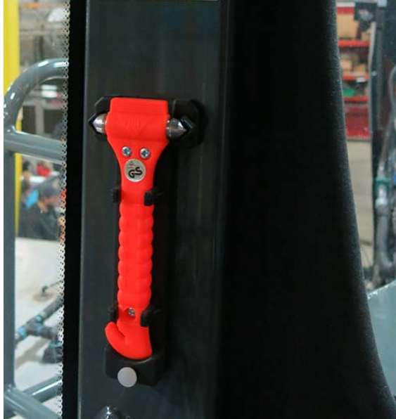
Emergency Exit Tool (Located along rear right-hand side of cab) -Typical View
