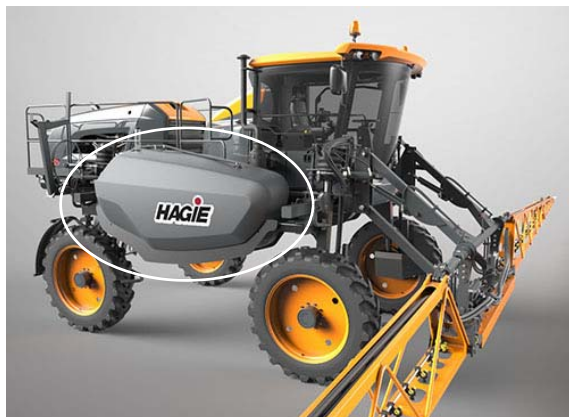
Solution Tank -Typical View
