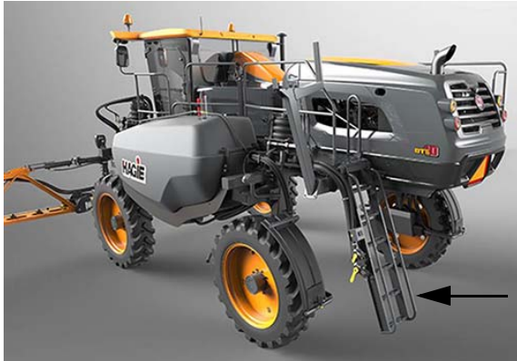
Ladder -Typical View * Lowered position shown
