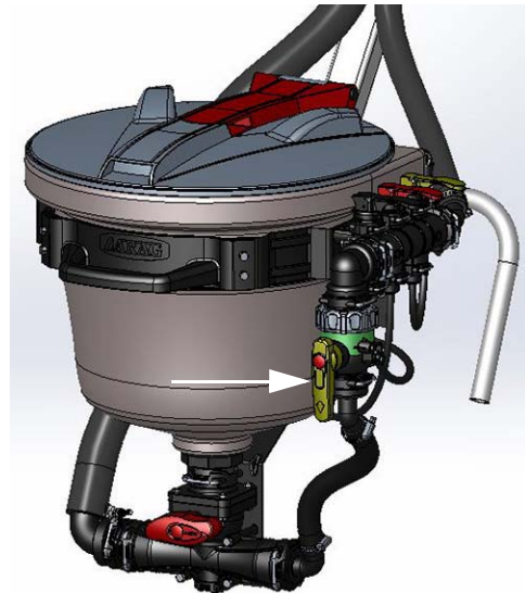
Venturi Valve (Located on the side of eductor tank) -Typical View
