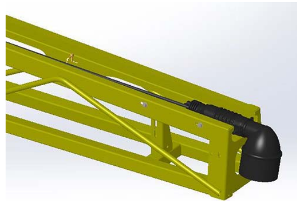
Foam Drop (2) -Typical View
