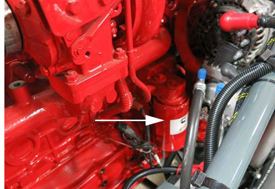
Engine Oil Filter (Located on right-hand side of engine through access opening) -Typical View
