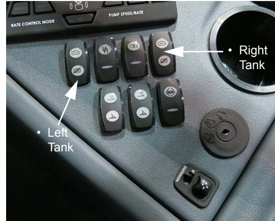
Main Tank Valve Switches - Left/Right (Located on the side console) -Typical View
