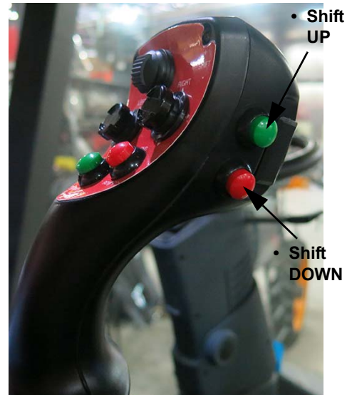
Shift Up/Down Switches (Located on the side of the Hydrostatic Drive Control Handle) -Typical View
