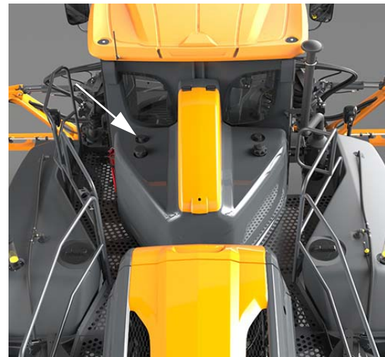
Foam Marker Reservoir Fill (Located on the front left-hand side of fuel-rinse module - “FRM”) -Typical View
