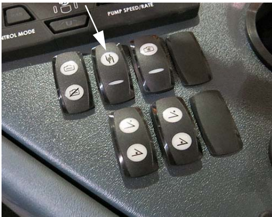
Solution Pump Switch (Located on the side console) -Typical View
