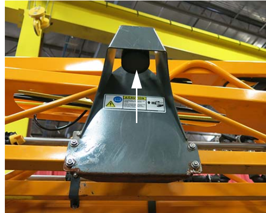
NORAC Sensor Foam Pad (Located on the bottom of each sensor) -Typical View
