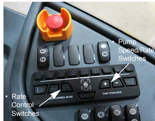
Rate Control and Pump Speed/Rate Switches (Located on the side console) -Typical View
