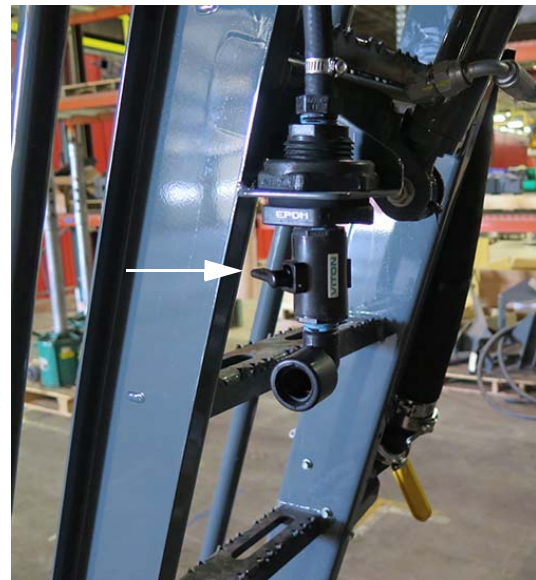
Hand Wash Valve (Ladder) -Typical View
