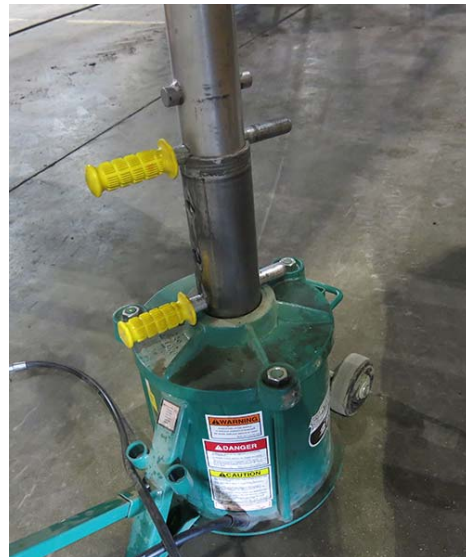
Lock Pin Installation -Typical View
