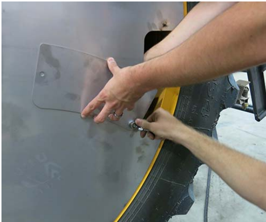
Valve Stem Access Panel -Typical View
