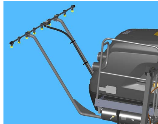
Rear Spray Boom Installation -Typical View
