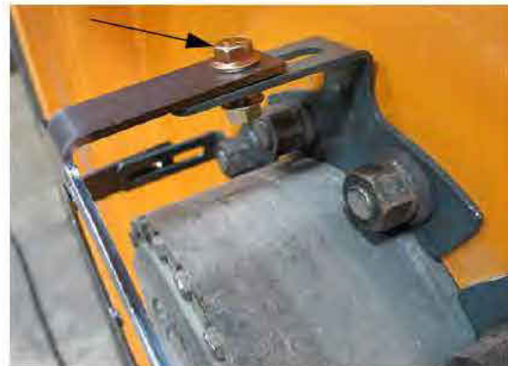
Hub Cap Adapter Bolt Installation -Typical View
