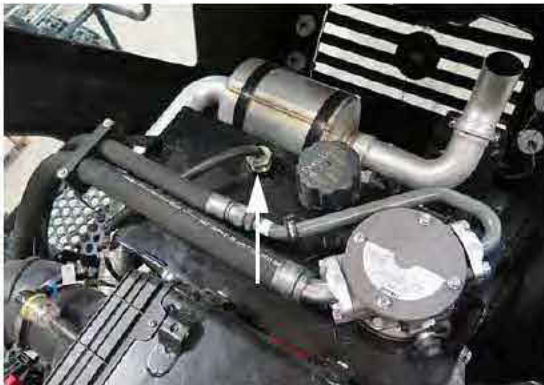
Level/Temp Sensor (Located on top of hydraulic oil reservoir) -Typical View
