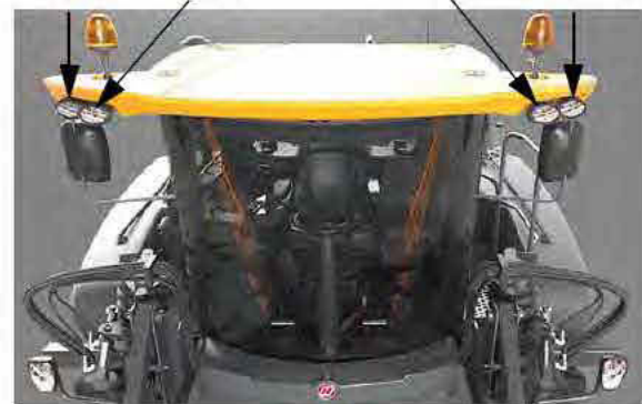
Field Lights (Located on the front of cab) -Typical View
