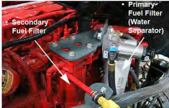
Primary and Secondary Fuel Filters (Located on left-hand side of engine through access opening) -Typical View
