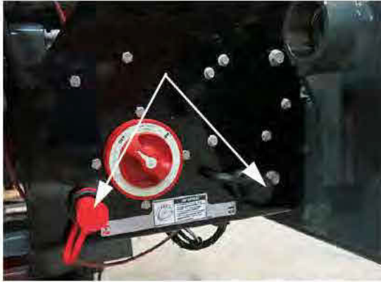
Auxiliary Battery Charging Posts (Located on the rear mainframe) -Typical View
