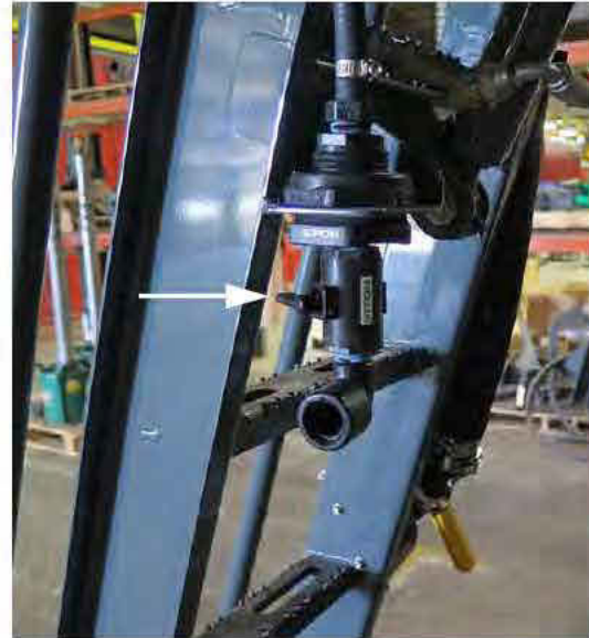
Hand Wash Valve (Ladder) -Typical View
