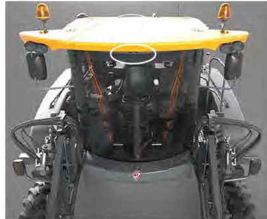
Windshield Washer Fluid Spray Nozzle (Located near top of exterior cab) -Typical View
