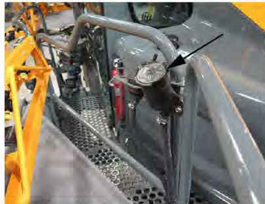
Hand Wash Fill Port (Located on the left-hand platform handrail) -Typical View
