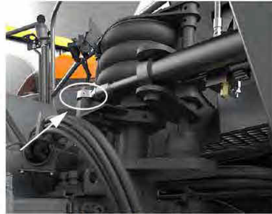
Tie Rod Ball Grease Zerk (Located on the front legs*) -Typical View
