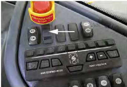
Night Spray Switch (Located on the side console) -Typical View
