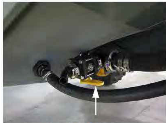
Solution Tank Drain Valve (Located beneath each solution tank on underside of machine) -Typical View
