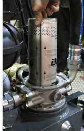
Return Filter (Located inside filter housing on left-hand side of machine) -Typical View
