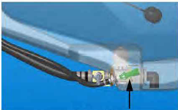
Jet Agitator (Located in sump on each solution tank) -Typical View
