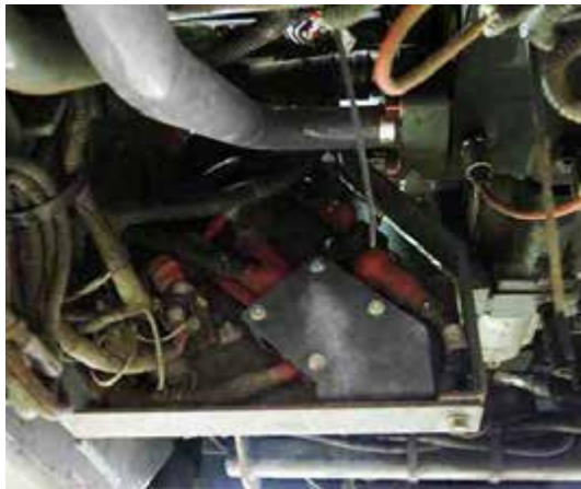
Tier 4 Final Engine Fuse/Relay Block (Located beneath batteries on the rear right-hand side of machine) -Typical View
