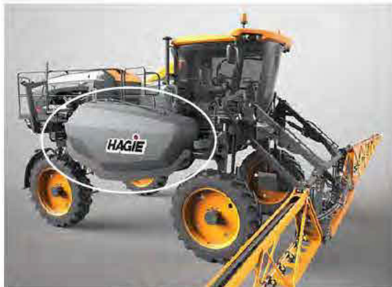
Solution Tank -Typical View
