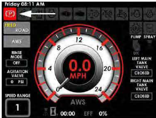
Parking Brake Indicator (Located on the top left-hand side of each Machine Display page)
