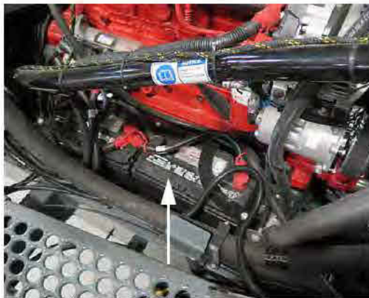
Batteries (Located on the rear right-hand side of machine) -Typical View
