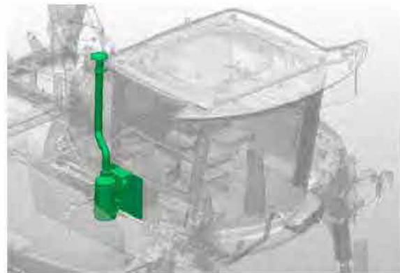
Cab Filtration System (Located on the right-hand side of the exterior cab) -Typical View
