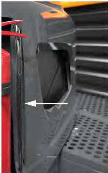
Rinse Tank Sight Gauge (Located on the side of rinse tank) -Typical View
