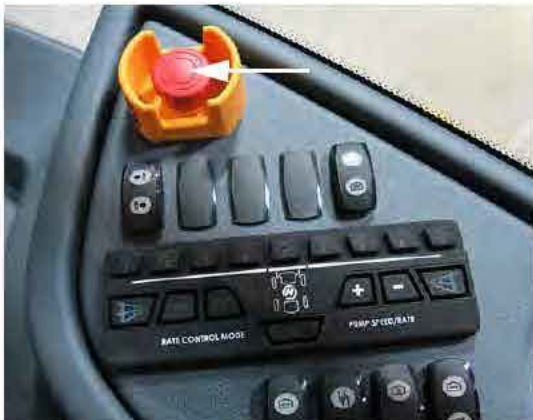
E-Stop Switch (Located on the side console) -Typical View
