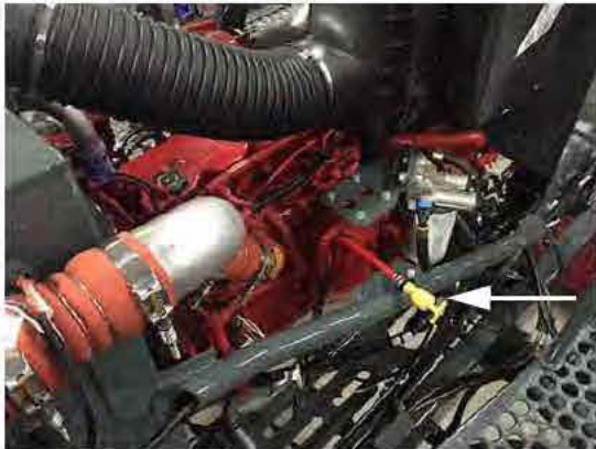
Engine Oil Dipstick (Located on left-hand side of engine through service access opening) -Typical View
