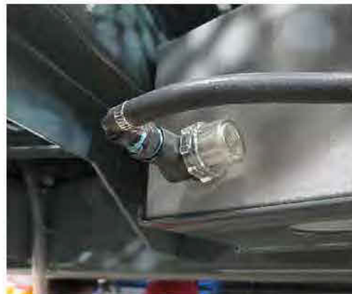
Hand Wash Strainer (Located near the bottom of hand wash tank) -Typical View
