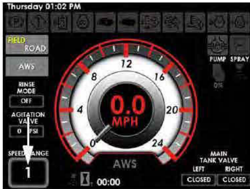
Speed Range (Located on the Machine Display Home Page - Road and Field Mode)
