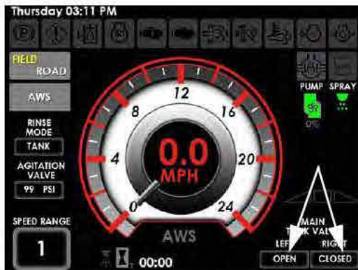
Main Tank Valve Status Indicators (Located on the Machine Display Home Page - Field Mode)
