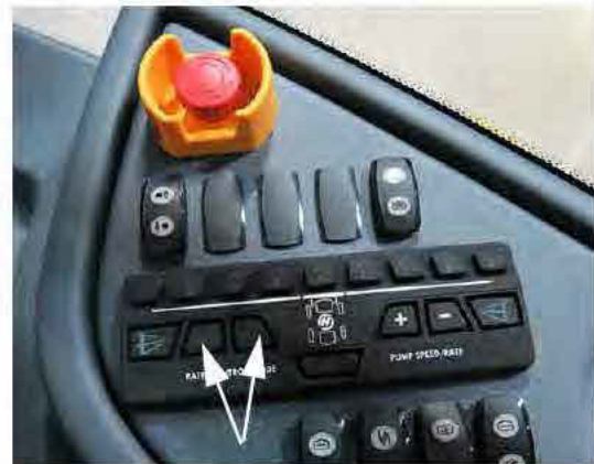
Rate Control Switches (Located on the side console) -Typical View
