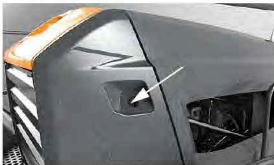
DEF Fill Cap (Located on left-hand side of hood) -Typical View
