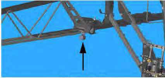
Work Lights (Located on the underside of each boom wing) -Typical View
