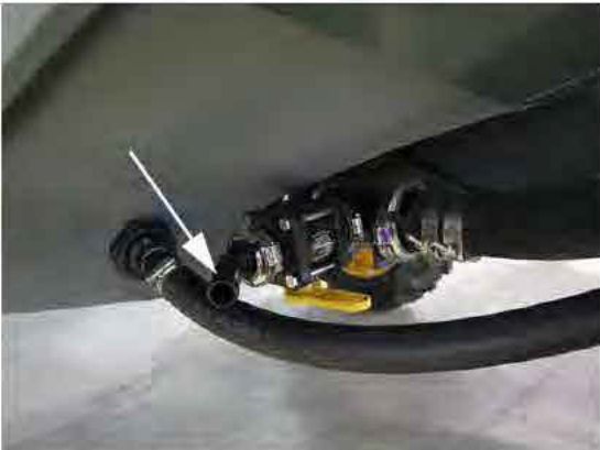
Solution Tank Discharge Outlet (Located beneath each solution tank on underside of machine) -Typical View
