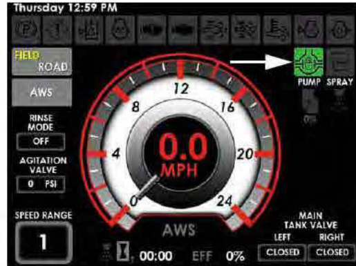
Traction Valve Indicator (Located on the Machine Display Home Page - Road and Field Mode) -Typical View
