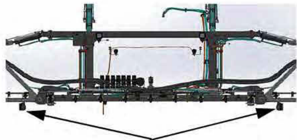
Night Spray Lights (2) (Located on each side of the main boom fold section) -Typical View
