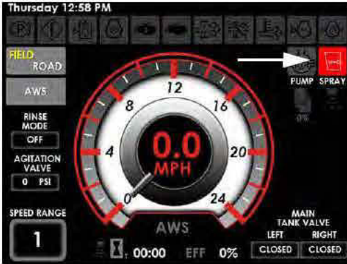
Insufficient Cab Air Pressure Indicator (Located on the Machine Display Home Page - Road or Field Mode)
