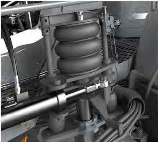
Air Bag (Located on each leg) -Typical View
