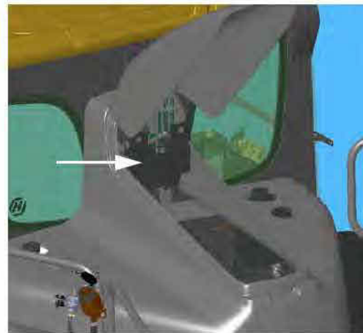
Foam Marker Control Panel (Located inside the FRM compartment - lift lid to access) -Typical View
