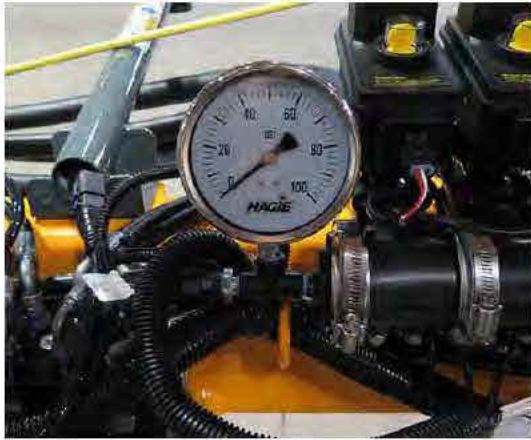
Pressure Gauge (Mounted on boom) -Typical View
