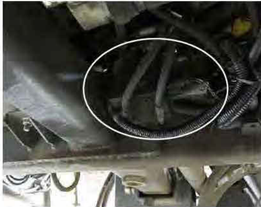
Valve Manifold (Located on the underside of machine) -Typical View
