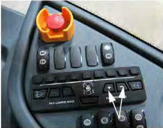
Pump Speed/Rate Switches (Located on the side console) -Typical View
