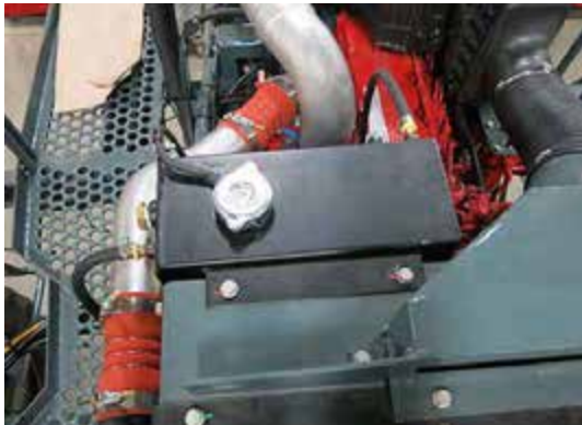
Radiator (Located near the rear of machine - open hood to access) -Typical View
