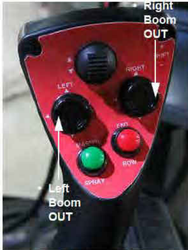
Left and Right-Hand Boom Switches (Located on the Hydrostatic Drive Control Handle) -Typical View
