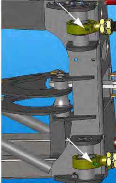
Outer Fold Joint Rod End Grease Zerks -Typical View
