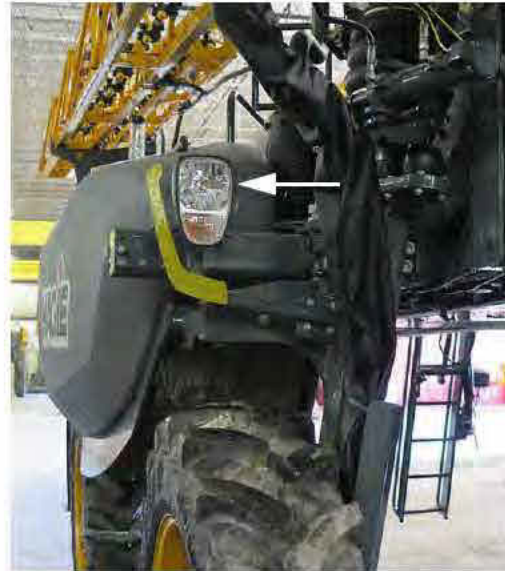
Highway Running Lights (2) -Typical View
