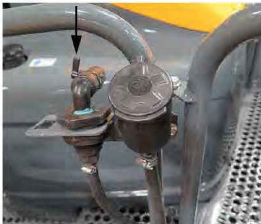
Hand Wash Valve (Left-Hand Platform Handrail) -Typical View
