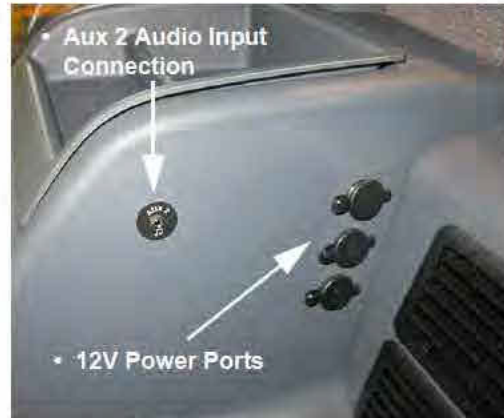
12V Power Ports and Aux 2 Audio Input Connection (Located on the inward side console panel) -Typical View
