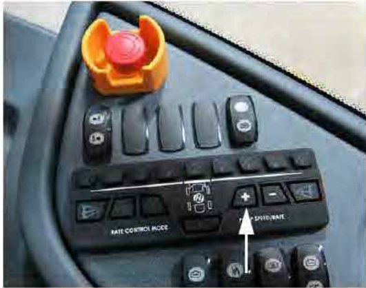
“+” Pump Speed/Rate Switch (Located on the side console) -Typical View
