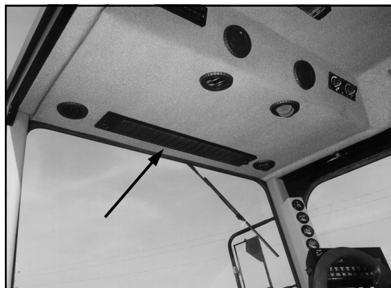
CAB FILTER LOCATION FIG 8.27
