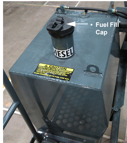
Engine Fuel Fill (Located on top of fuel tank on each side of machine) -Typical View
