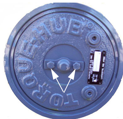
Cap Bolts -Typical View
