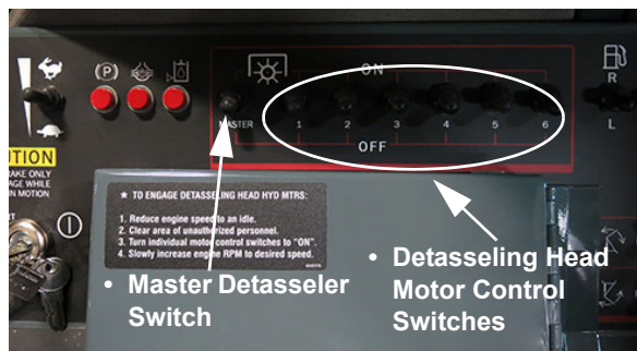
Master Detasseler and Detasseling Head Motor Control Switches (Located on the side console) -Typical View
