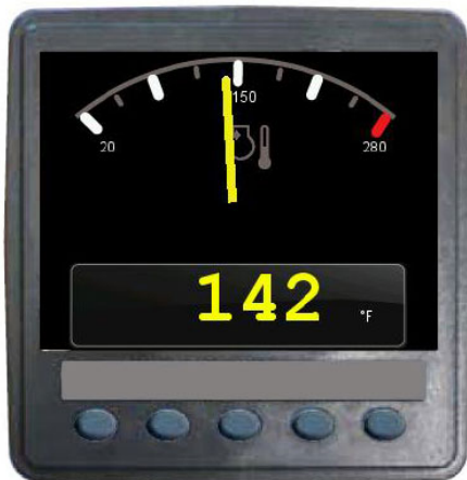
Single Analog Gauge Screen -Typical View
