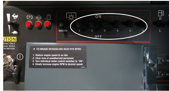
Detasseling Head Motor Control Switches (Located on the side console) -Typical View
