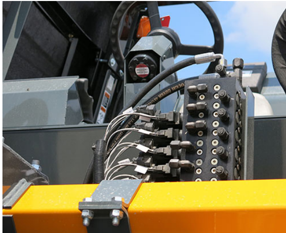
Electro-Hydraulic Valves (Located on the front of tool bar) -Typical View
