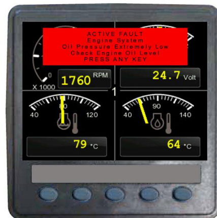
Active Fault Warning -Typical View
