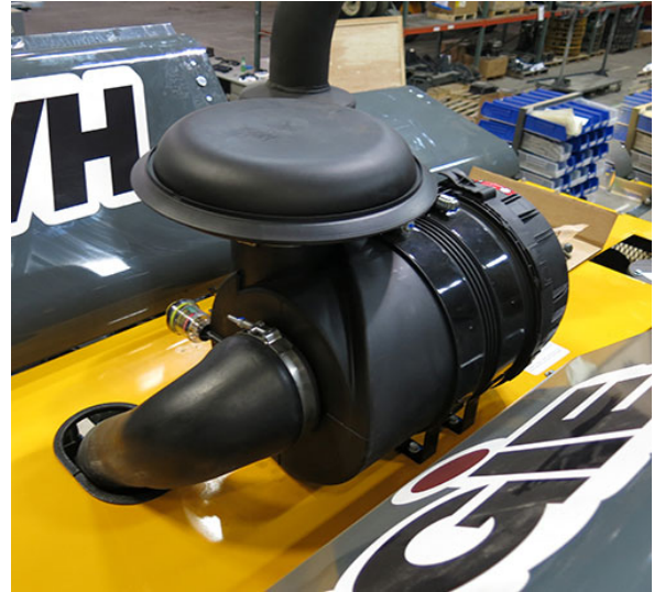
Engine Air Intake Filter (Located near rear of machine - remove air cleaner end cap to access) -Typical View
