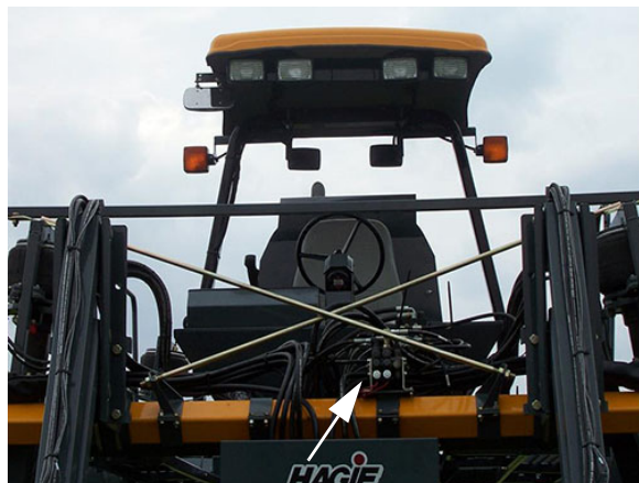
Hydraulic Fold Valve (Located on center tool bar) -Typical View
