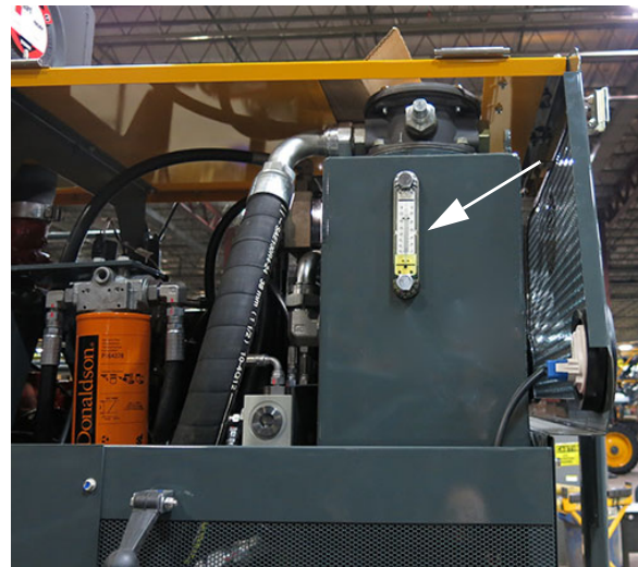
Hydraulic Oil Reservoir Sight Gauge (Located on front of hydraulic oil reservoir) -Typical View
