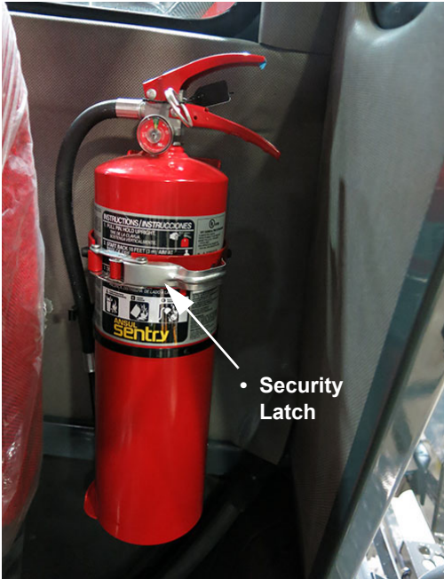
Fire Extinguisher (Located along side of operator's seat) -Typical View
