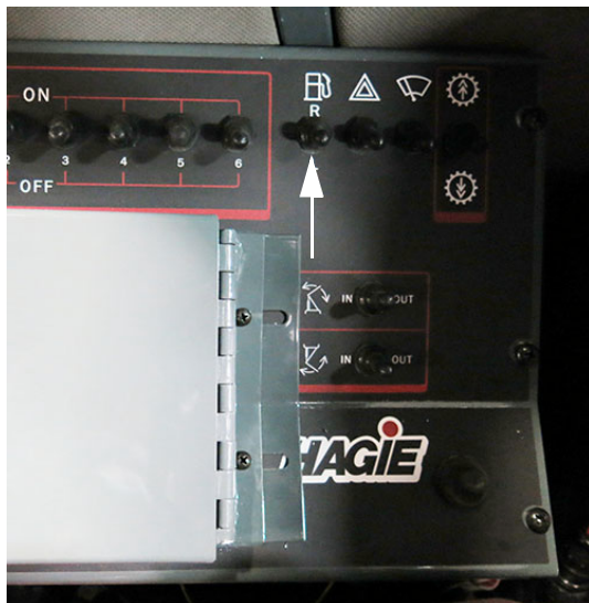
Fuel Tank Selector Switch (Located on the side console) -Typical View
