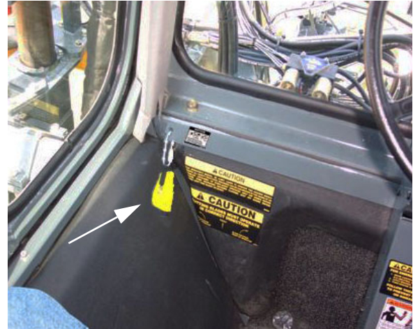
Emergency Exit Tool (Located near the left-hand side of cab) -Typical View
