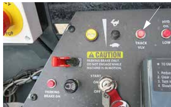
Traction Valve Indicator (Located on the side console) -Typical View
