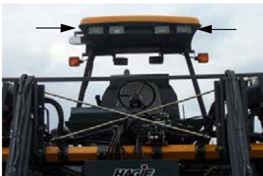
Work Lights (Located on the front and rear of operator's station) -Typical View
