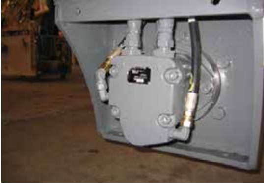
Right Rear Wheel Motor (w/Sensor) -Typical View
