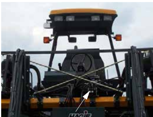
Hydraulic Fold Valve (Located on center tool bar) -Typical View
