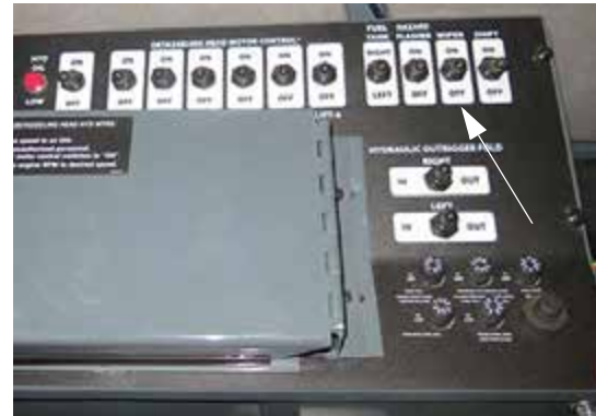
Windshield Wiper Switch (Located on the side console) -Typical View
