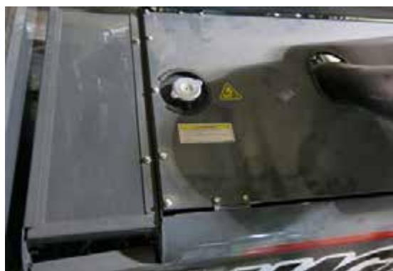
Radiator Cap (Located behind the operator’s station) -Typical View
