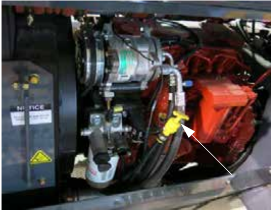
Engine Oil Dipstick (Located on the left-hand side of engine - open hood to access) -Typical View
