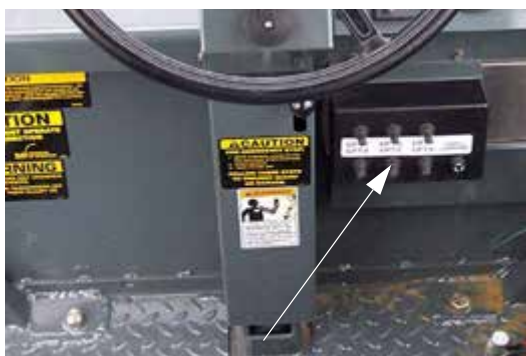
Depth Command Switches (Located near the front of operator's station) -Typical View
