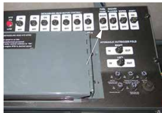
Fuel Tank Selector Switch (Located on the side console) -Typical View
