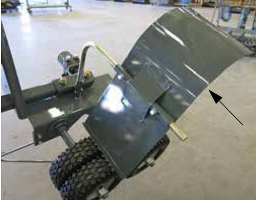
Deflector Shield -Typical View
