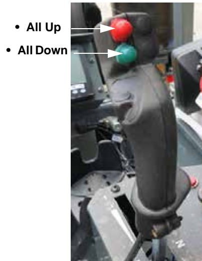
All Up/Down Switches (Located on the Hydrostatic Drive Control Handle) -Typical View
