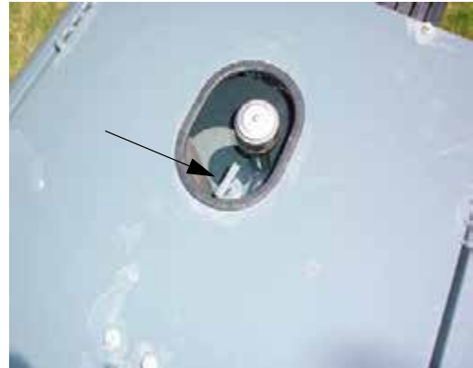
Hydraulic Oil Dipstick (Located on top of the hydraulic oil reservoir) -Typical View
