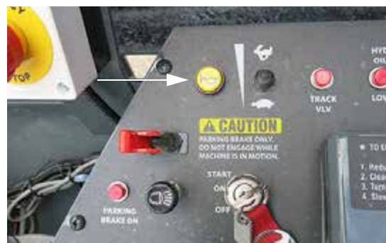
Horn Button (Located on the side console) -Typical View
