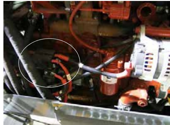
Wire Harness Circuit Breaker and Fuses (Located on the left-hand side of engine) -Typical View
