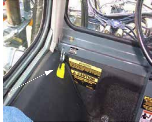
Emergency Exit Tool (Located near the left-hand side of cab) -Typical View
