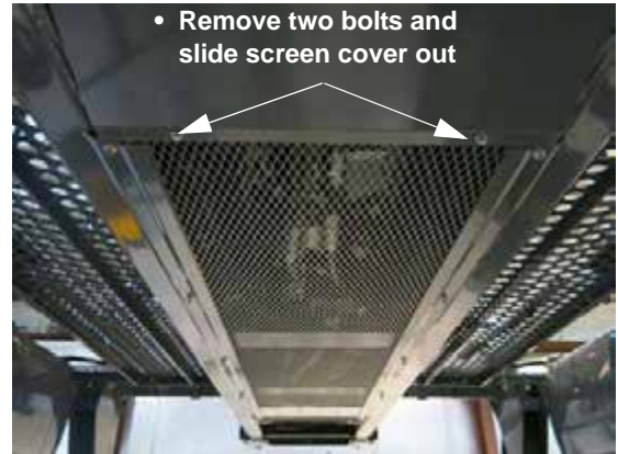
Screen Cover (Located on underside of machine) -Typical View
