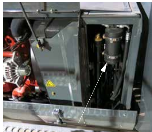
A/C System Receiver/Dryer (Located behind cab near the radiator - remove radiator screens to access) -Typical View
