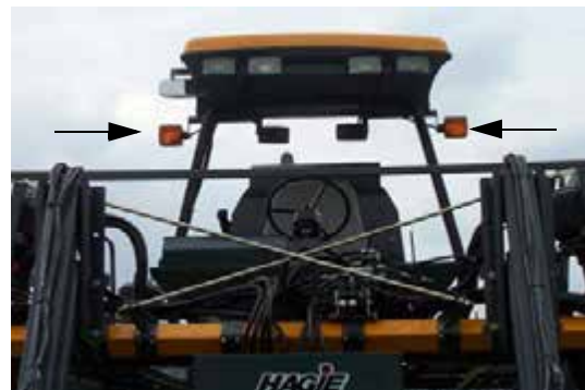
Highway Running Lights (Located on the front and rear of operator's station) -Typical View
