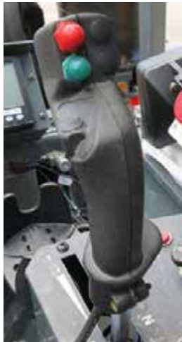
Hydrostatic Drive Control Handle (Located on the side console) -Typical View
