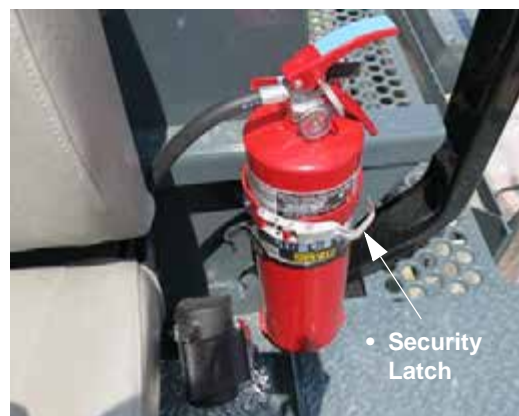
Fire Extinguisher (Located along side of operator's seat) -Typical View
