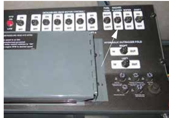
Hazard Flasher Switch (Located on the side console) -Typical View
