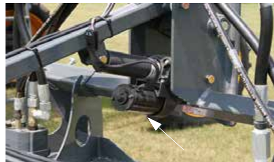
Depth Command Actuator (Located on the tool bar lift head tube) -Typical View
