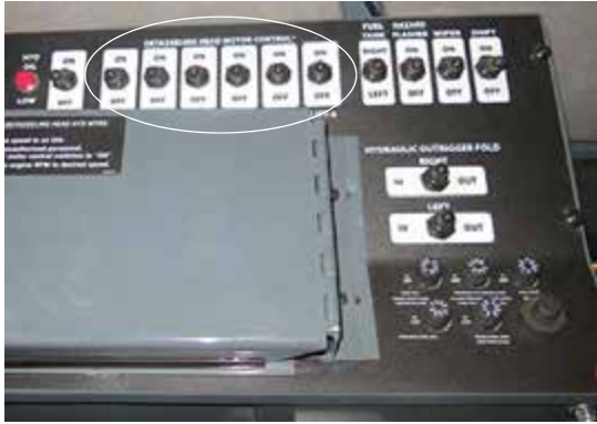
Detasseling Head Motor Control Switches (Located on the side console) -Typical View
