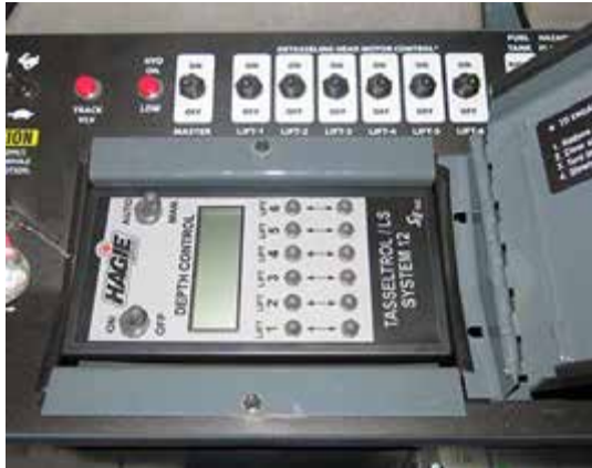
Tasselrol/LS System 12 Control Panel (Located on the side console - lift cover to access) -Typical View
