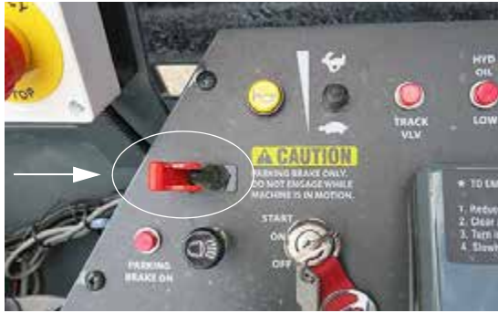
Parking Brake Switch (Located on the side console) -Typical View
