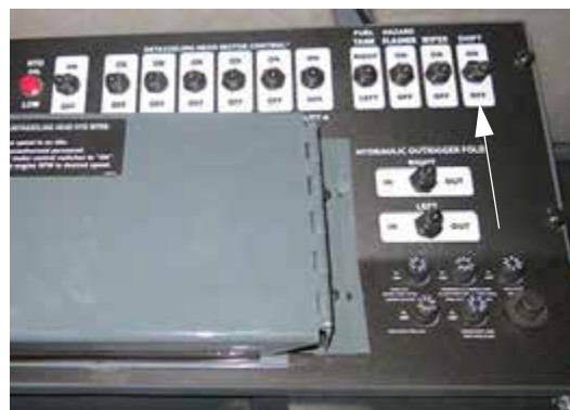
Shift Switch (Located on the side console) -Typical View
