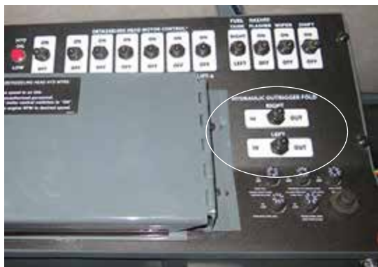
Hydraulic Outrigger Fold Switches (Located on the side console) -Typical View
