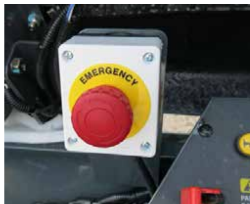
E-Stop Switch (Located near the side console) -Typical View
