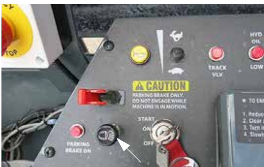
Work Lights Switch (Located on the side console) -Typical View
