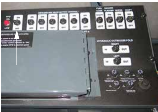
Master Detasseler Switch (Located on the side console) -Typical View
