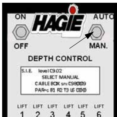
Auto/Manual Switch (Located on the Tasseltrrol Control Panel)
