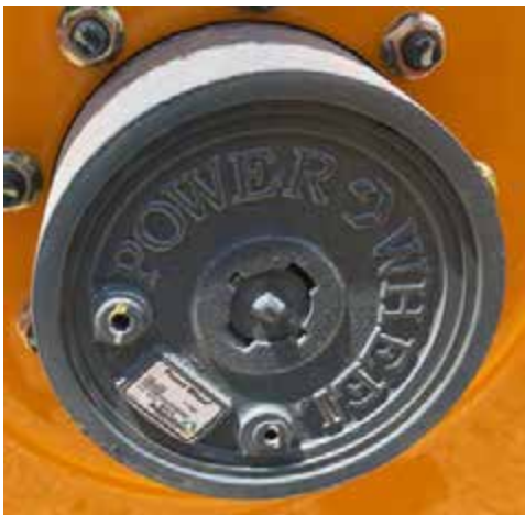
Planetary Wheel Hubs (w/Brakes) -Typical View
