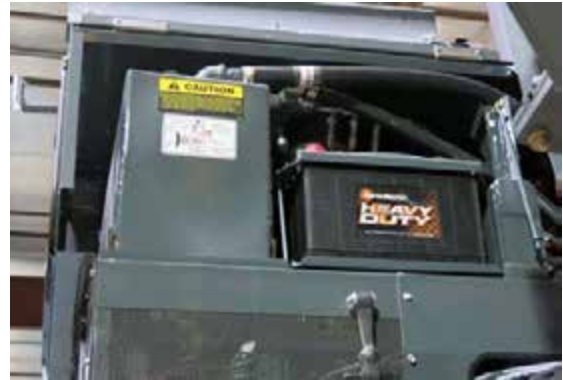
Battery Access (Located near rear right-hand side of machine - open hood to access) -Typical View
